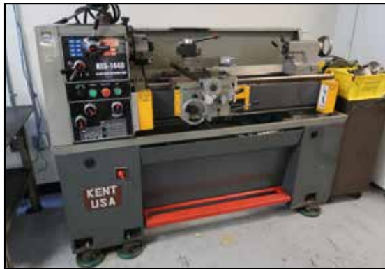
Kent KLS-1440 14" x 40" Geared Head - Gap Bed Lathe w/ 45-1800 RPM, Inch/mm Threading, Tailstock, Steady and Follow Rests, Phase II Tool Post, 5C Collet Closer, 8" 4-Jaw Chuck, 6.5" 3-Jaw Chuc
