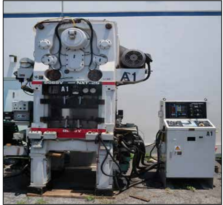
2000 Yamada Dobby NXT-25I 25-Ton High Rigidity High Speed CNC Hydraulic Punch Press s/n 0140 w/ Yamada Digital Controls, Double Link Motion, 15-30mm Adjustable Stroke, 180-1100 Strokes/Min, 50mm Slide Adj, 640mm x 450mm Bolster Area, 640mm x 320mm Slide Area, 500mm x 80mm Bed Opening, Yamada 4" Servo Feeder.
