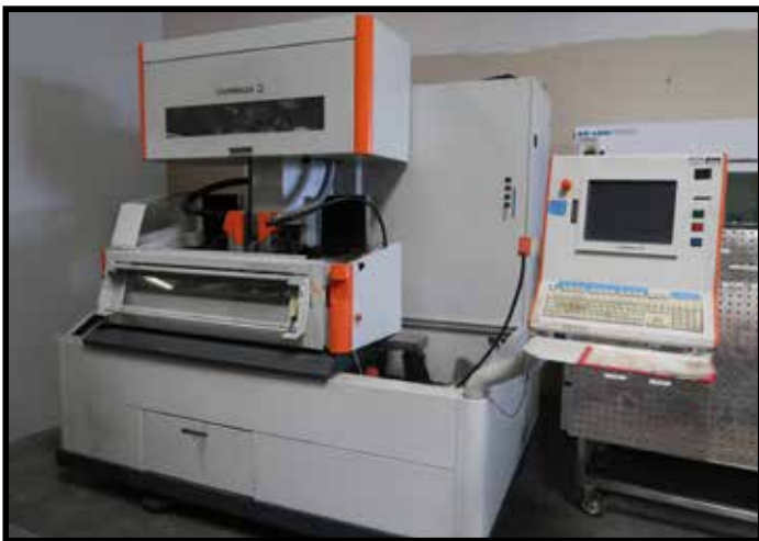
Charmilles Robofil 2050TW CNC Wire EDM Machine w/ Dielectric Filtration System, 16" x 23 1/2" Table Area, 10" x 14" Work Area.
