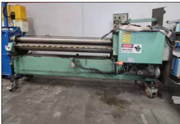
M Montgomery 9612-H 8' Power Roll s/n 200001 w/ 6" Top Roll, 7" Bottom Rolls.
