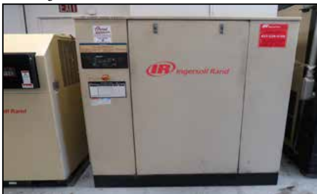
Ingersoll Rand SSR-EP100 100Hp Rotary Air Compressor s/n CK9762U11280 w/Ingersoll Rand Digital Controls, 434 CFM @ 125 PSIG.
