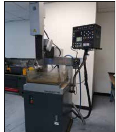
2004 Elenix "EdmDrill C T300" CNC Hole Popper EDM Machine s/n 84241 w/ Elenix CT300 Controls, Hand Controller, 12" x 12" Table.
