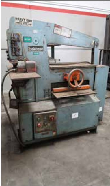
Scotchman 65 Ton Hydraulic Iron Worker w/ Punch Head, 24" Flat Shear.
