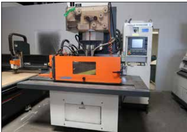
Charmilles Robofil 4020ST CNC Wire EDM Machine w/ Dielectric Filtration System.
