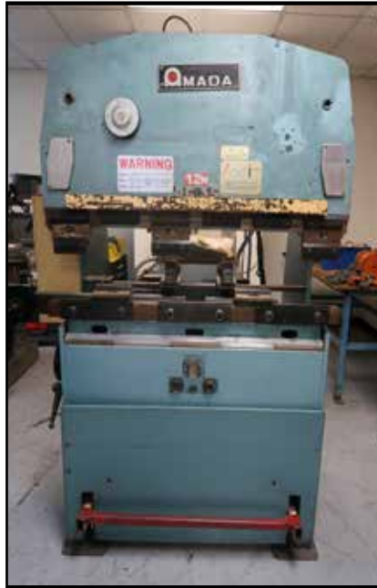
Amada RG-35S 35 Ton x 48" Press Brake s/n 351642 w/ Manual Back Gaging, 48" Bed Length, 40" Between Uprights, 7.88" Throat, 3.94" Stroke, 13.79" Open Height.
