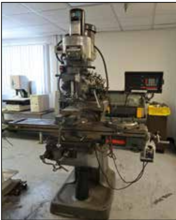
Bridgeport Vertical Mill w/ Newall DP7 3-Axis Programmable DRO, 60-4200 Dial Change PM, Kurt Power Draw-Bar, Chrome Ways, Power Feed, 9" x 48" Table.
