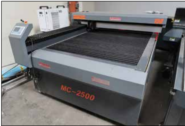
2022 Mintech MC-2500 150 Watt CO2 High Performance Laser Cutting / Engraving Machine s/n 131208220 w/ PLC Controls, 49" x 98" Cap, Cooling Unit, Exhaust Blower.
