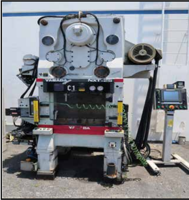
2006 Yamada Dobby NXT-25I 25-Ton High Rigidity High Speed CNC Hydraulic Punch Press s/n 0354 w/ Up-Graded Yamada CNC Controls, Double Link Motion, 15-30mm Adjustable Stroke, 180-1100 Strokes/Min, 50mm Slide Adj, 640mm x 450mm Bolster Area, 640mm x 320mm Slide Area, 500mm x 80mm Bed Opening, Yamada 4" Servo Feeder, Light Curtain.
