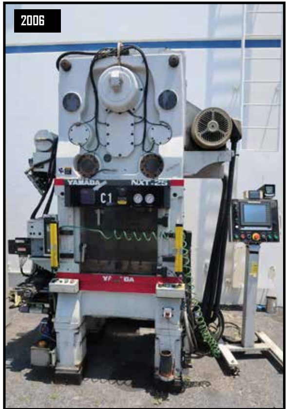
2006 Yamada Dobby NXT-25I 25-Ton High Rigidity High Speed CNC Hydraulic Punch press s/n 0354 w/ Up-Graded Yamada CNC Controls, Double Link Motion, 15-30mm Adjustable Stroke, 180-1100 Strokes/Min, 50mm Slide Adj, 640mm x 450mm Bolster Area, 640mm x 320mm Slide Area, 500mm x 80mm Bed Opening, Yamada 4" Servo Feeder, Light Curtain.
