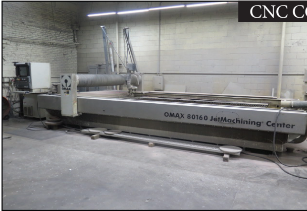
Omax 80160 5-Axis CNC Waterjet Contour Machine s/n E511599 w/ Omax CNC Controls, 6' x 12' Sheet Cap, Tilt-A-Jet 5-Axis Cutting Head, mdl. 4055V 40Hp 55,000 PSI Pump, Koolant Koolers Cooling Unit.
