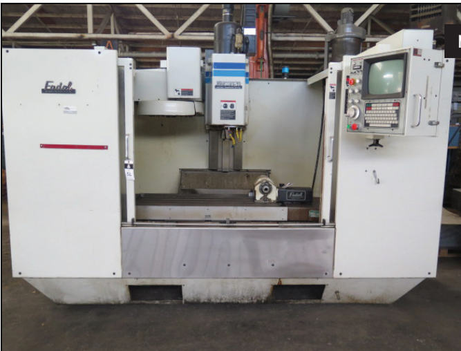
Fadal VMC4020HT 5-Axis Capable CNC VMC w/ CNC88 Controls, 21-Station ATC, CAT-40 Spindle, 7500 RPM
