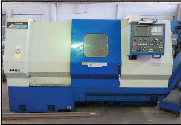
1999 Johnford TC-35 CNC Turning Center w/ Fanuc 18-T Controls, 12-Station Turret, Tailstock, 10" Power Chuck
