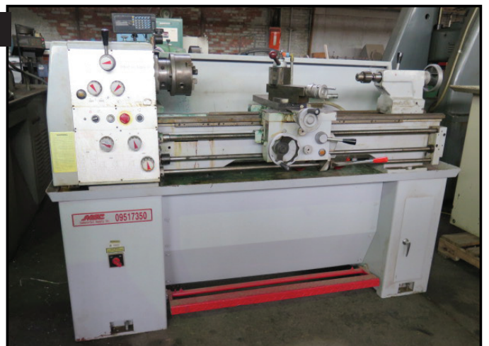
MSC 13" x 36" Geared Head Gap Bed Lathe w/ 105-2000 RPM, 6" Chuck
