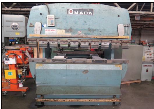
Amada RG-80S 80 Ton x 78" CNC Press Brake w/ Amada Controls and Back Gauging
