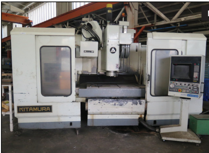
Kitamura Mycenter-6B CNC VMC w/ Fanuc 11M Controls, 30-Station ATC, CAT-50
