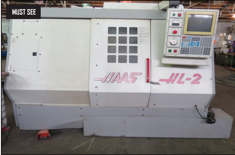
Haas HL-2 CNC Turning Center w/ 10-Station Turret, Tailstock, 8" Power Chuck
