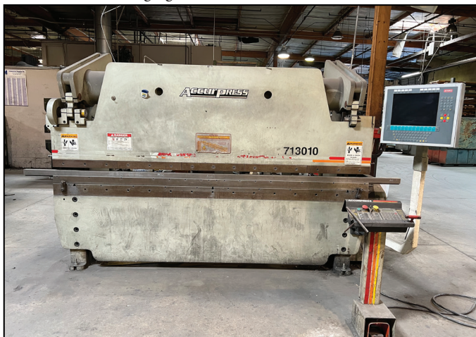
2001 Accurpress 713010 130 Ton x 10' CNC Hydraulic Press Brake s/n 6776 w/ Accurpress Controls and Back Gauging, Accurpress ETS Control, 12 3/4" Throat.
