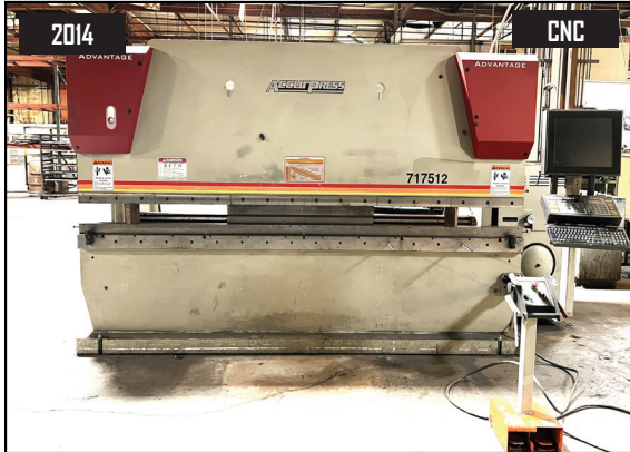
2014 Accurpress Advantage 177512 175 Ton x 12' CNC Hydraulic Press Brake s/n 11867 w/ Accurpress ETS Controls and CNC Back Gauging, 10 3/4" Throat.
