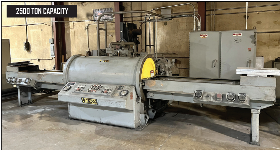
Version 2500R-20-50 2500 Ton Hydraulic Bladder Press s/n 27758 w/ Version Controls, 5000 Max PSI, 20" x 50" Platen Area, 4" Platen Depth.
