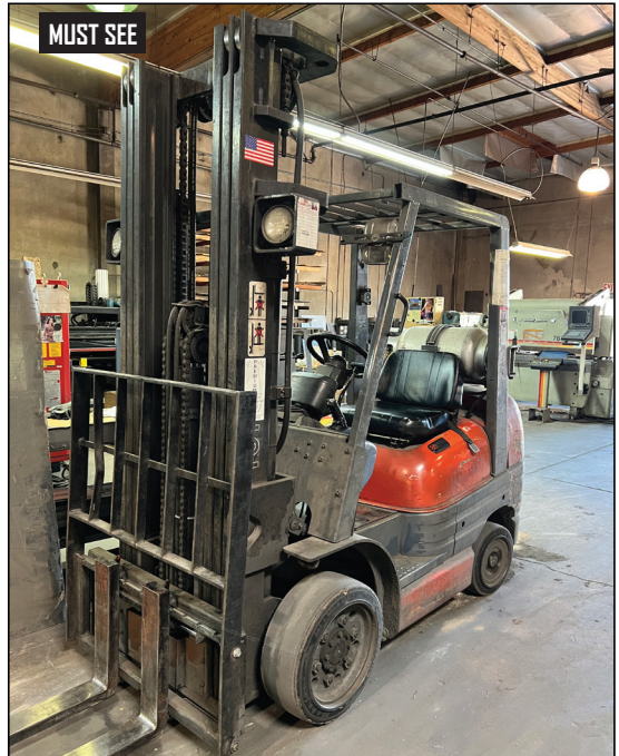
Toyota 42-6FGCU30 5000 Lb Cap LPG Forklift s/n 61406 w/ 3-Stage Mast, 205" LiftHeight, Side Shift, Cushion Tires, 15,375 Hours.
