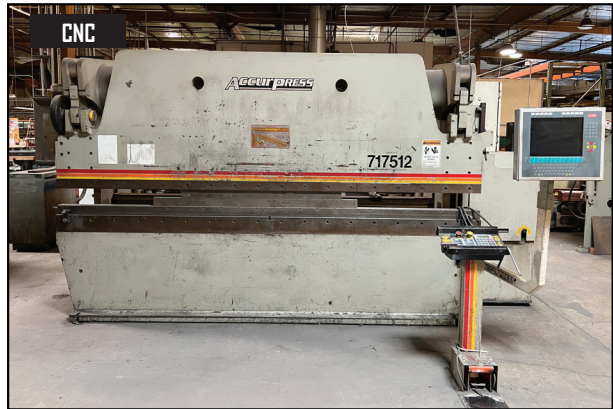
2002 Accurpress 717512 175 Ton x 12' CNC Hydraulic Press Brake s/n 7285 w/ Accurpress Controls and ETS CNC Back Gauging, 10 1/4" Throat.
