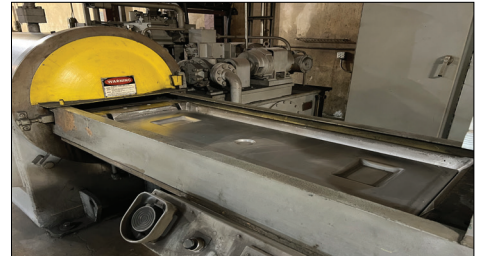
Version 2500R-20-50 2500 Ton Hydraulic Bladder Press s/n 27758 w/ Version Controls, 5000 Max PSI, 20" x 50" Platen Area, 4" Platen Depth.
