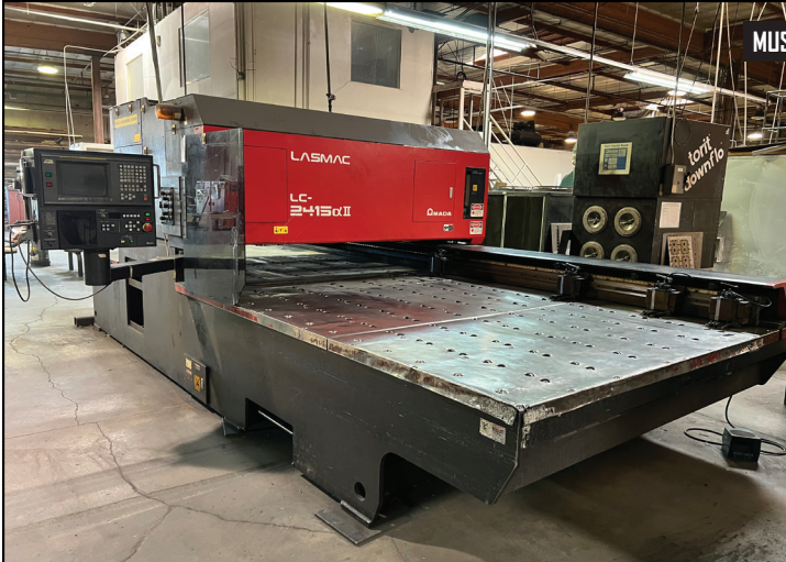
1995 Amada Lasmac LC-2415 cxII 1.5kW CNC Laser Contour Machine s/n 12415052 w/ Fanuc Series 16-L Controls, Fanuc 1500 Watt Laser Source, Torit Downflo Dust Collector, Roller-Top Table.
