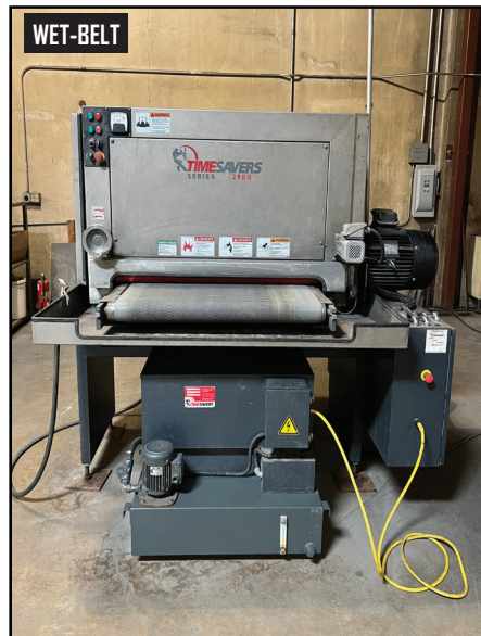
Timesavers 2111-13-0 36" Wet-Belt Grainer s/n SN34194 w/ 36" Belt Feed, Particulate Separation and Filtration System.
