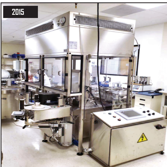
2015 COZZOLI RFC-140 Liquid Filling Line, Rated 12-120ML, Labeling Station to Monobloc, Fill Cycle at 50 PPM, Vibratory Sorting System, Cozzoi UT30-981 Descalber. Automated Bottling Line w/ Controls, Single Station Filling, Labeling Station, Out-Feed Turntable, Conveyor, Enclosure Booth with Ventilation.
