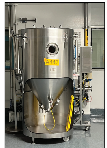
2015 GEA MM-PSR MOBILE MINOR SPRAY DRYER, PLANT SIZE 0.8.
