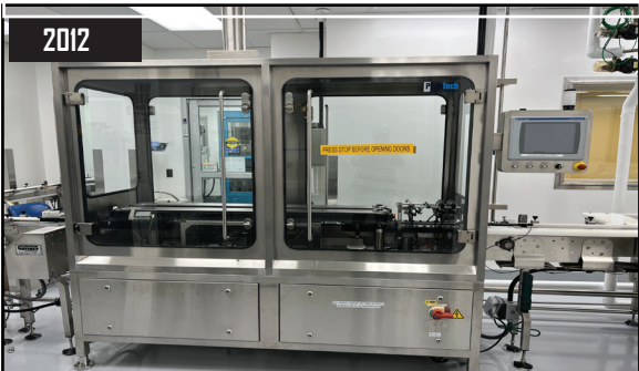
2012 PENN-TECH EVW-200 (SP-HULL) EXTERNAL VIAL WASHER W/ ALLEN BRADLEY PANEL VIEW 1000 CONTROLS.
