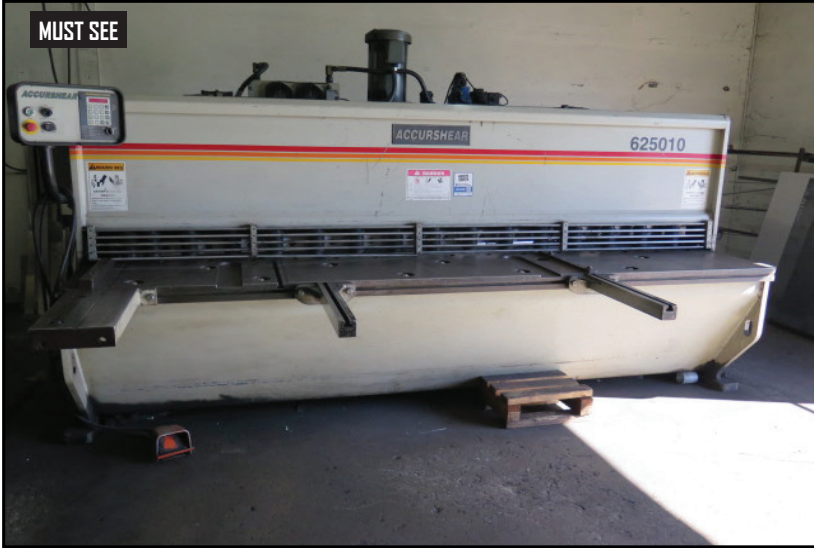
1999 Accurshear 625010 ¼" x 10' Hydraulic Power Shear w/ Accurshear SC2 Back Gauging Controls, 48" Squaring Arm
