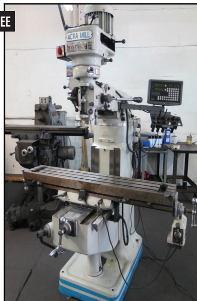
Acra Mill AM2S Vertical Mill w/ Sino SDS6-2V DRO, 3Hp, 80-5440 RPM, 16-Speeds, Chrome Ways, Power Feed
