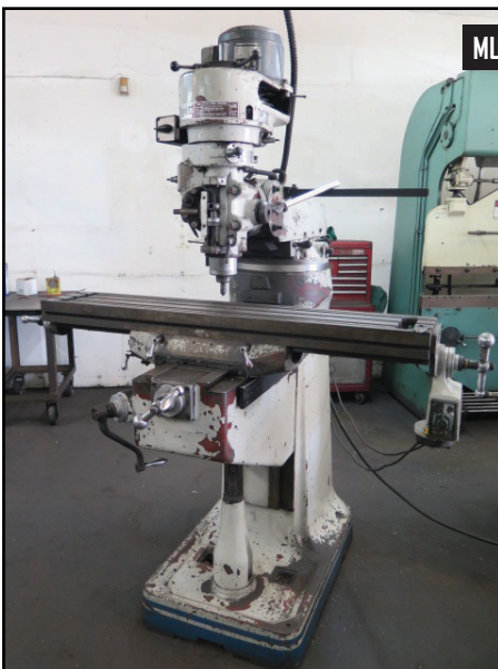
Acra AM-2S Vertical Mill w/ 1Hp, 80-5440 RPM, 16-Speeds, Power Feed
