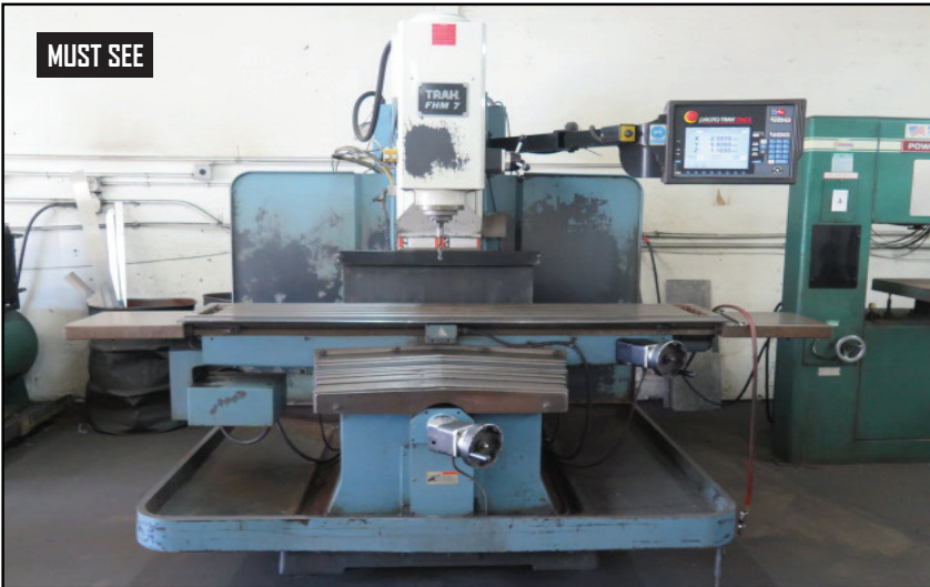
Trak FHM 7 CNC VMC w/ Proto Trak SMX Controls, 200-5000 Controlled RPM, 40-Taper Spindle
