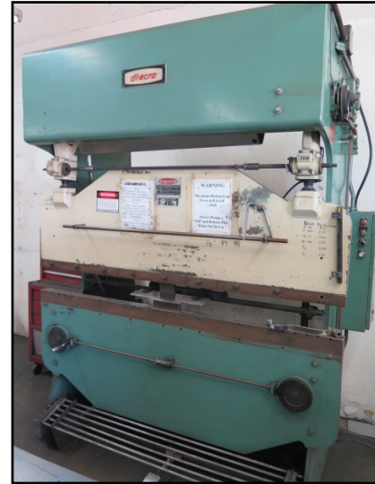
DiAcro 16-72 16GA x 6' Hydra Power Press Brake w/ Dial Back Gauge, 9 1/8" Throat
