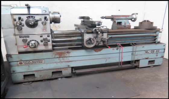
Toga Japan NL-20X60 20" x 60" Gear-Gap Lathe w/Inch/mm Threading, Tailstock, 8" 3-Jaw Chuck
