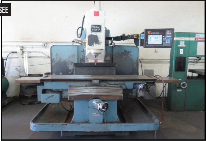
Trak FHM 7 CNC VMC w/ Proto Trak SMX Controls, 200-5000 Controlled RPM, 40-Taper Spindle
