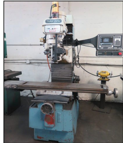
Trak DPM 3-Axis CNC Vertical Mill w/ Proto Trak MX3 Controls, 70-4200 RPM, 40-Taper Spindle, Power Draw-Bar, Chrome Box Ways
