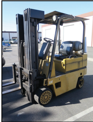
Caterpillar T40D 4000 Lb Cap LPG Forklift w/ 3-Stage Mast, 188" Lift Height, Side Shift
