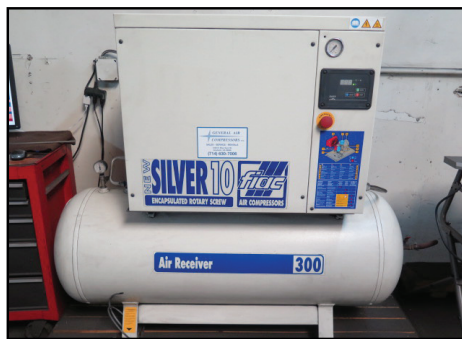
2017 Fiac "New Silver 10/300" Rotary Air Compressor w/ Easy-Air Digital Controls, 10Hp
