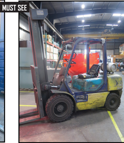
Komatsu 30 6000 lb Cap LPG Forklift w/ 2-Stage Mast, Solid Yard Tires
