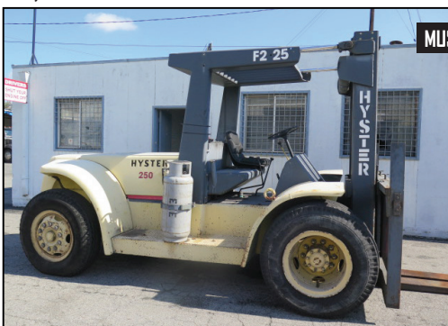
Hyster H250E 25,000 Lb Cap Short Mast LPG Forklift w/ Pneumatic Tires
