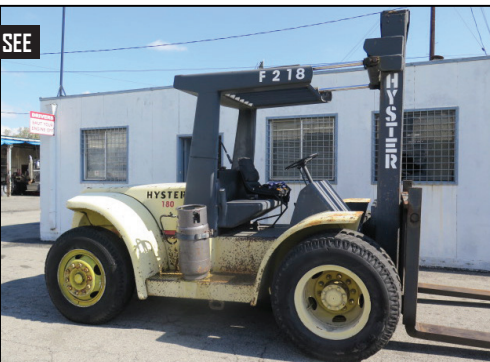
Hyster 180 18,000 Lb Cap LPG Forklift w/ 212" Lift Height, Pneumatic Tires
