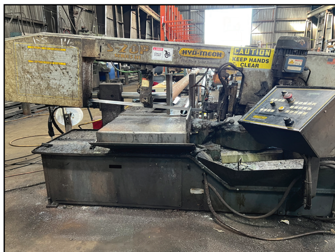
Hyd-Mech S-20P Series III 13" Horizontal Band Saw w/ Hyd-Mech Controls, Hydraulic Clamping, Coolant.
