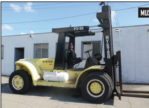
Hyster 300 30,000 Lb Cap LPG Forklift Adjustable Blades, Pneumatic Tires
