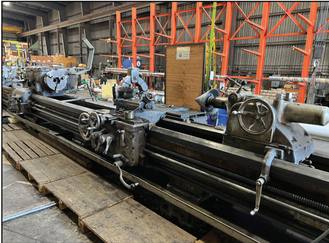
Axelson 25 28" x 216" Geared Head Lathe w/ 24' Bed, 8-555 RPM, Taper Attachment, Tailstock, Steady Rest, Indexing Tool Post, 16" 3-Jaw Chuck.
