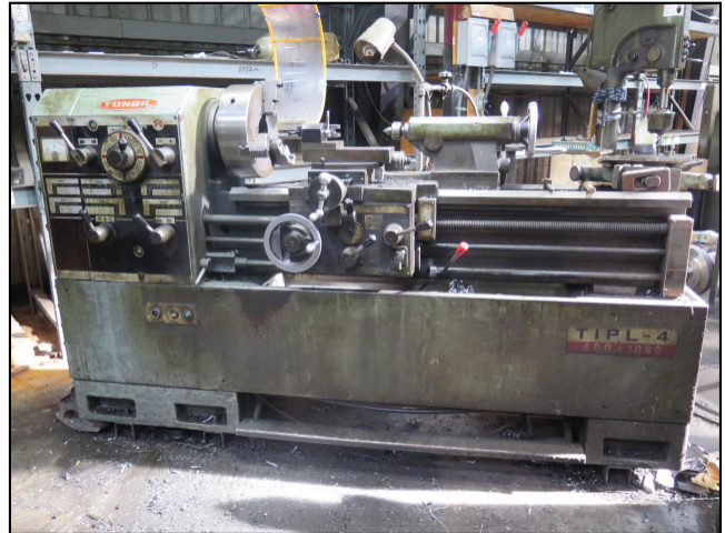
Tongil TIPL-4 15" x 42" Geared Head Gap Bed Lathe w/ 60-1500 RPM, Inch/mm Threading, Tailstock, 13" Chuck
