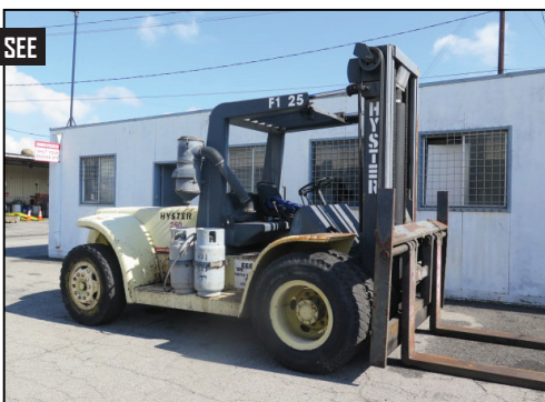
Hyster H250E 25,000 Lb Cap LPG Forklift w/ Side Shift, Solid Rear Tires
