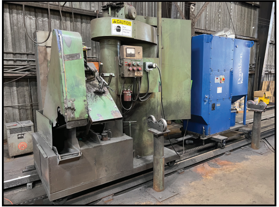
Custom Pipe Grinding Machine w/ 4" Belt Sander, Power Rotational Feed, Approx 60' Length, Donaldson Torit DF02-2 Down Flo Dust Collector s/n 15147829-L1-1.
