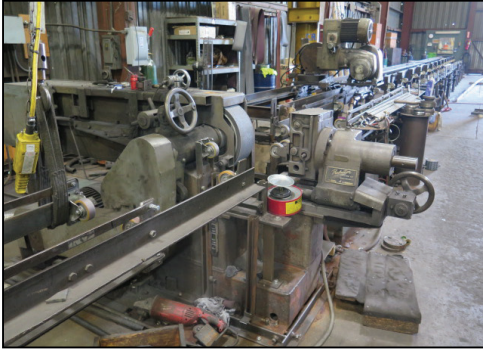
Production Machine Co Custom 6" Belt Sander / Tube Finishing Machine
