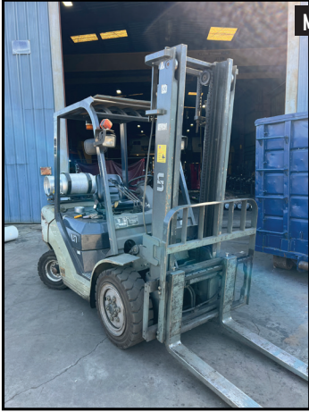
Un Sino American FL30T-JG 6600 Lb Cap LPG Forklift s/n 13L300395 w/ 2-Stage Mast, 144" Lift Height, Side Shift, Solid Yard Tires.
