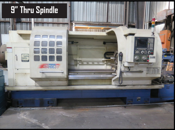
Summit "Smart Cut" SC30-9X80M Big Bore CNC Turning Center w/ Fagor Controls, 9" Thru Spindle Bore, 4-600 RPM, 8-Station Turret, Tailstock, (2) 24" 3-Jaw Chucks
