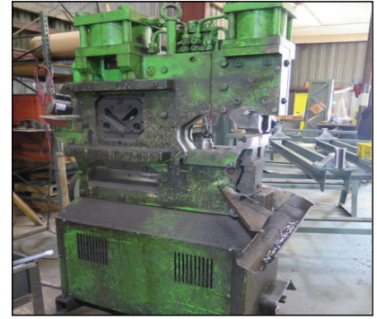
Heller / Mubeo KLSH60 60-Ton Iron Worker w/ Punch, 16" Flat Shear, Bar Shears, Angle Shear
