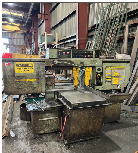
Hyd-Mech S-23P Horizontal Band Saw w/ Hyd-Mech Controls, Hydraulic Clamping, Coolant.
