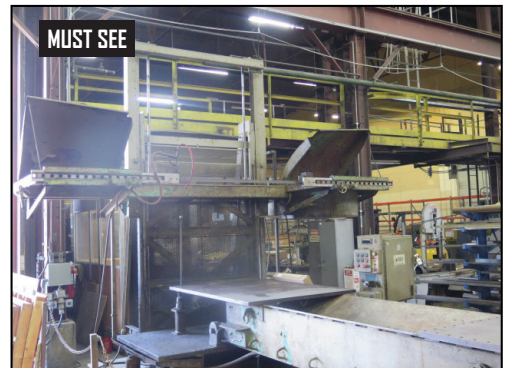
Wellsaw 1220G Special Purpose Horizontal Miter Band Saw w/ Wellsaw Controls, Adjustable Level Table
