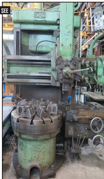
King 42" Vertical Turret Lathe w/ 6.7-200 RPM, 47" Swing, 5-Station Turret Head, Facing/Turning Head, Power Feeds, 42" 4-Jaw Chuck
