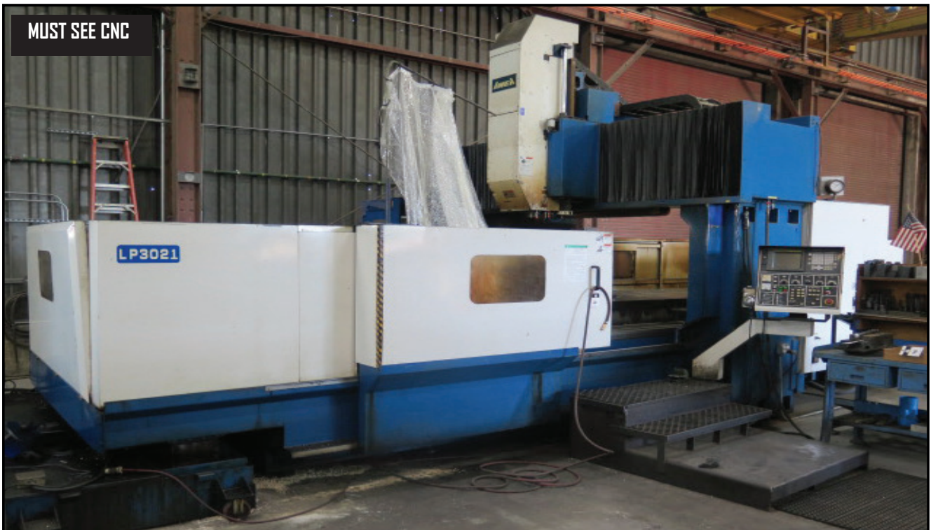
Awea LP3021 CNC Bridge Style VMC w/ Fanuc 18-M Controls, 32-ATC, CAT-50, 4000 RPM
