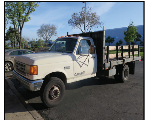
1990 Ford Super Duty Custom 12' Stake Bed Truck w/ EFI Gas Engine, Auto Trans, Dual Fuel Tanks
