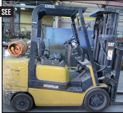
Caterpillar GC30K 3120 Lb Cap LPG Forklift w/ 3-Stage Mast, 186" Lift Height, Side Shift, Cushion Tires
