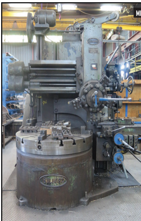
Bullard 50" Vertical Turret Lathe w/ 56" Swing, 5-Station Turret Head, Facing/Turning Head, Power Feeds, 50" 4-Jaw Chuck
