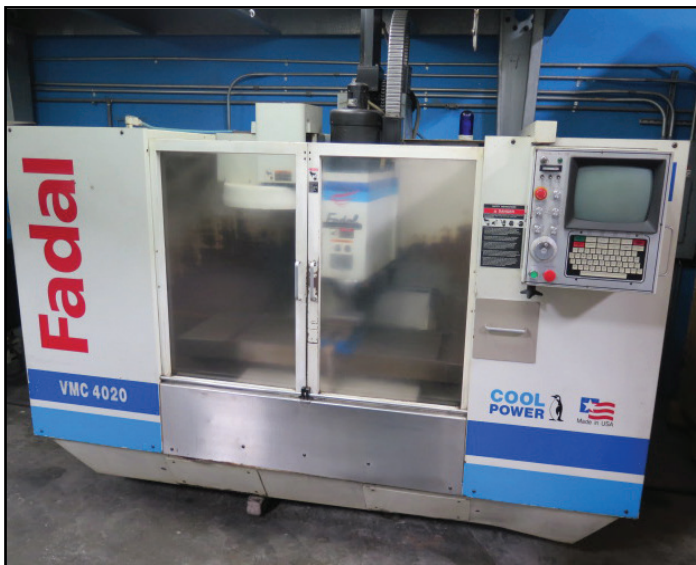
Fadal VMC4020HT 4-Axis CNC Vertical Machining Center s/n 8808659 (MISSING CONTROL BOARDS) w/ Fadal CNC88 Controls, 21-Station ATC, 40-Taper Spindle, 10,000 ROM, 20" x 48" Table.
