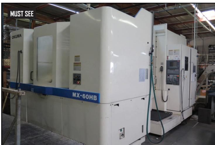
Okuma MX-60HB 2-Pallet 4-Axis CNC Horizontal Machining Center s/n 11020342 w/ Okuma OSP-U100M Controls, Tool Presetter, 60-Station ATC, CAT-50 Taper Spindle, 4 th Axis Thru Pallets, (2) 25" x 25" Pallets, Chip Conveyor, Coolant.
