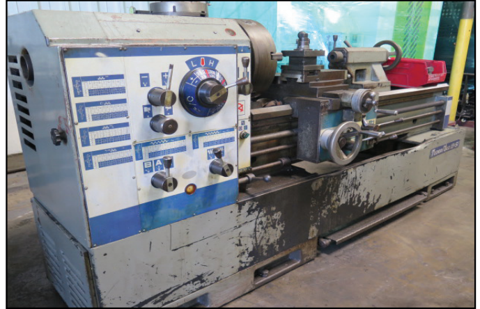
Tuda TudaMax 19X51 19" x 51" Gear-Gap Lathe w/ 25-1800 RPM, 3" Thru Spindle, Inch/mm Threading, Tailstock, 16" Chuck
