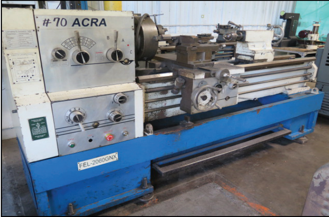
Acra FEL-2060GNX 20" x 60" Gear-Gap Lathe w/ 32-1500 RPM, 3 1/8" Thru Spindle, Inch/mm Threading, Tailstock
