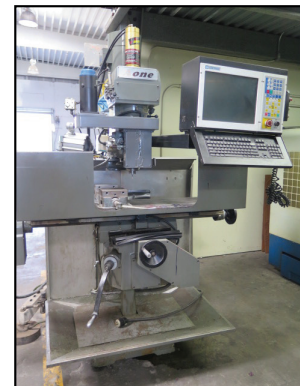
2006 Atrump "A One" 3VK WVERTER 3-Axis CNC Vertical Mill w/ Centroid Controls, R8, Power Draw-Bar, Chrome Box Ways
