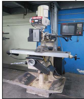
2000 Ganesh Deluxe GMV-3 3-Axis CNC Vertical Mill w/ Anilam 3300 MK Controls, 100-5200 RPM, Power Draw-Bar, Chrome Box Ways
