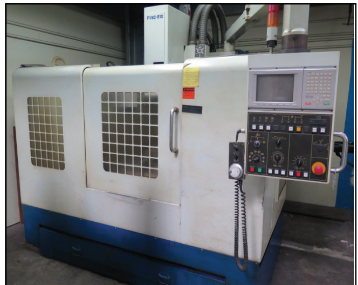
Acra FVMC-810 CNC Vertical Machining Center s/n V3013 w/ Mitsubishi Controls, 16-Station ATC, 40-Taper Spindle, 17 1/2" x 39 1/2" Table
