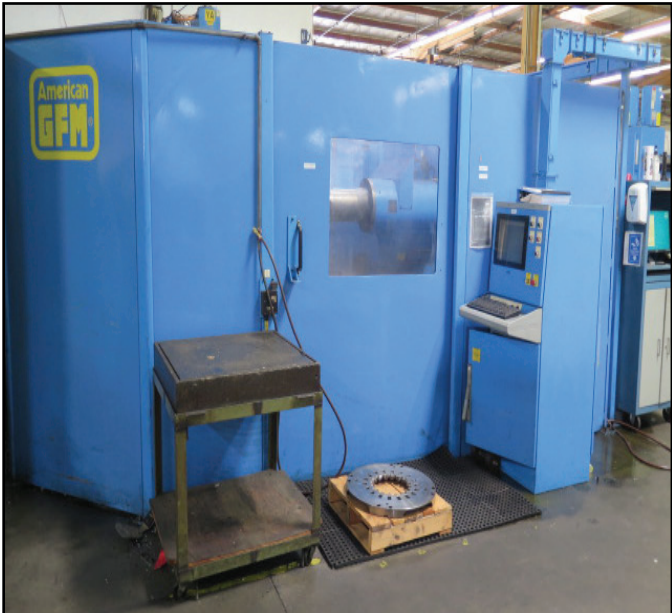
American GFM "AMS-20 CNC 6000" CNC Crank Shaft Milling Machine w/ CNC Controls.
