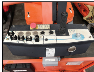
JLG TOUCAN E33MJ ELECTRIC MAN LIFT, 32.75FT MAX PLATFORM HEIGHT, 14.76 MAX HORIZONTAL REACH, POWERFINN 24V-DC CHARGER, S/N 1300052335.
