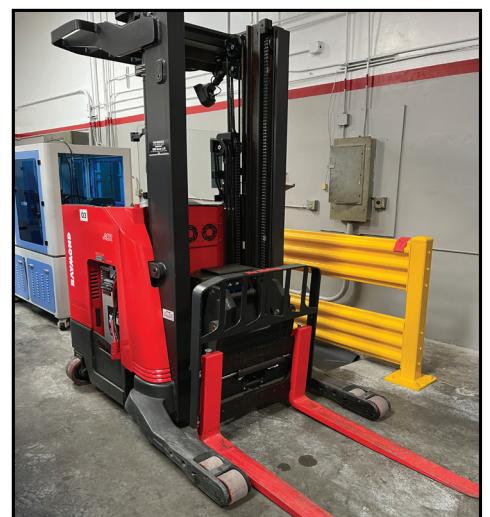
RAYMOND 720-R35TT, 3500 LB CAP DEEP REACH ELECTRIC FORKLIFT, 24V.
