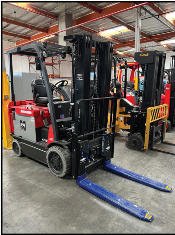
RAYMOND MODEL 4750C60, 5800 ELECTRIC FORKLIFT, 36V, SIDE SHIFTER, WITH CASCADE-RAVAS LIFT SCALE, S/N 475-16-10129.
