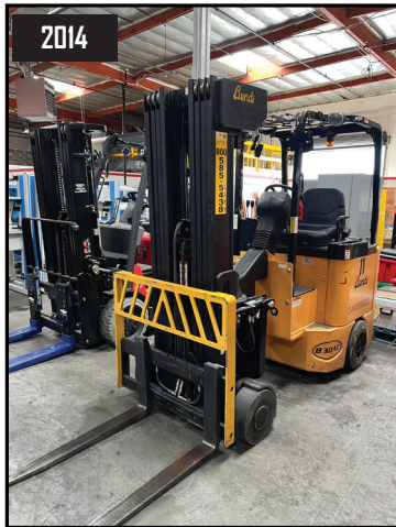
BENDI-LANDLOLL B30/42E-180DAC 3000 LB NARROW AISLE FORKLIFT, 48V, S/N B30/42AC-1105A-06581.
