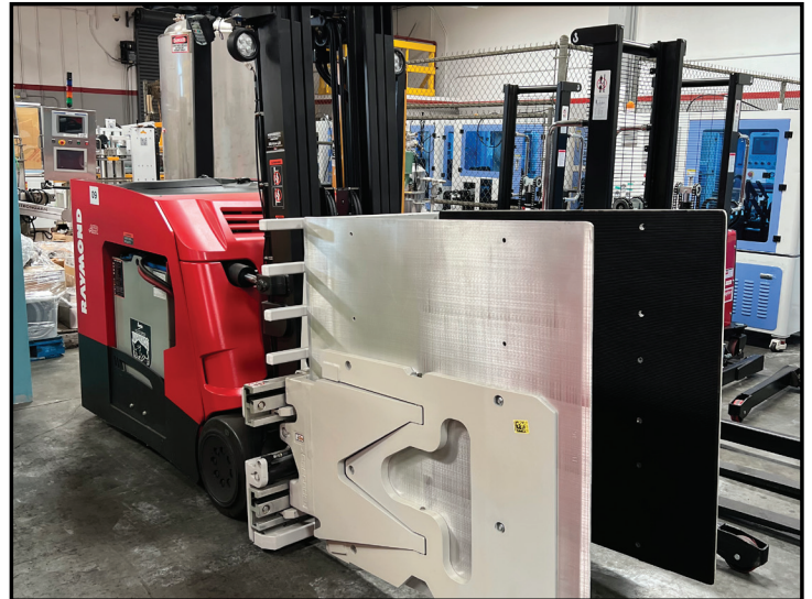
RAYMOND 425-C50TT 5000 LB CAPACITY ELECTRIC NARROW AISLE DOCKER STAND UP FORKLIFT, 36V, W/ CASCADE CARTON CLAMP ATTACHMENT, S/N 425-16-51804
