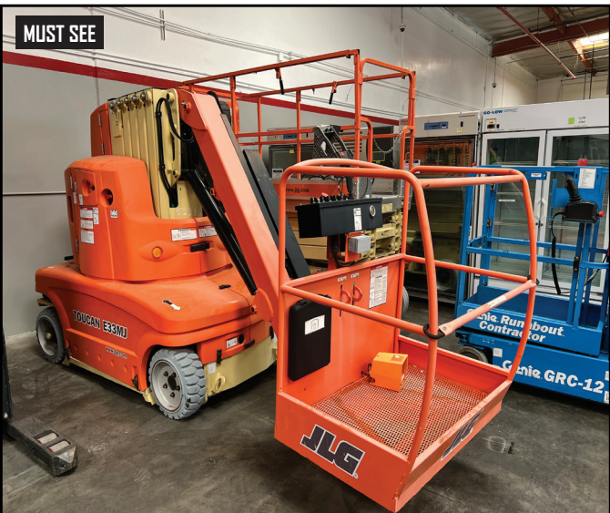
JLG TOUCAN E33MJ ELECTRIC MAN LIFT, 32.75FT MAX PLATFORM HEIGHT, 14.76 MAX HORIZONTAL REACH, POWERFINN 24V-DC CHARGER, S/N 1300052335.
