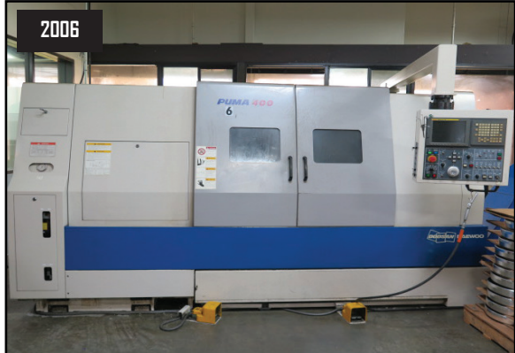
2006 2006 Doosan Daewoo PUMA 400B CNC Turning Center w/ Fanuc 21i-TB Controls, Tool Presetter, 12-Station Turret, Tailstock, 15" Power Chuck
