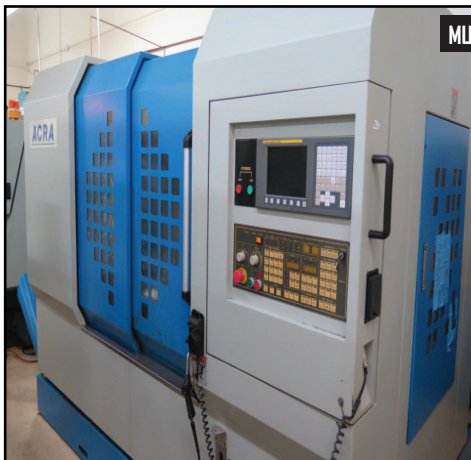
2001 Acra BVM1000 CNC VMC w/ Fanuc 0i-MC Controls, 20-Station ATC, CAT-40
