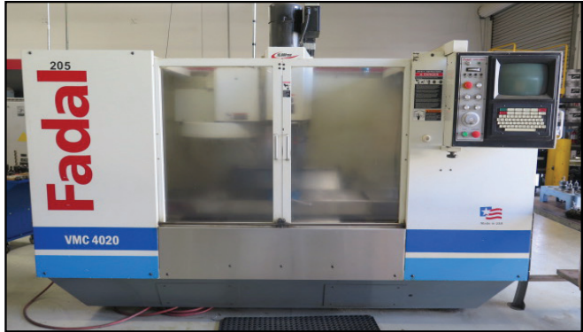
2005 Fadal VMC 4020HT CNC VMC w/ CNC88HS Controls, 21-ATC, CAT-40, 10,000 RPM, Rigid Tapping, 4meg Memory, High Torque, High Speed CPU, Graphics
