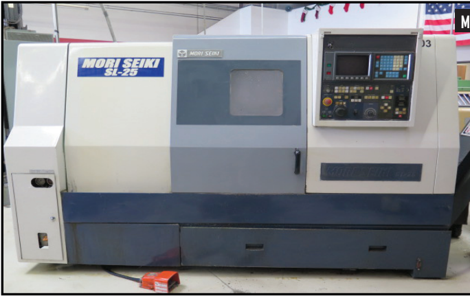
Mori Seiki SL-25S CNC Turning Center w/ Fanuc Controls, Tool Presetter, 10-Station Turret, Hydraulic Tailstock, 10" Power Chuck
