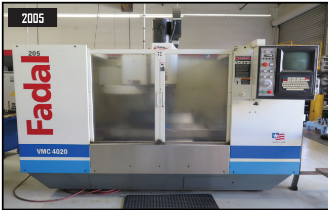
2005 Fadal VMC 4020HT CNC VMC w/ CNC88HS Controls, 21-ATC, CAT-40, 10,000 RPM, Rigid Tapping, 4meg Memory, High Torque, High Speed CPU, Graphics
