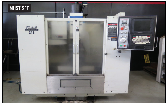
Fadal VMC15 CNC VMC w/ CNC88HS Controls, 21-ATC, CAT-40 Spindle, 7500 RPM, Rigid Tapping, 422k Memory Expansion, High Speed CPU, Graphics
