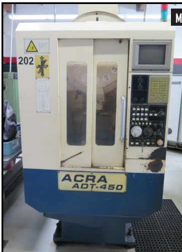
2003 Acra ADT-450 CNC Drilling / Tapping Center w/ Mitsubishi 50M Controls, 12-Station Turret, BT-30, 8000 RPM, Rigid Tapping
