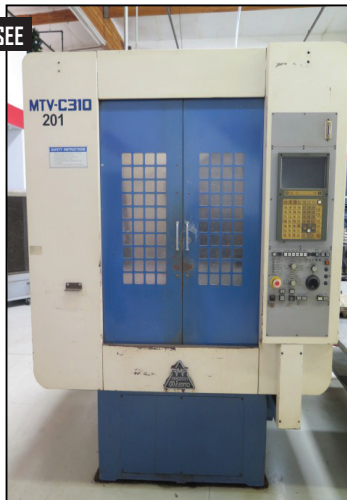
Mectron / Miyano MTC-C310 2-Pallet CNC Drilling / Tapping Center w/ Yasnac Controls, 15-Station Turret, BT-30, 16,000 RPM
