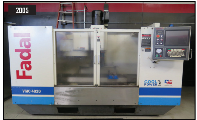
2005 Fadal VMC 4020HT CNC VMC w/ Multi Processor CNC Controls, 21-ATC, CAT-40, 10,000 RPM, Rigid Tapping, 4meg Memory, High Torque, High Speed CPU, Graphics, Metric Ball Screws
