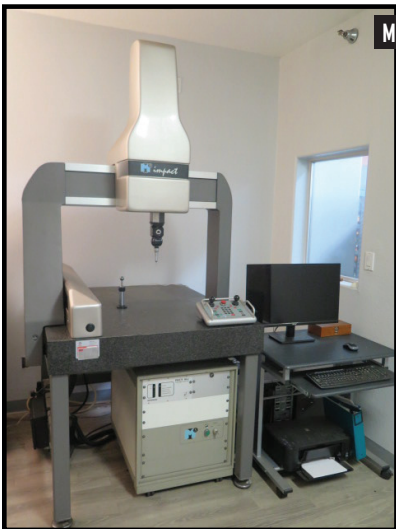
IMS "Impact" CMM w/ Renishaw PH9A Probe Head, PHC9 MK2 Probe Head Control Unit, VDMIS Software
