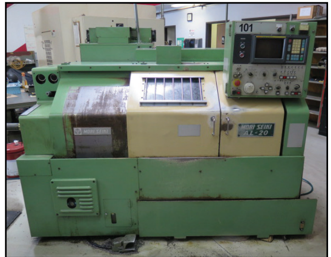
Mori Seiki AL-20 CNC Turning Center w/ Fanuc Series 0-Mate T Controls, 8-Station Turret, Hydraulic Tailstock, 5C Spindle Nose
