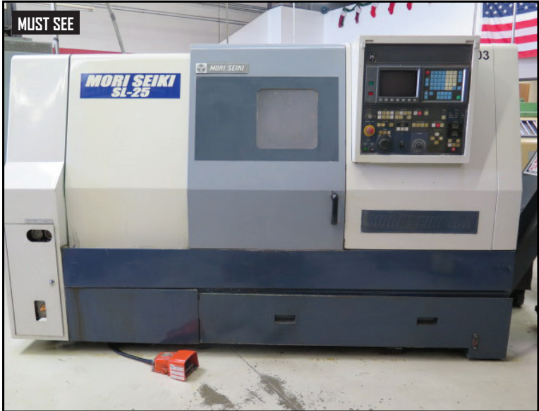
Mori Seiki SL-25BS CNC Turning Center w/ Fanuc Controls, Tool Presetter, 10-Station Turret, Hydraulic Tailstock, 10" Power Chuck
