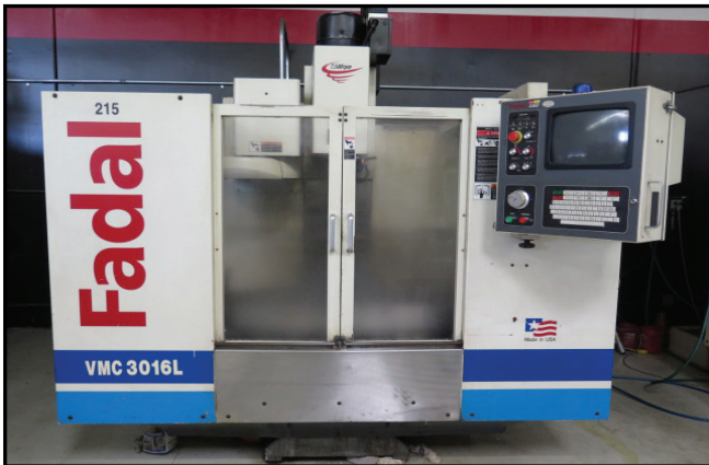
2000 Fadal VMC 3016L CNC VMC w/ Multi Processor CNC Controls, 21-ATC, CAT-40, 7500 RPM, Rigid Tapping, 28" Extended "Z" Axis, High Speed CPU, Graphics
