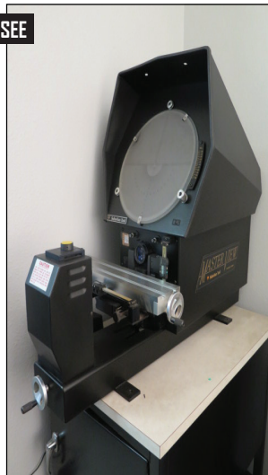
Suburban "Master View" 14" Optical Comparator w/ Mitutoyo Digital Scales, Surface and Profile Illumination
