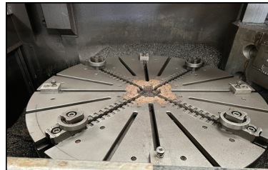
BULLARD MODEL 75 CUT MASTER VERTICAL TURRET LATHE, WITH 56" 4 JAW CHUCK, VERTICAL BORING HEAD, 5 POSITION TURRET HEAD, SIDE BORING HEAD, 2 DRO'S, S/N 30247.
