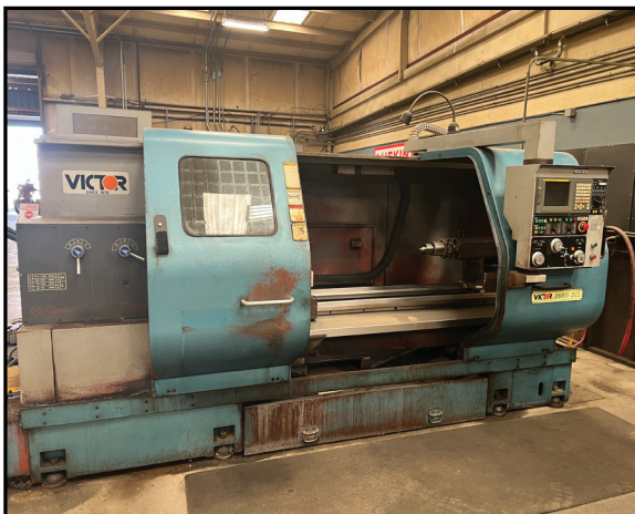
VICTOR MODEL 2680i DCL 26" X 80" CNC FLAT BED LATHE, W/ FANUC 20i-TB CONTROL, CHIP CONVEYOR.
