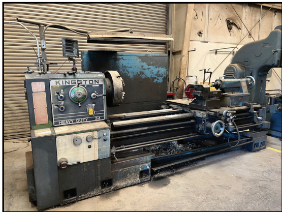
KINGSTON MODEL 34 HEAVY DUTY, 34" X 84" GAP ENGINE LATHE, 20" 4 JAW CHUCK, TAPER ATTACHMENT, NEWALL DRO, 4" THROUGH HOLE, IN/METRIC THREADING,, 8 TO 800 RPM.
