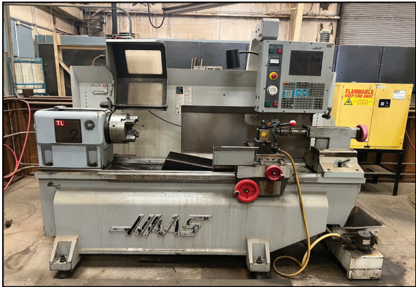
2004 HAAS TL-2 CNC LATHE, W/ 4 JAW CHUCK, TAIL STOCK, TOOL POST.
