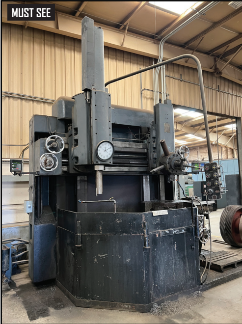
BULLARD MODEL 75 CUT MASTER VERTICAL TURRET LATHE, WITH 56" 4 JAW CHUCK, VERTICAL BORING HEAD, 5 POSITION TURRET HEAD, SIDE BORING HEAD, 2 DRO'S, S/N 30247.
