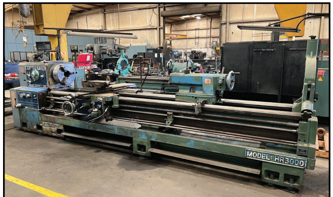
KINGSTON MODEL HR3000, 25" X 10FT GAP ENGINE LATHE, 4" THROUGH HOLE, TAPER ATTACHMENT, 3 JAW CHUCK AND 4 JAW CHUCK, TAPER ATTACHMENT, NEWALL DRO, IN/METRICK THREADING, 14 TO 800 RPM.
