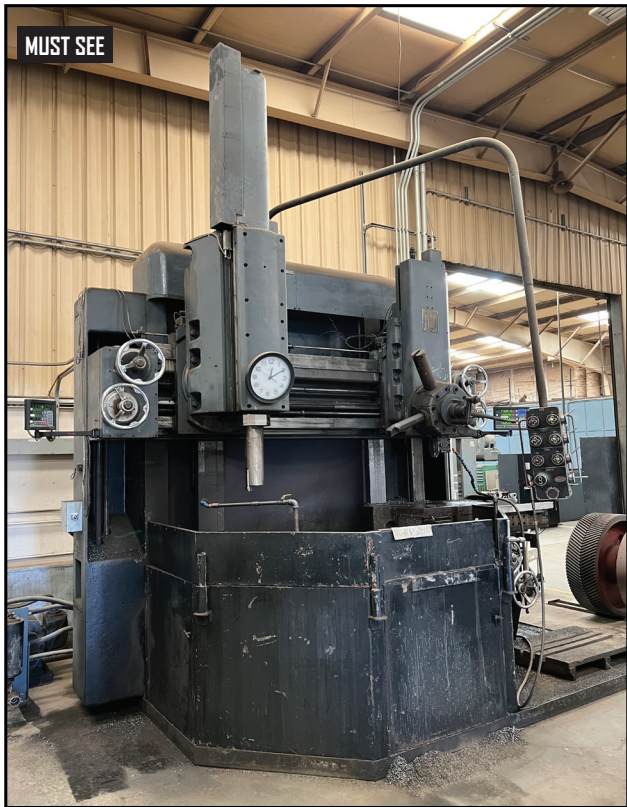
BULLARD MODEL 75 CUT MASTER VERTICAL TURRET LATHE, WITH 56" 4 JAW CHUCK, VERTICAL BORING HEAD, 5 POSITION TURRET HEAD, SIDE BORING HEAD, 2 DRO'S, S/N 30247.
