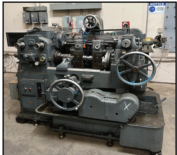
W.E. SYKES HARRINGBONE GEAR GENERATOR.
