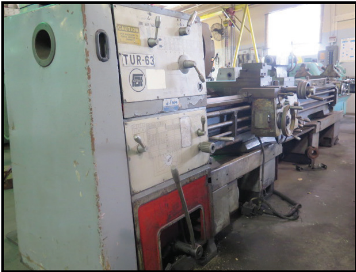
Ponar TUR-63 Geared Head Lathe w/ 4" Thru Spindle Bore, 18-1800 RPM, Taper Attach
