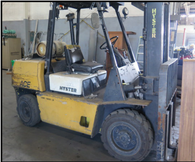
Hyster H90XLS 7000 Lb Cap LPG Forklift w/ 2-Stage Mast, 119" Lift Height, Pneumatic Yard Tires
