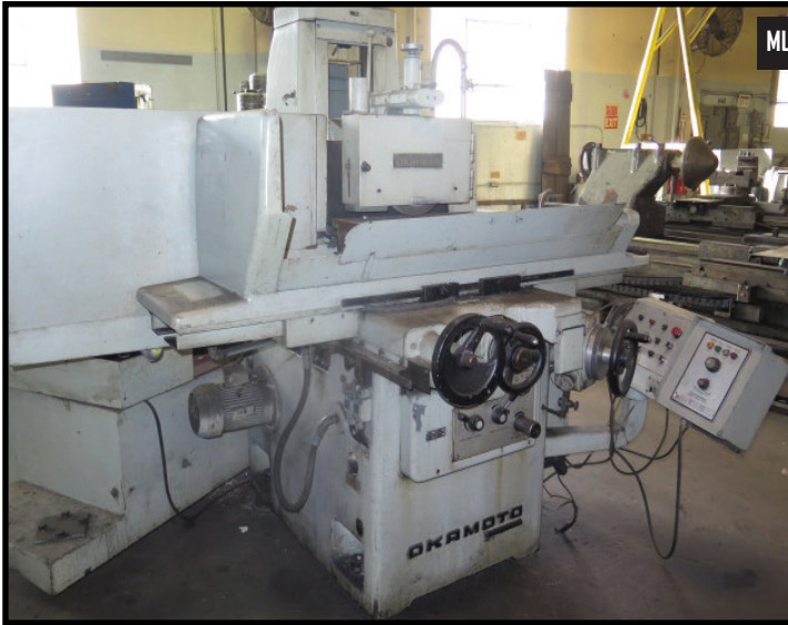
Okamoto Accugar-124N 12" x 24" Automatic Surface Grinder
