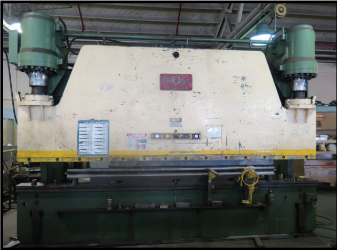
Chicago 300-F-12 300 Ton x 12' Hydraulic Power Press Brake w/ Manual Back Gage
