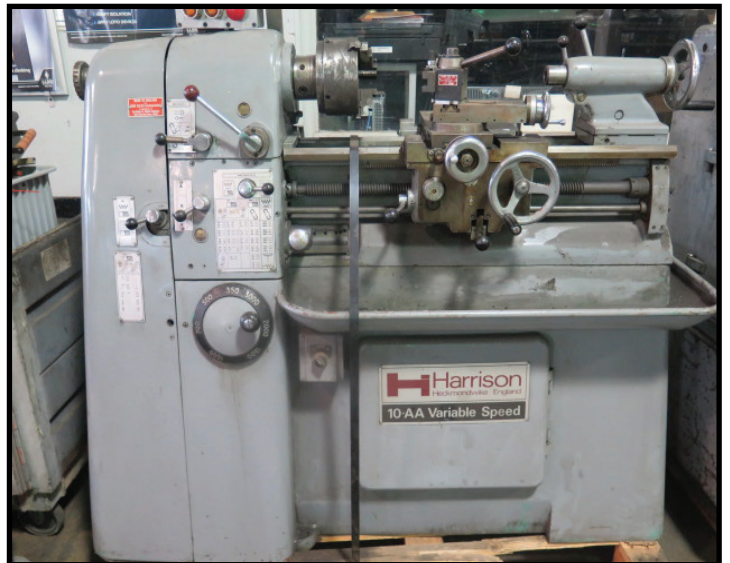
Harrison 10-AA Variable Speed 11" x 16" Tool Room Lathe
