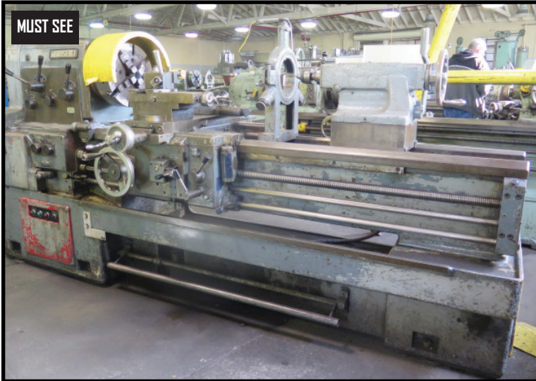
Mori Seiki MH-1500 24" x 60" Geared Head Gap Bed Lathe w/ 27-1205 RPM, Inch threading, Tailstock
