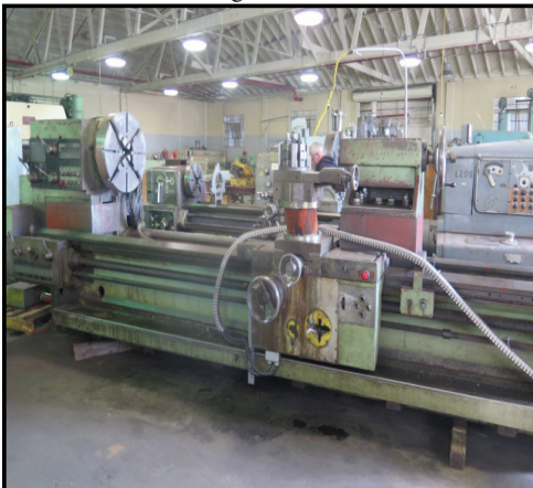
TOS SUS-80 50" x 140" Geared Head Gap Bed Lathe w/ 9" Riser, 7.1-900 RPM, Inch/mm Threading, Tailstock
