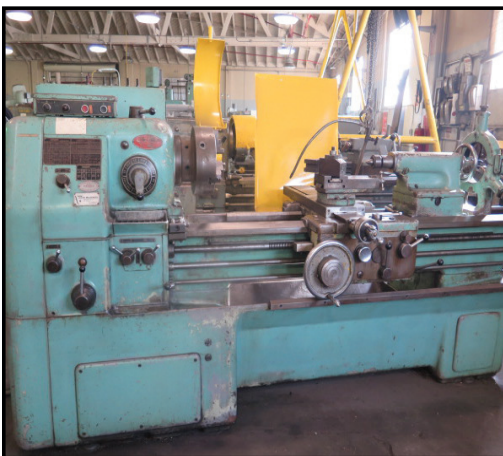
Okuma LS 22" x 60" Geared Head Gap Bed Lathe w/ 35-1800 RPM, Inch Threading, Tailstock
