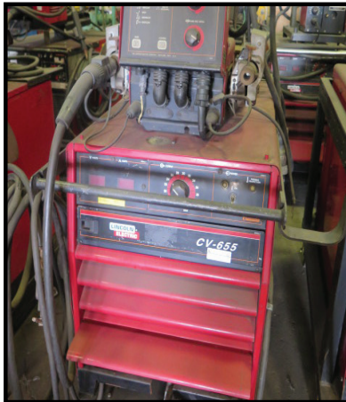
Lincoln CV-655 Arc Welding Power Source w/ DN10 Dual Wire Feed
