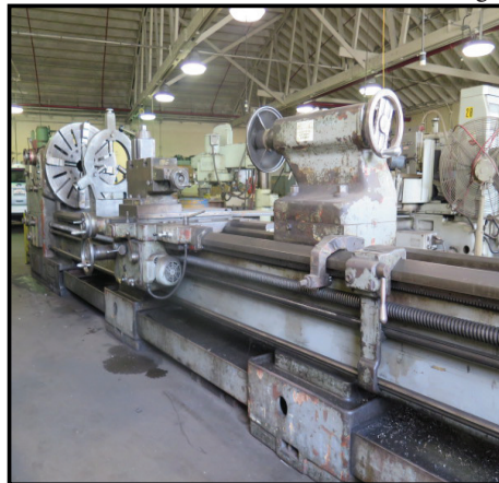
PBR TM-500 Big Bore Gap Bed Lathe w/ 90-800 RPM, 5 7/8" Thru Spindle Bore, Taper Attach, Inch/mm Threading, Tailstock
