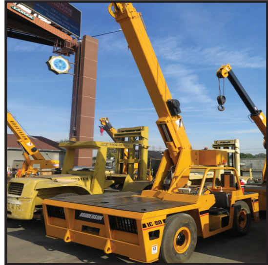
Broderick IC-80-3F 18,000 Lb Cap (On Outriggers) Diesel Carry Deck Crane w/ 40' Reach
