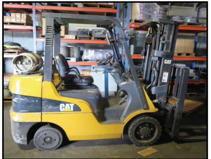
Caterpillar GP30 5300 Lb Cap LPG Forklift w/ 3-Stage Mast, Side Shift
