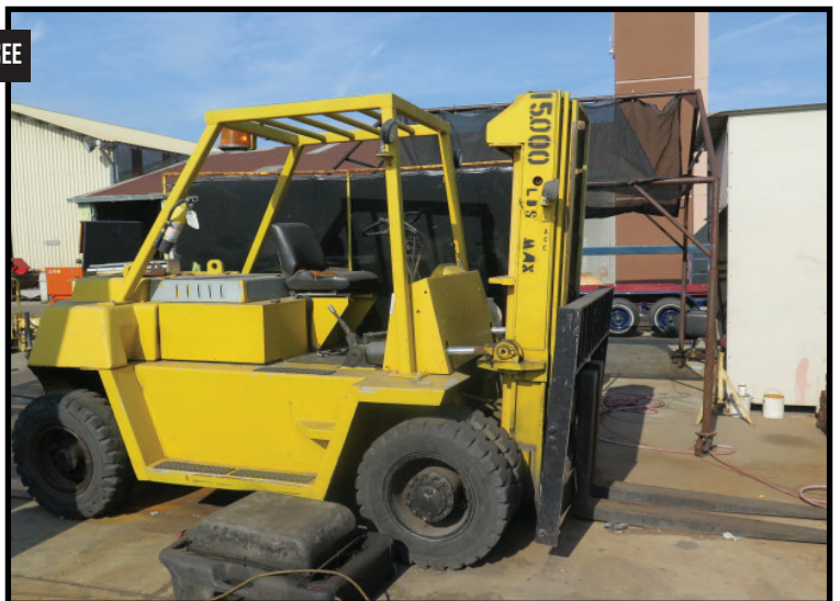
Komatsu 15,000 Lb Cap Diesel Forklift w/ 2-Stage Mast, Solid Yard Tires
