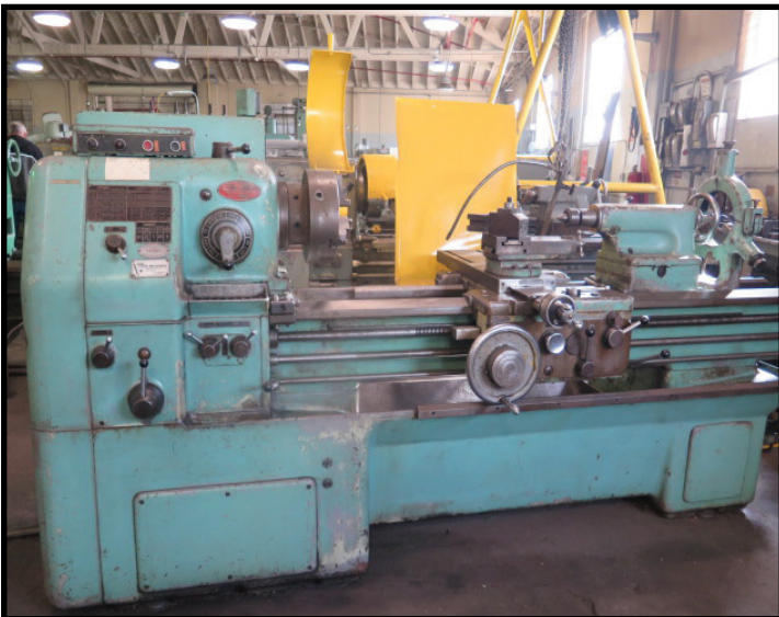
Okuma LS 22" x 60" Geared Head Gap Bed Lathe w/ 35-1800 RPM, Inch Threading, Tailstock
