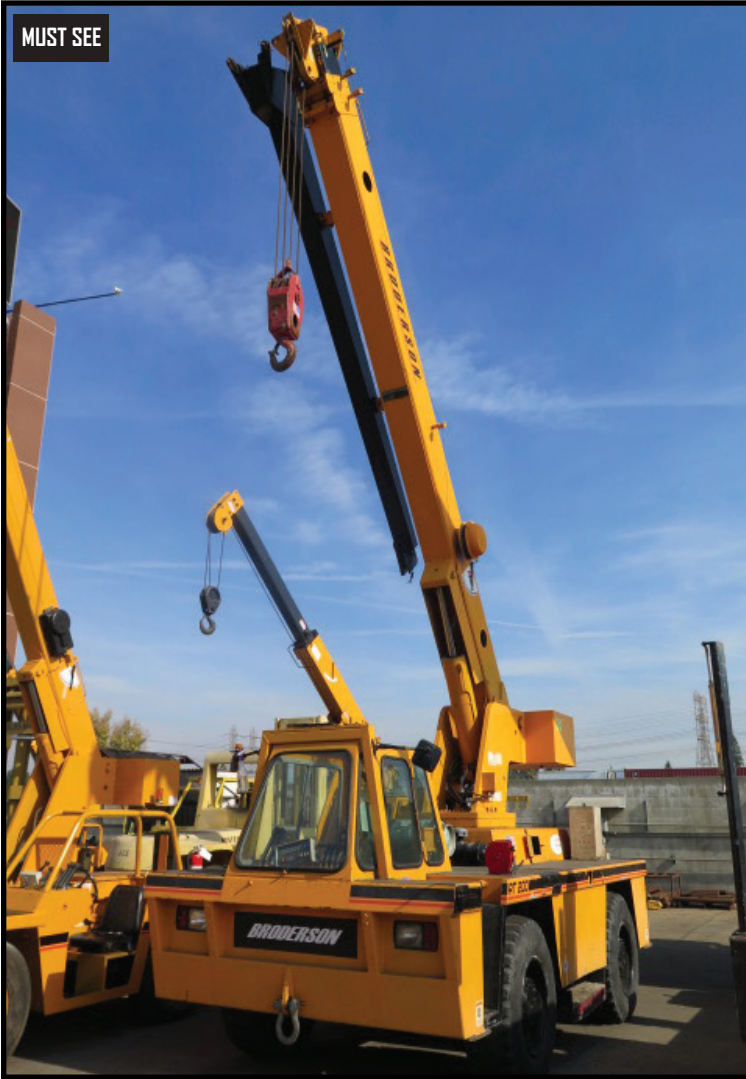
Broderick RT200-3A 30,000 Lb Cap (On Outriggers) LPG Carry Deck Crane w/ 59' Reach
