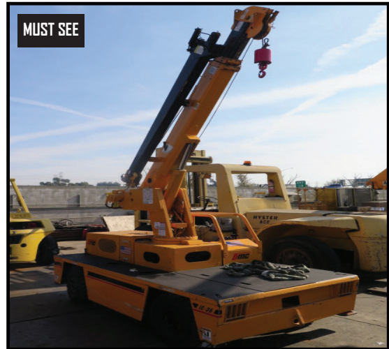
Broderick IC-35 8000 Lb Cap (On Outriggers) LPG Carry Deck Crane w/ 30' Reach, 26' Max Height
