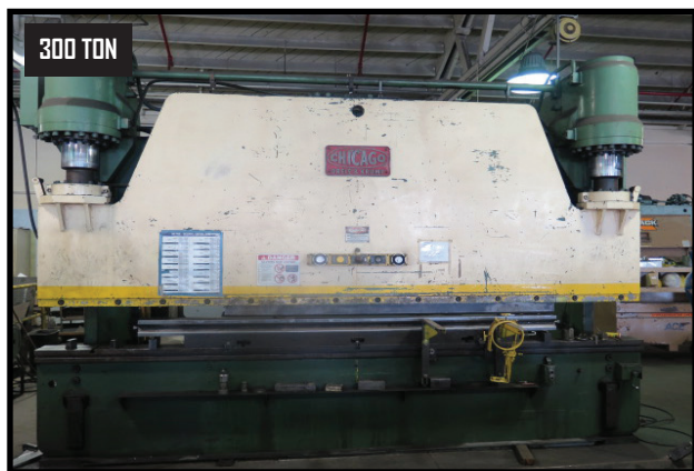
Chicago 300-F-12 300 Ton x 12' Hydraulic Power Press Brake w/ Manual Back Gage
