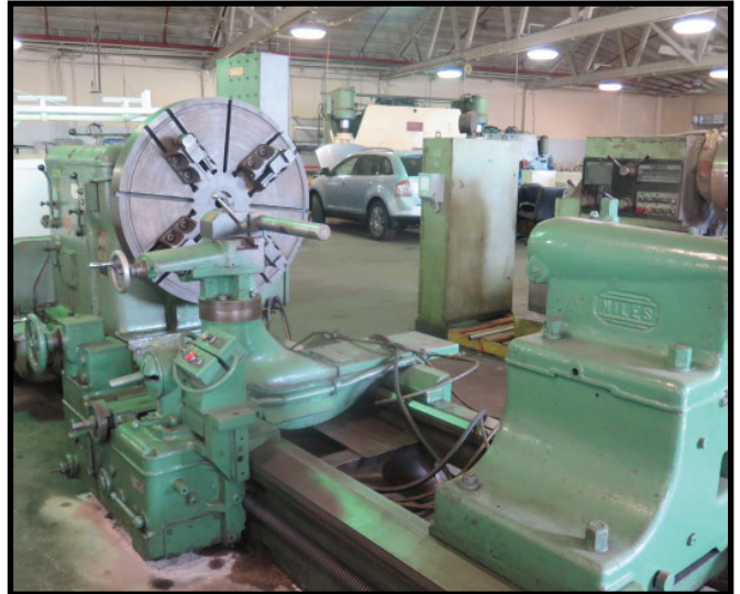
Niles A54P 62" x 140" Lathe s/n 23579 w/ 3.94-232 RPM, Inch Threading, Tailstock, Steady Rest
