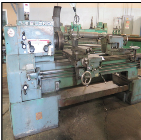
LeBlond Regal 19" x 58" Geared Head Lathe w/ 40-1600 RPM, Inch Threading, Tailstock
