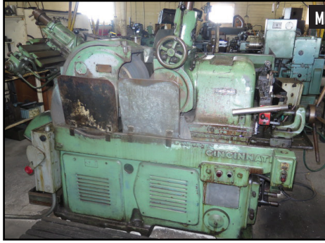
Cincinnati EA Centerless Grinder w/ Hydraulic Grinding Wheel Dresser, Manual Feed Wheel Dresser, Bellows-Velvac BSE-5BD Kicker Attachment
