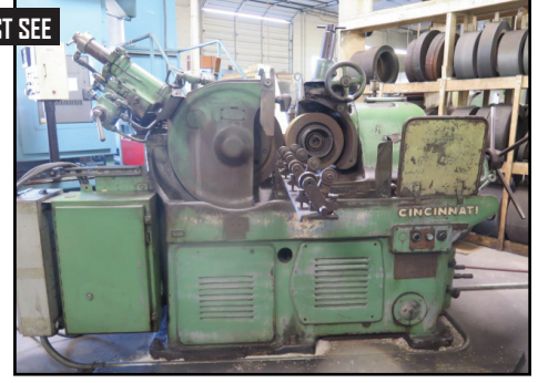
Cincinnati EA Centerless Grinder w/ Hydraulic Grinding Wheel Dresser, Manual Feed Wheel Dresser
