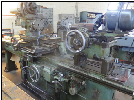
Heald 72-A ID Grinder w/ Cross Slide Assembly, 7" Riser, Motorized Work Head, Red Head Grinding Head
