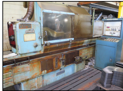
Ex-Cell-O Style 50 NC Thread Grinding Machine w/ Marposh Controls, Work Head, Tailstock
