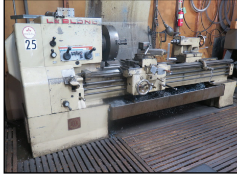
LeBlond Regal 26" x 72" Geared Head Lathe w/ 27-1080 RPM, Inch Threading, Tailstock, 18" Chuck
