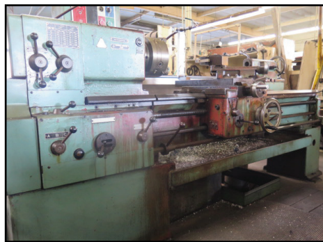
TOS SN50B 20" x 65" Geared Head Lathe w/ 22.4-2000 RPM, Inch Threading, Taper Attachment, Tailstock, Steady and Follow Rests
