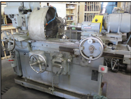
Heald 72-A ID Grinder w/ Motorized Work Head, Red Head Grinding Head
