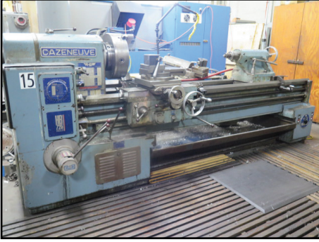
Cazeneuve HB725 26" x 74" Gap Bed Lathe w/ 60-1600 RPM, Inch/mm Threading, Tailstock, 3 3/16" Thru Spindle Bore, Trava-Dial, 16" Chuck
