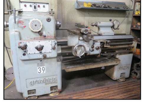
Graziano Tortona SAG14 14" x 39" Lathe w/ 70-1800 RPM, Inch/mm Threading, Tailstock, Steady Rest, Trava-Dial, 5C
