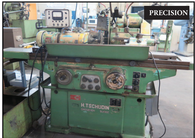
H. Tschudin HTG-600 Cylindrical Grinder w/ Motorized Work Head, Tailstock, Movomatic CR100TH Electronic Sizer
