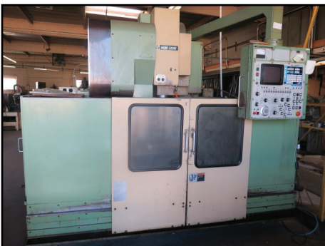
Mori Seiki MV-35/40 CNC VMC w/ Yasnac MX-1 Controls, 20-Station ATC, BT-40 Taper Spindle
