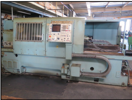
Mori Seiki TL-5 CNC Turning Center w/ Fanuc 6T Controls, 8-Station Turret, Hydraulic Tailstock, 12" 3-Jaw Chuck
