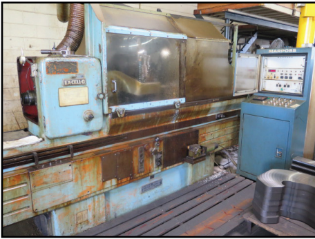
Ex-Cell-O Style 50 NC Thread Grinding Machine w/ Marposh Controls, Work Head, Tailstock
