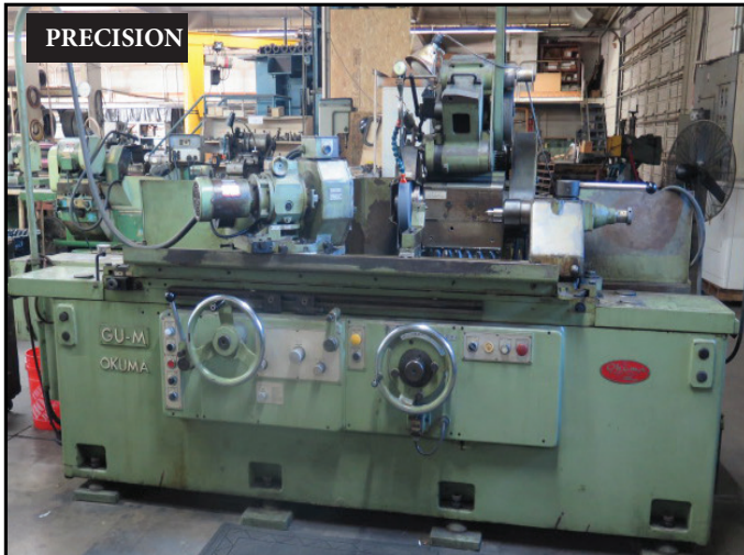
Okuma GU-M 12.6" x 39" Cylindrical Grinder s/n 5508-2515 w/ Motorized Miter Work Head, Tailstock, Coolant.
