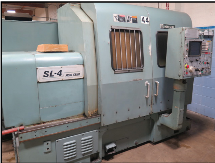
Mori Seiki SL-4A CNC Turning Center w/ Fanuc 6T Controls, 10-Station Turret, Hydraulic Tailstock, 2500 RPM, 10" 3-Jaw Chuck
