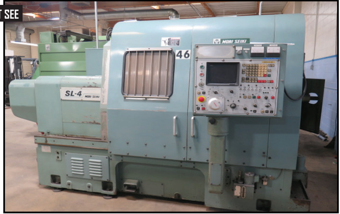
Mori Seiki SL-4A CNC Turning Center w/ Fanuc 6T Controls, 10-Station Turret, Hydraulic Tailstock, 2500 RPM, 10 1/2" 3-Jaw Chuck
