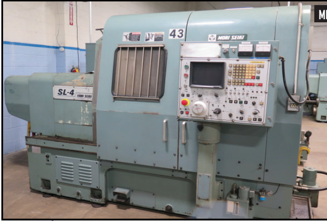
Mori Seiki SL-4A CNC Turning Center w/ Fanuc 6T Controls, 10-Station Turret, Hydraulic Tailstock, 2500 RPM, 10 1/2" 3-Jaw Chuck
