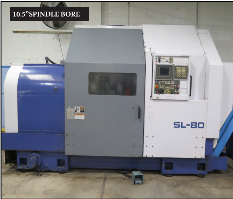
1997 Mori Seiki SL-80 Big Bore CNC Turning Center w/ Mori Seiki SC-518 Controls, 10 1/2" Thru Spindle Bore, 6-Station Turret, 4-550 RPM, 33" 3-Jaw Chuck with 16" Bore
