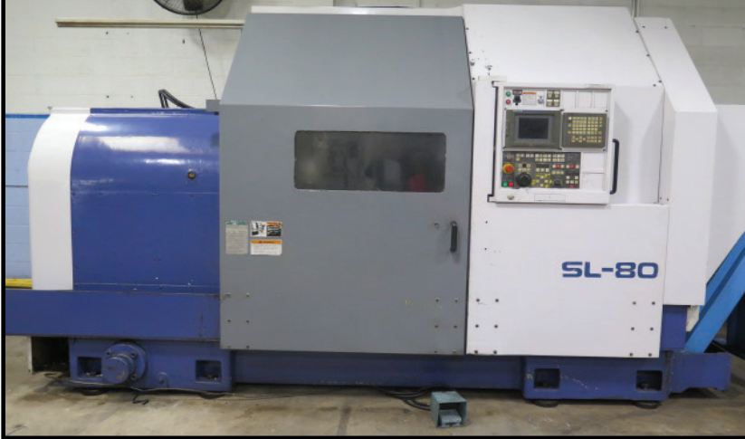
1997 Mori Seiki SL-80 Big Bore CNC Turning Center w/ Mori Seiki SC-518 Controls, 10 1/2" Thru Spindle Bore, 6-Station Turret, 4-550 RPM, 33" 3-Jaw Chuck with 16" Bore
