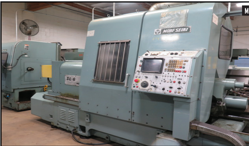
Mori Seiki SL-6 CNC Turning Center w/ Fanuc 6T Controls, 12-Station Turret, Hydraulic Tailstock, 18" 3-Jaw Chuck
