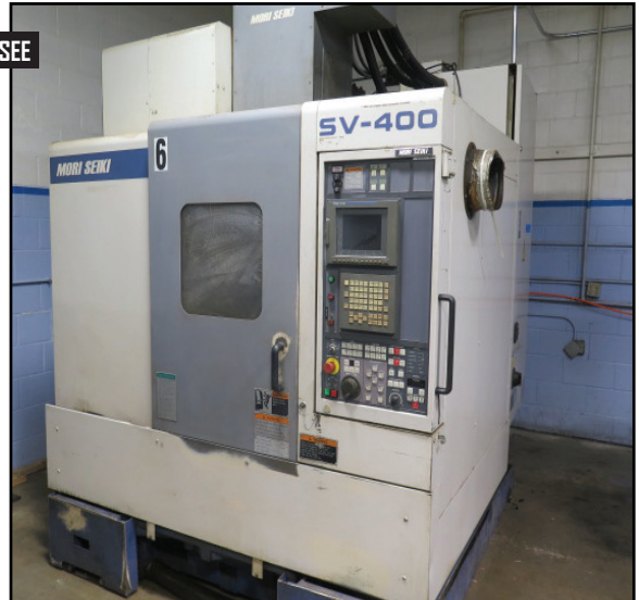
Mori Seiki SV-400 5-Axis CNC Vertical Machining Center s/n 157 w/Mori Seiki MSC-518 Controls, 30-Station Side Mount ATC, BT-40 Taper Spindle, 19 1/2" x 35 1/2" Table, Coolant, (2006) Nikken 5AX-130FA 4-5 Axis Trunnion Style Rotary Head
