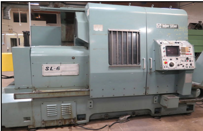
Mori Seiki SL-6B CNC Turning Center w/ Fanuc 6T Controls, 12-Station Turret, Hydraulic Tailstock, 18" 3-Jaw Chuck
