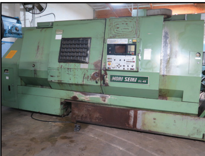
Mori Seiki SL-45A CNC Turning Center w/ Fanuc 10T Controls, 12-Station Turret, Hydraulic Tailstock, 16" 3-Jaw Chuck
