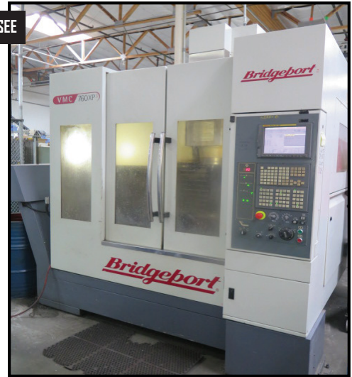
2005 Bridgeport VMC760 XP3 CNC VMC w/ Fanuc 18i-MB Controls, 30-ATC, CAT-40 Spindle, 12,000 RPM, Rigid Tapping,
