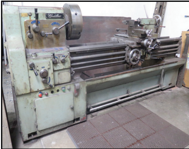
Cadillac 2260 22" x 60" Lathe w/ 25-1500 RPM, Inch Threading, Tailstock, Steady Rest, Trava-Dial, 16" Chuck
