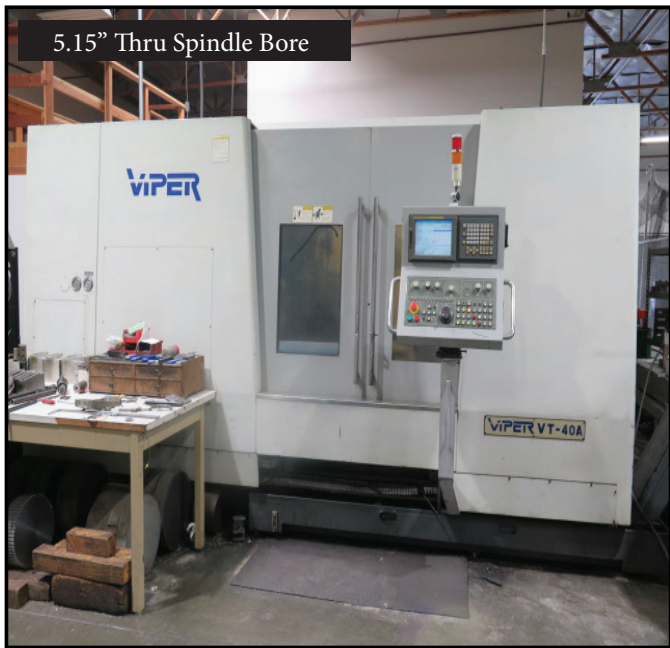
2005 Viper VT-40A CNC Turning Center w/ Fanuc 21i-TB Controls, 12-Station Turret, Hydraulic Tailstock, 2000 RPM, 5.15" Thru Spindle Bore, 33.8" Max Dia., 18" Power Chuck
