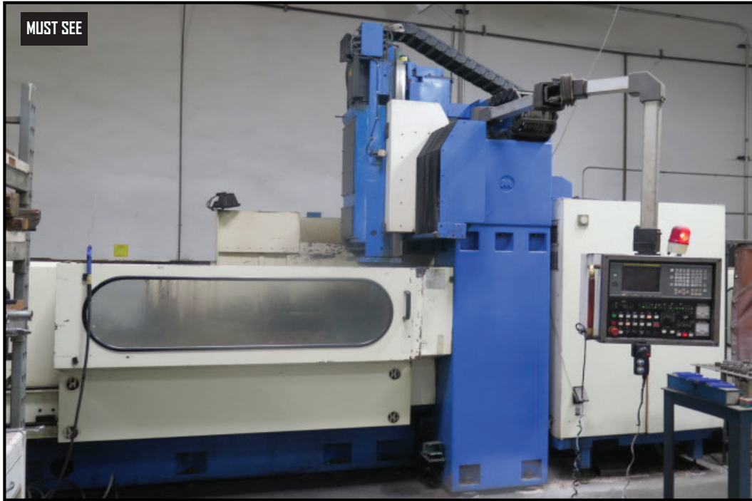
1998 Kao Ming KMC-3000 SD CNC Gantry Style Machining Center s/n 38099 w/ Fanuc Series 18-M Controls, Hand Wheel, 30-Station ATC, CAT-50 Taper Spindle, 4000 RPM, Travels X=124", Y=55", Z=27.5", 118" x 49" Table, Harbor Oil Cooler, Chip Augers, Chip Conveyor, Coolant.
