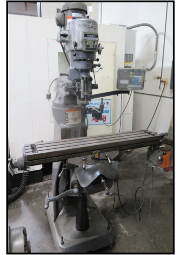
Bridgeport Vertical Mill w/ Jing JCS900-2AE DRO, 2Hp, 60-4200 Dial RPM, Chrome Ways, Power Feed
