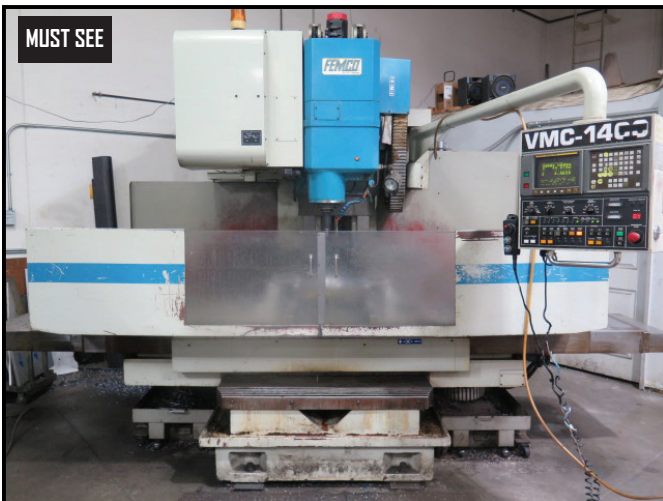
1996 Femco VMC-1400 CNC Vertical Machining Center s/n 018220 w/ Fanuc Series 0-M Controls, Hand Wheel, 30-Station ATC, CAT-50 Taper Spindle, 4500 RPM, Rigid Tapping, Travels X=55.9", Y=30.4", Z=30.3", Harbor Oil Cooler, 67" x 29 1/2" Table, Chip Auger, Coolant.
