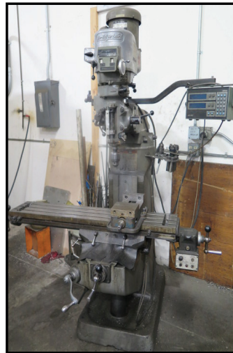
Bridgeport Vertical Mill w/ Acu-Rite MillMate DRO, 2Hp, 60-4200 Dial RPM, Chrome Ways, Power Feed
