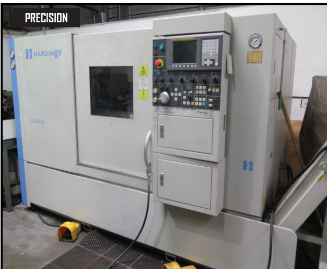
Hardinge GS 200/66 CNC Turning Center w/ Fanuc 0i-TC Controls, 12-Station Turret, Hydraulic Tailstock, 4200 RPM, 8" Power Chuck
