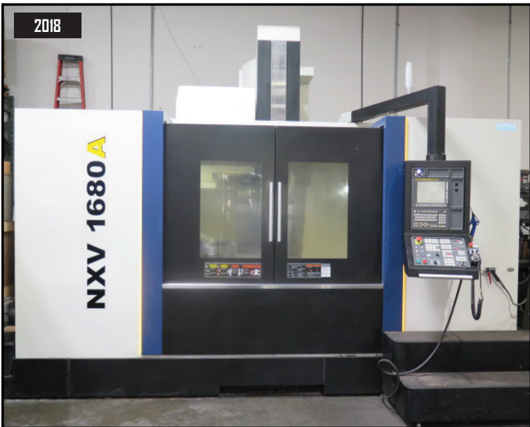
2018 YCM NXV1680A CNC VMC w/ Fanuc MXP-200FP Controls, 30-ATC, CAT-40 Spindle, 12,000 RPM, Rigid Tapping
