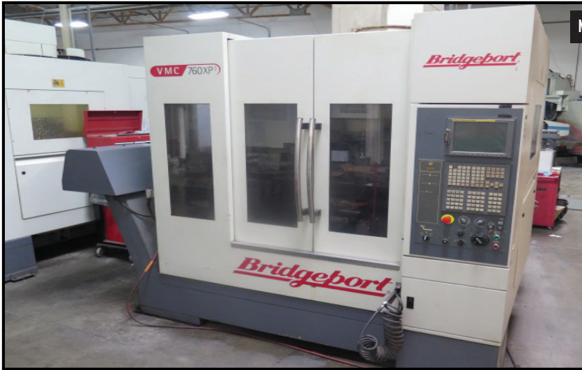
2005 Bridgeport VMC760 XP3 CNC VMC w/ Fanuc 18i-MB Controls, 30-ATC, BT-40Taper, 12,000 RPM, Rigid Tapping
