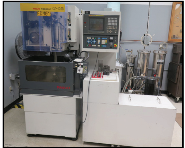
Fanuc Robotuc α-0B CNC Wire EDM Machine s/n P9520B201 w/ Fanuc Series 16-W Controls, Hand Controller, Ebbco Dielectric Coolant and Filtration System.
