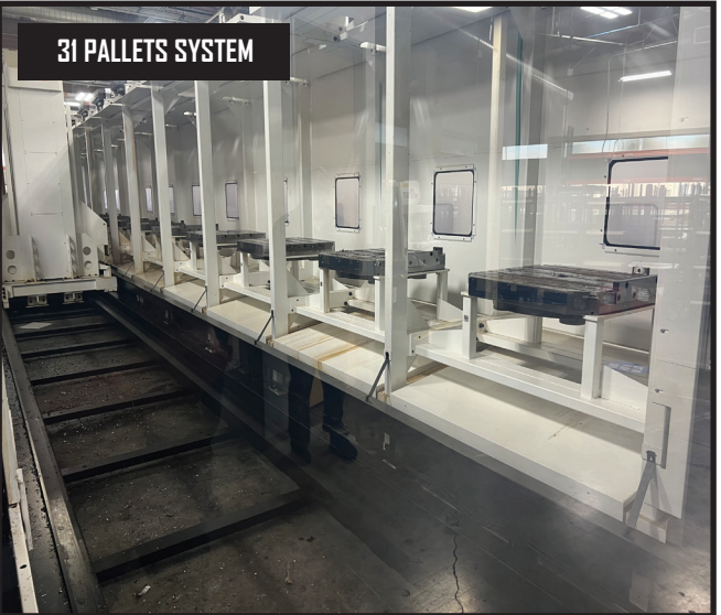
Mazak Pallettech High Rise 31-Station Pallet System w/ Mazatrol Nexus 2 Controls, Mazak PMC-Web System Monitor, (2) Loading Stations, 31 Pallets.
