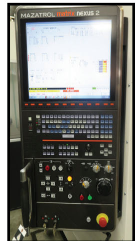
Mazak Nexus 530C-II HS 2-Pallet CHC Vertical Machining Center s/n 273302 w/ Mazatrol Matrix Nexus 2 Controls, Hand Wheel, 48-Station ATC, CAT-40 Taper pindle, 18,000 RPM, Renishaw OTS Wireless Tool Touch Probe, Renishaw Wireless Probing System with CAT-40 Taper Probe Head, Mazak Superflow T8/1000 1000psi Coolant and Filtration System, Oil Cooler, Chip Augers, Chip Conveyor.
