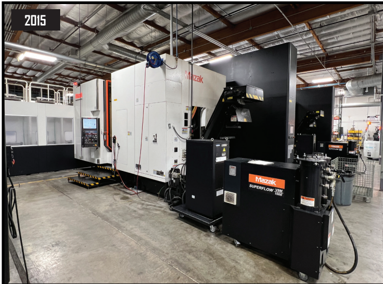
2/2015 Mazak Nexus 6800-II 4-Axis CNC Horizontal Machining Center s/n 261528 w/ Mazatrol Matrix Nexus 2 Controls, Hand Wheel, 240-Station ATC, HSK-100 Spindle, 16,000 RPM Spindle, Laser Tool Presetter, Renishaw Wireless Probing System with Probe Head, 4th Axis Thru Pallets, 24.8" x 24.8" Pallet, Mazak Superflow V8M/1000 1000psi Coolant and Filtration System, Oilmatic Oil Cooler, Chip Augers, Chip Conveyor.
