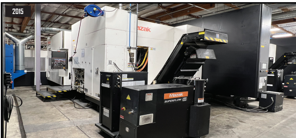
8/2015 Mazak Nexus 8800-II 4-Axis CNC Horizontal Machining Center s/n 265675 (NEEDS SPINDLE REBUILD) w/ Mazatrol Matrix Nexus 2 Controls, Hand Wheel, 240-Station ATC, HSK-100 Spindle, 16,000 RPM, Laser Tool Presetter, Renishaw Wireless Probing System with Probe Head, 4 th Axis Thru Pallets, 31.5" x 31.5" Pallets, Mazak Superflow V8M/1000 1000psi Coolant and Filtration System, Oilmatic Oil Cooler, Chip Augers, Chip Conveyor.
