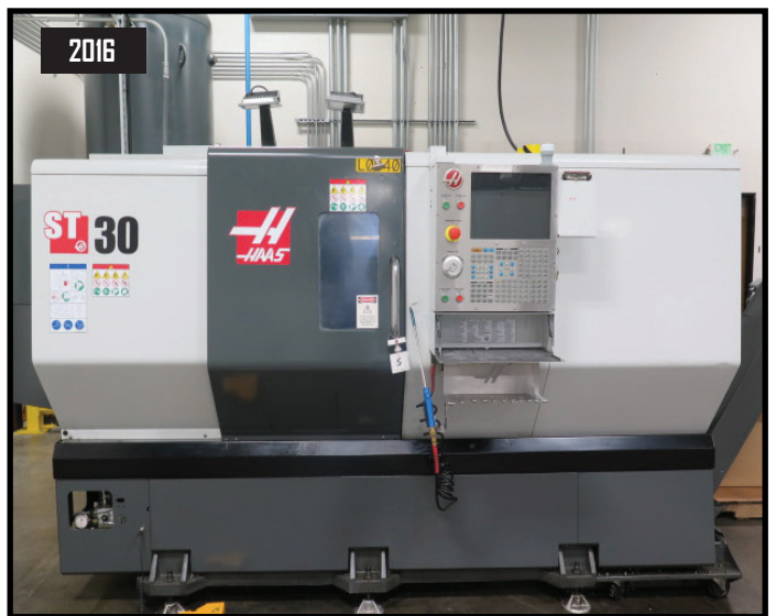
9/2016 Haas ST-30 CNC Turning Center s/n 3106116 w/ Haas Controls, Tool Presetter, 12-Station Turret, 3200 RPM, Rigid Tapping, M19 Spindle Orientation, Quick Code, 12" 3-Jaw Power Chuck, Chip Conveyor, High Flow Coolant.
