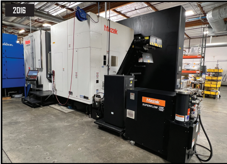
12/2016 Mazak Smooth Tech HCN-6800 4-Axis CNC Horizontal Machining Center s/n 279174 w/ Mazak Smooth-G Controls, Digital Hand Wheel, 240-Station ATC, HSK-100 Spindle, 16,000 RPM Spindle, Laser Tool Presetter, Renishaw Wireless Probing System with Probe Head, 4th Axis Thru Pallets, 24.8" x 24.8" Pallet, Mazak Superflow V8M/1000 1000psi Coolant and Filtration System, Oilmatic Oil Cooler, Chip Augers, Chip Conveyor.
