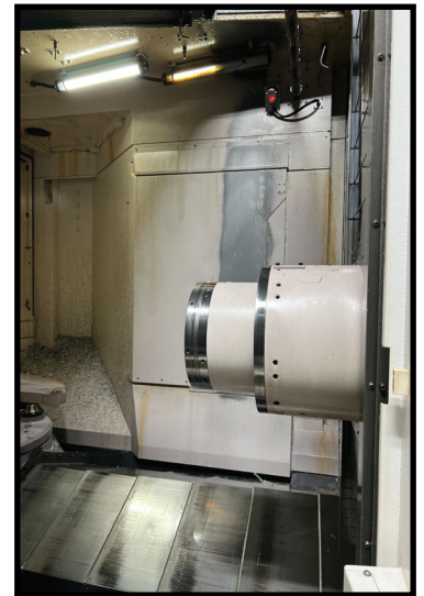
11/2016 Mazak Smooth Tech HCN-8800 4-Axis CNC Horizontal Machining Center s/n 279180 w/ Mazatrol Smooth-G Controls, Digital Hand Wheel, 240-Station ATC, HSK-100 Spindle, 16,000 RPM, Laser Tool Presetter, Renishaw Wireless Probing System with Probe Head, 4 th Axis Thru Pallets, 31.5" x 31.5" Pallets, Mazak Superflow V8M/1000 1000psi Collant and Filtration System, Oilmatic Oil Cooler, Chip Augers, Chip Conveyor.
