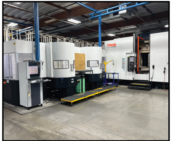
12/2016 Mazak Smooth Tech HCN-6800 4-Axis CNC Horizontal Machining Center s/n 279174 w/ Mazak Smooth-G Controls, Digital Hand Wheel, 240-Station ATC, HSK-100 Spindle, 16,000 RPM Spindle, Laser Tool Presetter, Renishaw Wireless Probing System with Probe Head, 4th Axis Thru Pallets, 24.8" x 24.8" Pallet, Mazak Superflow V8M/1000 1000psi Coolant and Filtration System, Oilmatic Oil Cooler, Chip Augers, Chip Conveyor.
