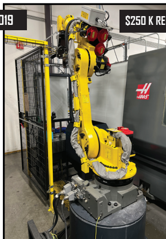
2019 Fanuc Robot R-1000iA/100F Robotic Manipulator, Type A05B-1330-B205 s/n R19320428, Fanuc System R-30iB Plus Touch Screen Controls, Hand Held Controller.
