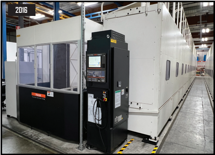
Mazak Pallettech High Rise 31-Station Pallet System w/ Mazatrol Nexus 2 Controls, Mazak PMC-Web System Monitor, (2) Loading Stations, 31 Pallets.
