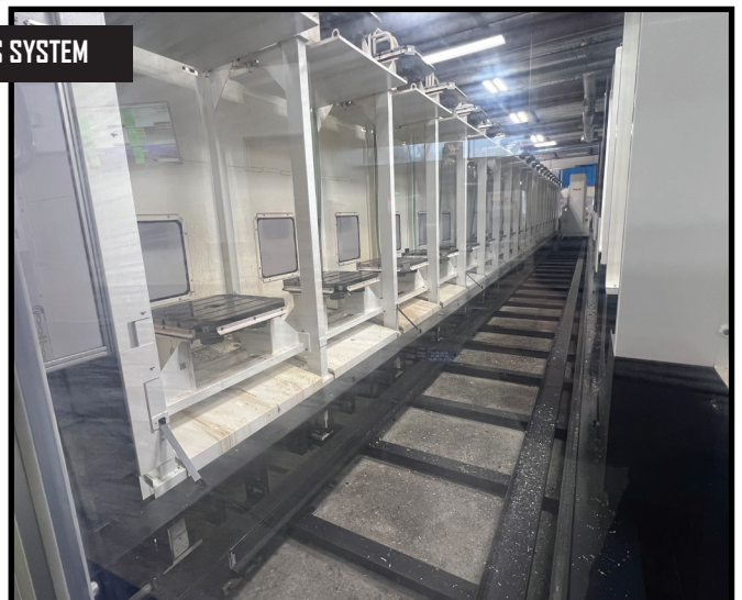
Mazak Pallettech High Rise 39-Station Pallet System w/ Mazatrol Nexus 2 Controls, Mazak PMC-Web System Monitor, (2) Loading Stations, 39 Pallets.
