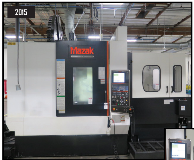
9/2015 Mazak Nexus 530C-II HS 2-Pallet CHC Vertical Machining Center s/n 266170 w/ Mazatrol Matrix Nexus 2 Controls, Hand Wheel, 48-Station ATC, CAT-40 Taper Spindle, 18,000 RPM, Renishaw OTS Wireless Tool Touch Probe, Renishaw Wireless Probing System with CAT-40 Taper Probe Head, Mazak Superflow T8/1000 1000psi Coolant and Filtration System, Oil Cooler, Chip Augers, Chip Conveyor.
