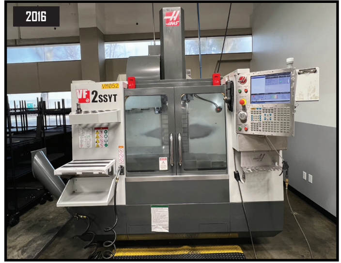
9/2016 Haas VF-2SSYT 4-Axis CNC Vertical Machining Center s/n 1132691 w/ Haas Controls, Hand Wheel, 24-Station ATC, CAT-40 Taper Spindle, 12,000 RPM, Renishaw OTS Wireless Tool Touch Probe, Renishaw Wireless Probing System with CAT-40 Taper Probe, Rigid Tapping, Programmable Coolant Nozzle, Macros, Coordinate Rotation and Scaling, M19 Spindle Orientation, High Speed Machining, VPS Editing, 32GB Memory, Compensation Tables, Chip Auger, Coolant.
