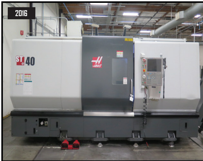
9/2016 Haas ST-40 CNC Machining Center s/n 3106112 w/ Haas Controls, Tool Presetter, 12-Station Turret, Hydraulic Tailstock, 2400 RPM, Rigid Tapping, M19 Spindle Orientation, Quick Code, 15" 3-Jaw Power Chuck, Chip Conveyor, Coolant.
