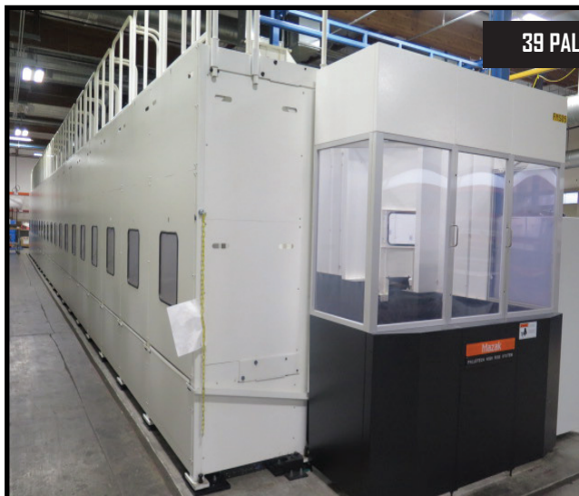
Mazak Pallettech High Rise 39-Station Pallet System w/ Mazatrol Nexus 2 Controls, Mazak PMC-Web System Monitor, (2) Loading Stations, 39 Pallets.
