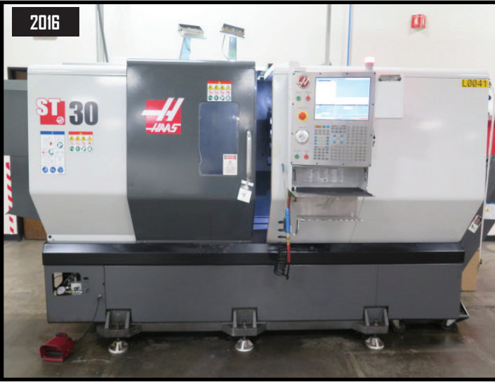
12/2016 Haas ST-30 CNC Turning Center s/n 3106850 w/ Haas Controls, Tool Presetter, 12-Station Turret, 3200 RPM, Rigid Tapping, M19 Spindle Orientation, Quick Code, 12" 3-Jaw Power Chuck, Chip Conveyor, High Flow Coolant.
