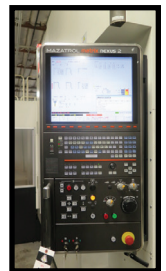
9/2015 Mazak Nexus 8800-II 4-Axis CNC Horizontal Machining Center s/n 265676 w/ Mazatrol Matrix Nexus 2 Controls, Hand Wheel, 240-Station ATC, HSK-100 Spindle, 16,000 RPM, Laser Tool Presetter, Renishaw Wireless Probing System with Probe Head, 4 th Axis Thru Pallets, 31.5" x 31.5" Pallets, Mazak Superflow V8M/1000 1000psi Coolant and Filtration System, Oilmatic Oil Cooler, Chip Augers, Chip Conveyor.
