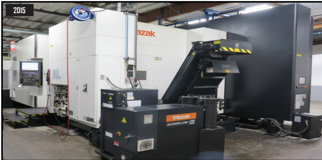
9/2015 Mazak Nexus 8800-II 4-Axis CNC Horizontal Machining Center s/n 265676 w/ Mazatrol Matrix Nexus 2 Controls, Hand Wheel, 240-Station ATC, HSK-100 Spindle, 16,000 RPM, Laser Tool Presetter, Renishaw Wireless Probing System with Probe Head, 4 th Axis Thru Pallets, 31.5" x 31.5" Pallets, Mazak Superflow V8M/1000 1000psi Coolant and Filtration System, Oilmatic Oil Cooler, Chip Augers, Chip Conveyor.
