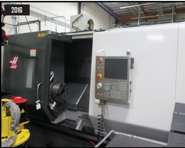
9/2016 Haas ST-40 CNC Robotic Machining Center s/n 3106137 w/ Haas Controls, Tool Presetter, 12-Station Turret, Hydraulic Tailstock, 2400 RPM, Rigid Tapping, M19 Spindle Orientation, Quick Code, 15" 3-Jaw Power Chuck, Chip Conveyor, Coolant
