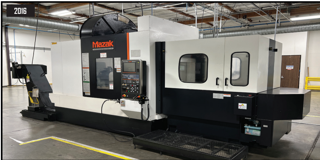
Mazak Nexus 530C-II HS 2-Pallet CHC Vertical Machining Center s/n 273302 w/ Mazatrol Matrix Nexus 2 Controls, Hand Wheel, 48-Station ATC, CAT-40 Taper pindle, 18,000 RPM, Renishaw OTS Wireless Tool Touch Probe, Renishaw Wireless Probing System with CAT-40 Taper Probe Head, Mazak Superflow T8/1000 1000psi Coolant and Filtration System, Oil Cooler, Chip Augers, Chip Conveyor.
