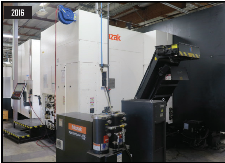
11/2016 Mazak Smooth Tech HCN-8800 4-Axis CNC Horizontal Machining Center s/n 279180 w/ Mazatrol Smooth-G Controls, Digital Hand Wheel, 240-Station ATC, HSK-100 Spindle, 16,000 RPM, Laser Tool Presetter, Renishaw Wireless Probing System with Probe Head, 4 th Axis Thru Pallets, 31.5" x 31.5" Pallets, Mazak Superflow V8M/1000 1000psi Collant and Filtration System, Oilmatic Oil Cooler, Chip Augers, Chip Conveyor.
