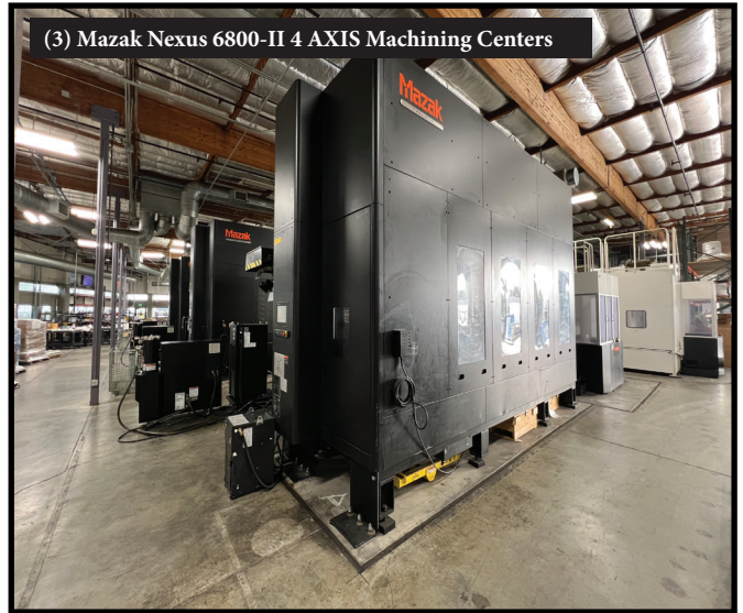
2/2015 Mazak Nexus 6800-II 4-Axis CNC Horizontal Machining Center s/n 261528 w/ Mazatrol Matrix Nexus 2 Controls, Hand Wheel, 240-Station ATC, HSK-100 Spindle, 16,000 RPM Spindle, Laser Tool Presetter, Renishaw Wireless Probing System with Probe Head, 4th Axis Thru Pallets, 24.8" x 24.8" Pallet, Mazak Superflow V8M/1000 1000psi Coolant and Filtration System, Oilmatic Oil Cooler, Chip Augers, Chip Conveyor.
