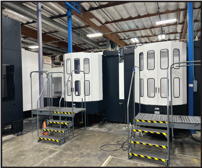
Mazak Pallettech High Rise 31-Station Pallet System w/ Mazatrol Nexus 2 Controls, Mazak PMC-Web System Monitor, (2) Loading Stations, 31 Pallets.
