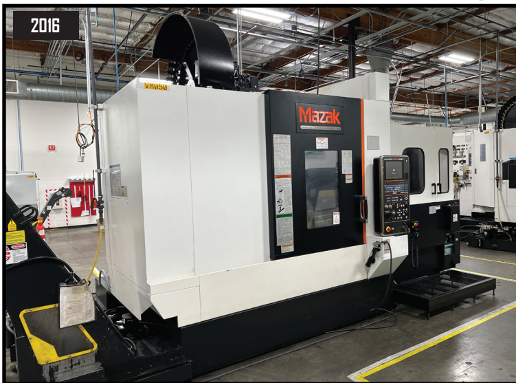
3/2016 Mazak Nexus 530C-II HS 2-Pallet CHC Vertical Machining Center s/n 273222 w/ Mazatrol Matrix Nexus 2 Controls, Hand Wheel, 48-Station ATC, CAT-40 Taper Spindle, 18,000 RPM, Renishaw OTS Wireless Tool Touch Probe, Renishaw Wireless Probing System with CAT-40 Taper Probe Head, Mazak Superflow T8/1000 1000psi Coolant and Filtration System, Oil Cooler, Chip Augers, Chip Conveyor.
