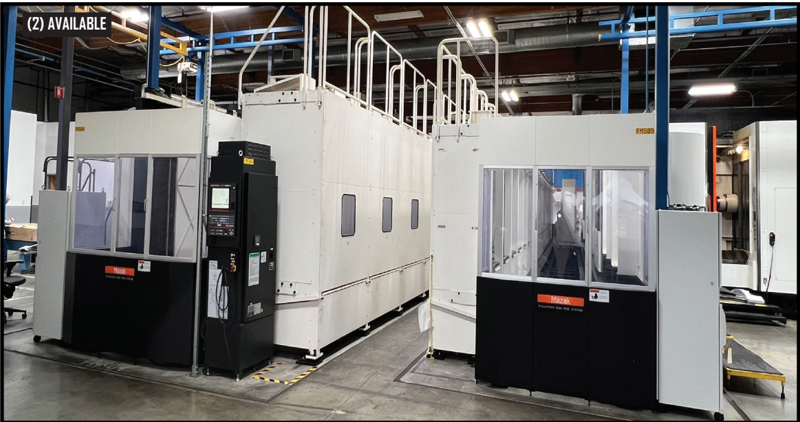
View of (2) Mazak Pallettech High Rise Pallet System for CNC.
