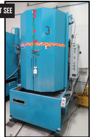
ADF mdl. M860 Heated Rotary Parts Washing System s/n 1410-5754 w/ 40"d x 42"h Basket, Electric Heater, Digital Temp Controller, Wash and Rinse Timers.
