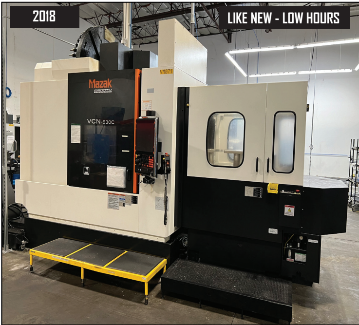
2018 MAZAK VCN 530C CNC VMC WITH PALLET CHANGER, 48 ATC, CAT 40, 41.13" X 20.08" X 20.08 (XYZ), TABLE SIZE 51.18", MEZATROL SMOOTH G CONTROL, MAYFRAM CHIP CONVEYOR, SUPERFLOW V8M-1000 HIGH PRESSURE COOLANT, 12,000 RPM, USED FOR R AND D WITH VERY LOW HOURS, S/N 296516.
