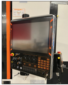
2018 MAZAK VCN 530C CNC VMC WITH PALLET CHANGER, 48 ATC, CAT 40, 41.13" X 20.08" X 20.08 (XYZ), TABLE SIZE 51.18", MEZATROL SMOOTH G CONTROL, MAYFRAM CHIP CONVEYOR, SUPERFLOW V8M-1000 HIGH PRESSURE COOLANT, 12,000 RPM, USED FOR R AND D WITH VERY LOW HOURS, S/N 296516.
