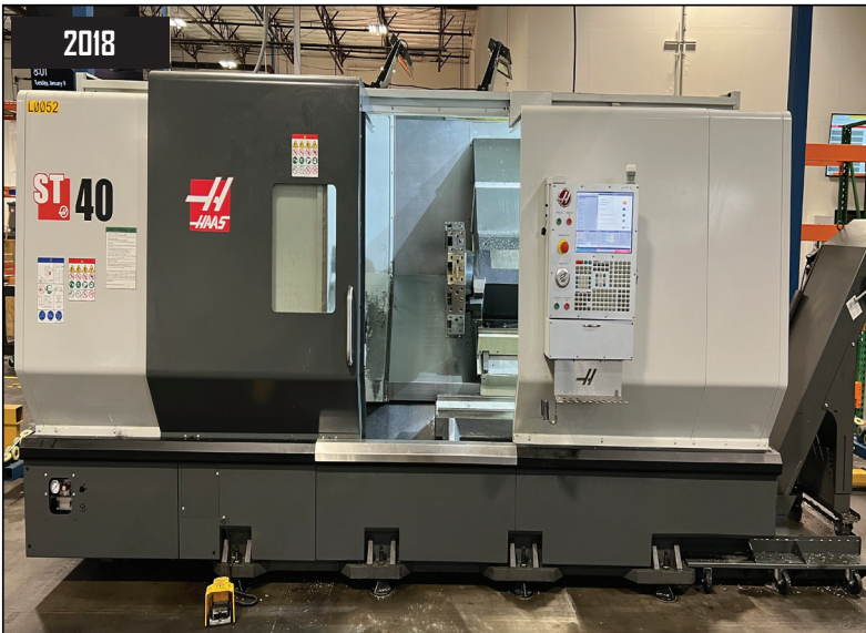
2018 HAAS ST-40 CNC TURNING CENTER, 15" CHUCKS, 34" SWING, 2400 RPM, 44" DISTANCE BETWEEN CENTER, 12 STATION, CHIP CONVEYOR, TAIL STOCK, S/N 3112509.
