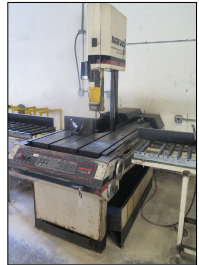
Marvel Series 6 MARK II Vertical Miter Band Saw w/ Marvel Controls
