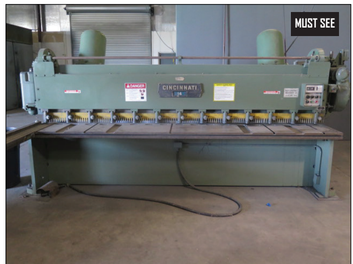
Cincinnati 1412 3/16" x 12' Mechanical Power Shear s/n 34180 w/ Cincinnati Controls and Back Gauging, 152" Squaring Arm.
