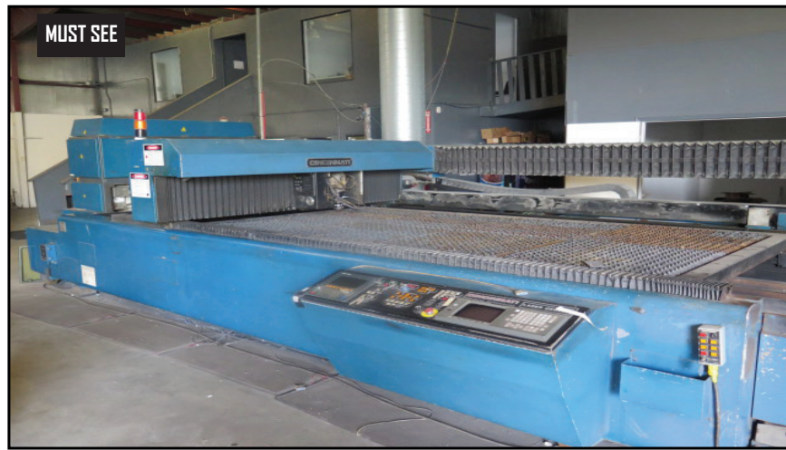
1997 Cincinnati CL-7A 6X12 CNC Laser Center s/n 50301 w/ Fanuc Series 16-M Controls, Dual Shuttle System, Rofin-Sinar 2000 SMX 2000 Watt Laser Source, Koolant Coolers HCV7500-2PR-NF Cooling System.
