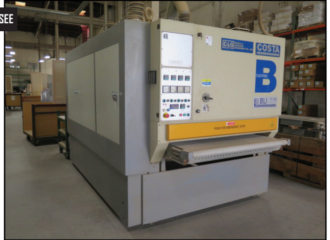
2004 Costa & Grissom BLI 1350 4-Head Cross and Longitudinal 54" Wide Belt Denibbing Sander w/Costa Controls, (2) Cross Brushes, (2) Rotary Brushes
