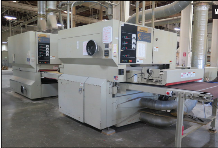
Timesavers 252-71 CBT 7-Head Top and Bottom 52" Wide Belt Sander w/ Timesavers Controls, 3-Head Bottom Sanding, 4-Head Top Sanding
