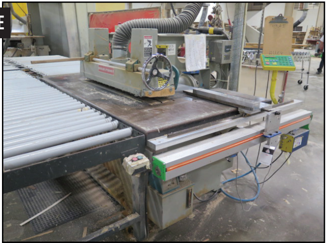
High Point JR-18T 88-1207 Straight Line Rip Saw w/ TigerStop Programmable Fence System
