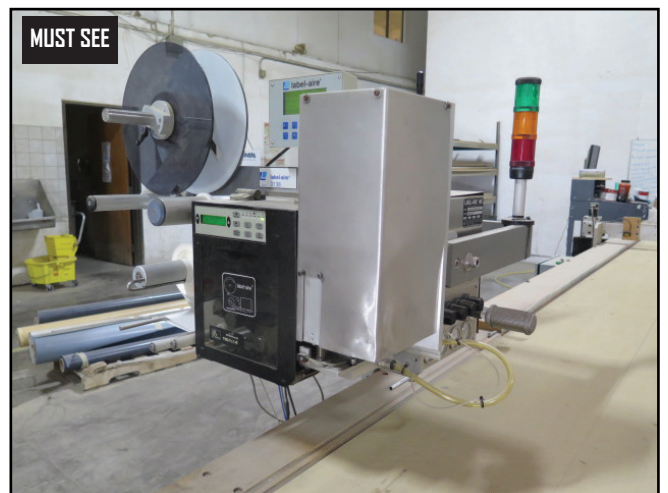
Custom Automatic Parts Labeling System w/ Label-Aire mdl. 3138N-RH STEP TAMP Label Printer / Applicator, Parts Scanner and Conveyors
