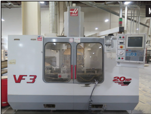
2000 Haas VF-3 CNC VMC w/ Haas Controls, 20-Station ATC, CAT-40 Spindle, 10,000 RPM, Haas Vector Drive
