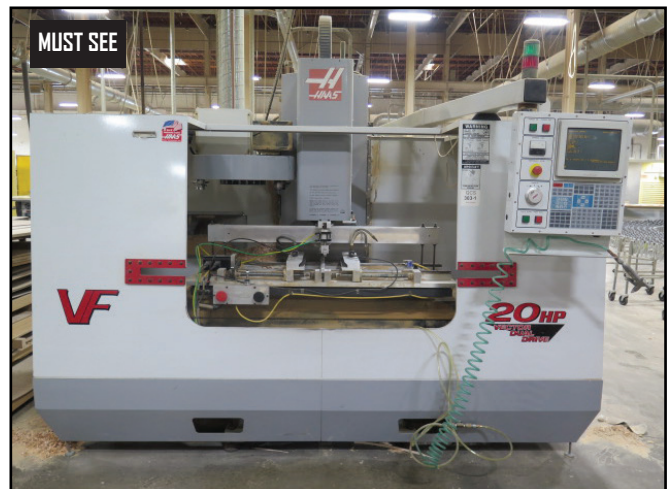
2000 Haas VF-3 CNC VMC w/ Haas Controls, 20-Station ATC, CAT-40 Spindle, 10,000 RPM, Rigid Tapping, 20HP Vector Drive
