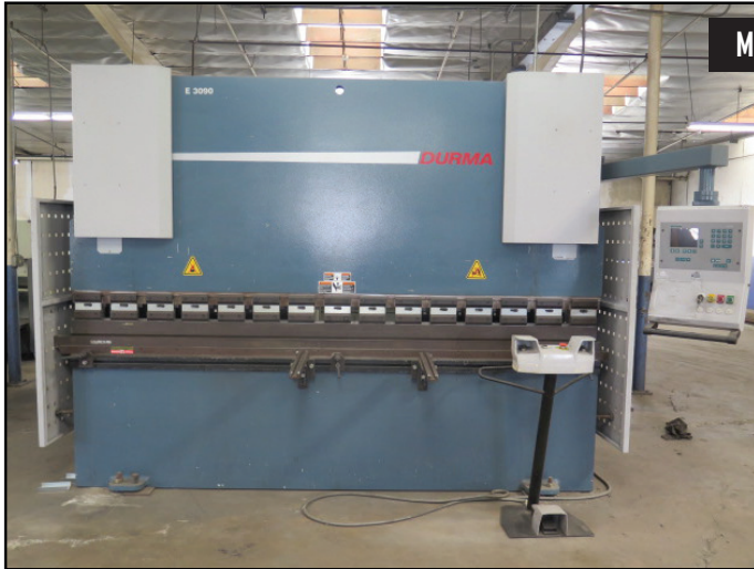
2008 Durma E3090 99 Ton x 10' CNC Hydraulic Press Brake w/ Delem DA-51 Controls and Back Gauging, 6.3" Stroke, 14" Throat, 100.5" Between Uprights
