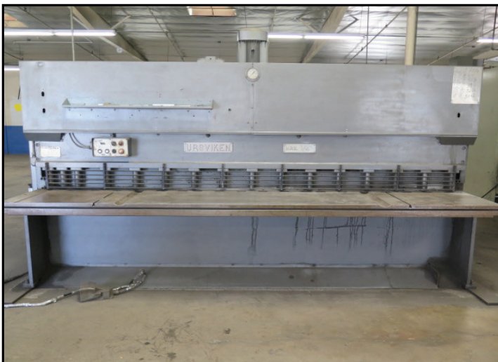
Ursviken type GSD8-6,5/3,5-250 12' x 1/4" Deep Throat Hydraulic Power Shear w/ Controlled Back Gauge, 10 1/2" Throat
