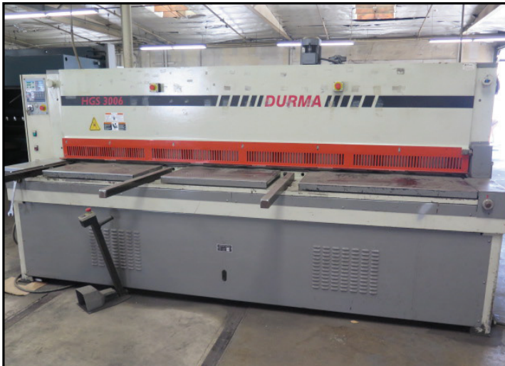
2003 Durma HGS 3006 10' x 0.236" CNC Power Shear w/ Durma ENC 100 Controls and Back Gauge, 42" Squaring Arm, 14 Strokes/Min
