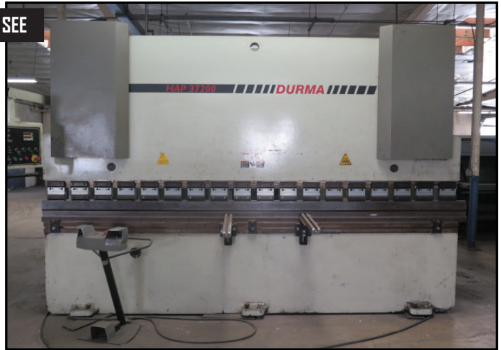
2002 Durma HAP 37200 200 Ton x 12' CNC Hydraulic Press Brake w/ Durma CAD-2-1 Controls and Back Gauging, 7.28" Stroke, 14" Throat, 122" Between Uprights
