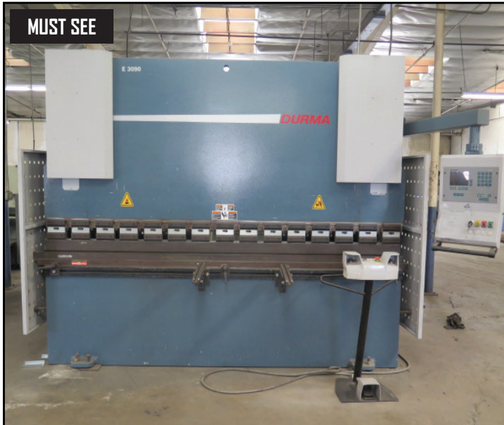
2008 Durma E3090 99 Ton x 10' CNC Hydraulic Press Brake w/ Delem DA-51 Controls and Back Gauging, 6.3" Stroke, 14" Throat, 100.5" Between Uprights
