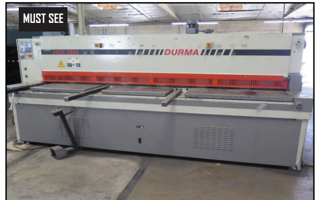
2003 Durma HGS 3006 10' x 0.236" CNC Power Shear w/ Durma ENC 100 Controls and Back Gauge, 42" Squaring Arm, 14 Strokes/Min
