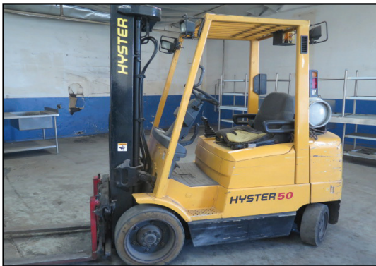
Hyster S50XM LPG Forklift w/ 2-Stage Mast, 130" Lift Height, Side Shift, 4 th Actuator Lever, Cushion Tires, 13,898 Hours
