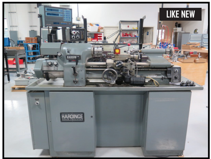
Hardinge HLV-H Wide-Bed Tool Room Lathe w/ Acu-Rite Master-TP DRO, 125-3000 RPM, Inch/mm Threading, Tailstock, Compound Cross Slide, Power Feeds, Change Gears
