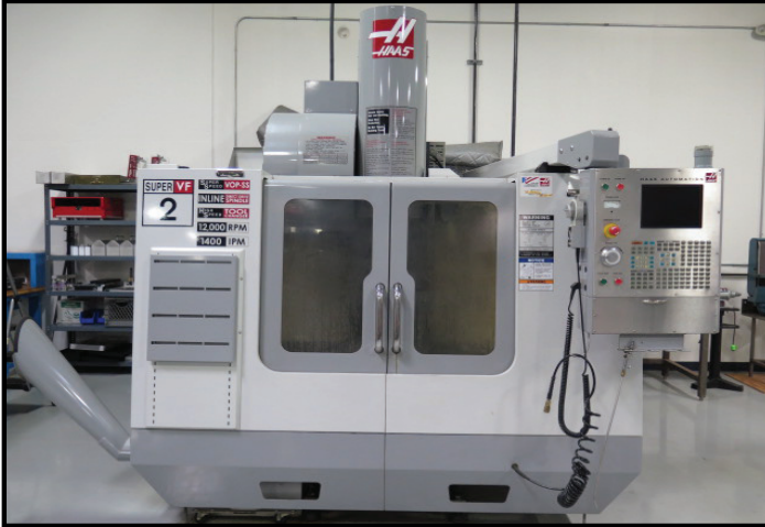
2005 Haas Super VF-2 SS 4-Axis CNC VMC w/ Haas Controls, 24-Station Side Mount ATC, CAT-40 Spindle, 12,000 RPM, Super Speed VOP-SS, Inline Direct Drive Spindle, High Speed Tool Changer
