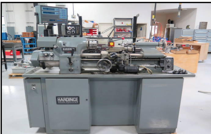
Hardinge HLV-H Wide-Bed Tool Room Lathe w/ Acu-Rite Master-TP DRO, 125-3000 RPM, Inch/mm Threading, Tailstock, Compound Cross Slide, Power Feeds, Change Gears
