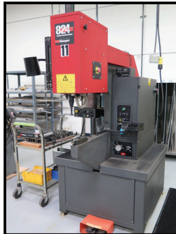
2000 Haeger 824-PLUS-1H 8 Ton x 24" Hardware Insertion Press w/ Haeger Modular Auto Feed System, TPS Tool Protection System, Digital Counters
