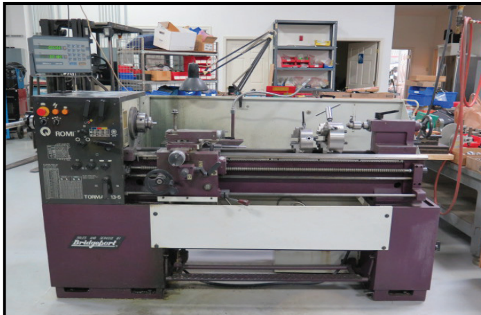
Bridgeport / Romi "Tormax 13-5" Geared Head Lathe w/ Mitutoyo UDR-220 DRO, 80-2500 RPM, Inch/mm Threading, Taper Attachment, Tailstock, Steady Rest, Change Gears
