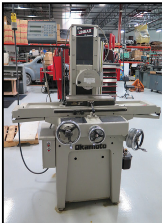
Okamoto "6-18 LINEAR" 6" x 18" Surface Grinder w/ Mitutoyo UDR-220 DRO, Magnetic Chuck
