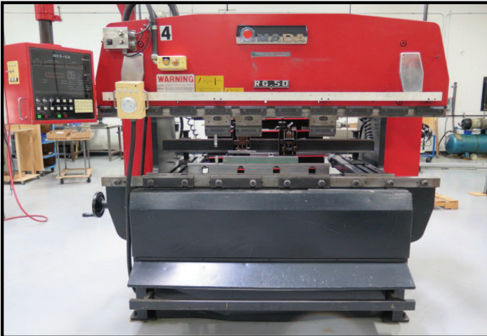
Amada RG-50, 50 Ton x 78" CNC Press Brake w/ NC9-EX Controls, 78.8" Bed, 82.1" Max Bend, 15.75" Throat, 3.94" Stroke, 14.58" Open Height
