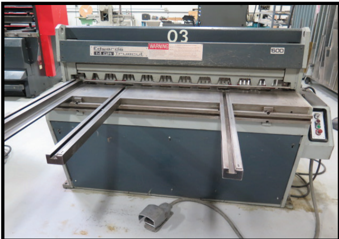
Edwards "14GA Truecut" mdl. 2.5/1250DD 49.5" x 14GA Power Shear w/ Dial Back Gauge, Trava-Dial, 40" Squaring Arm, Front Supports
