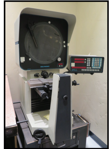
Deltronic DH-214 14" Optical Comparator w/ MPC-5 Programmable DRO, Digital Angular Readout, Shadow Detector, Surface and Profile Illumination
