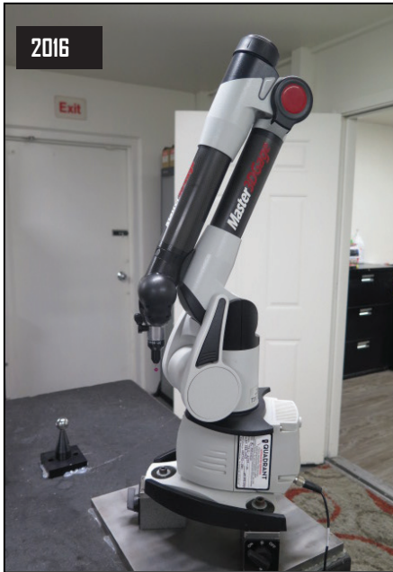
2016 VeriSurfX "Master 3D Gage" Portable CMM Arm w/ 1.2m (4') Measuring Volume, Acces
