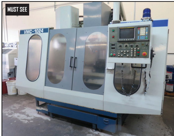
1997 Johnford VMC-1024 CNC VMC w/ Fanuc 0-M Controls, 24-Station ATC, CAT-40 Spindle, 8,000 RPM
