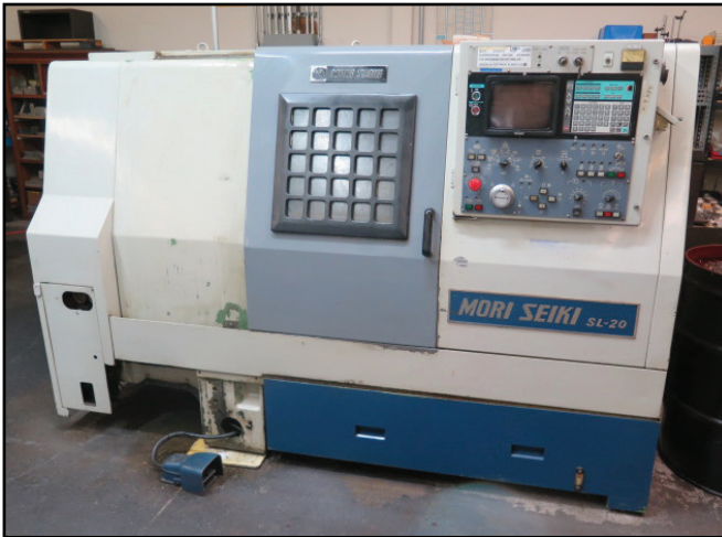
Mori Seiki SL-20 CNC Turning Center w/ Yasnac Controls, 10-Station Turret, Hydraulic Tailstock, 8" 3-Jaw Chuck, 3J Spindle Nose
