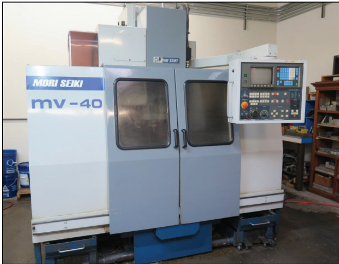
Mori Seiki MV-40 CNC VMC w/ Fanuc Controls, 20-Station ATC, BT-40 Spindle, 8000 RPM
