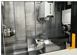
2015 DMG Mori NTX 2000/1500 SZM Multi-Axis Twin Spindle, Live Turret Turning Center s/n NTX21150902 w/ DMG Mori "ERGoline" Controls, (2) 40-Station ATC's (80 Total), CAPTO 6 Spindle, 12,000 4 th Axis Spindle, 5000 RPM on Main and Sub Spindles, 8" 3-Jaw Power Chucks and Royal Products QG-80 Collet Spindle Noses, 10-Station Live Turret, Renishaw Wireless Probing System, Chip Blaster High Pressure Coolant and Filtration System, Mist Collection Systems mdl. JV40 Mist Collector, Chip Conveyor, LNS Quick Load Servo 80 S2 Automatic Bar Loader / Feeder.
