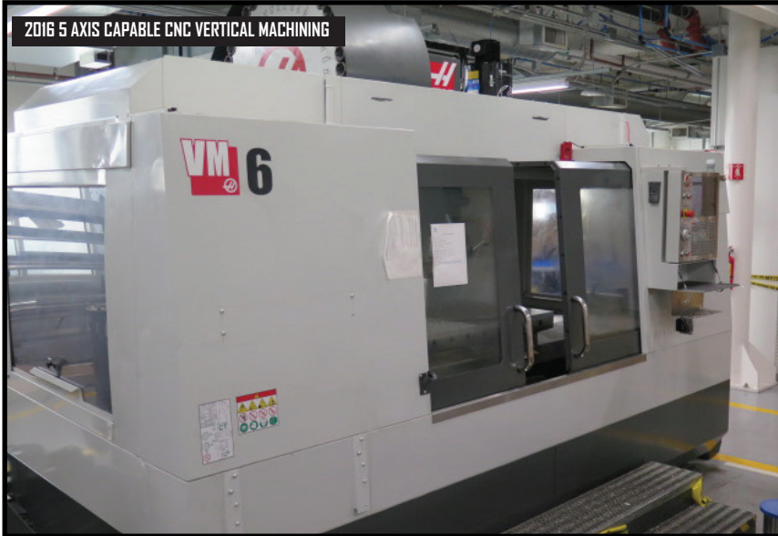
2016 Haas VM-6 5-Axis Capable CNC Vertical Machining Center s/n 1129373 w/ Haas Controls, 40-Station Side Mount ATC, CAT-40 Taper Spindle, Renishaw Wireless Probe System, Renishaw OTS Tool Touch Probe, Programmable Coolant Nozzle, Air Blow, (4) Chip Augers, Chip Conveyor, Coolant
