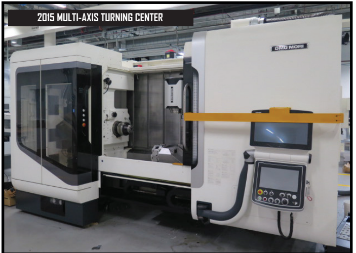
2015 DMG Mori NTX 2000/1500 SZM Multi-Axis Twin Spindle, Live Turret Turning Center s/n NTX21150902 w/ DMG Mori "ERGoline" Controls, (2) 40-Station ATC's (80 Total), CAPTO 6 Spindle, 12,000 4 th Axis Spindle, 5000 RPM on Main and Sub Spindles, 8" 3-Jaw Power Chucks and Royal Products QG-80 Collet Spindle Noses, 10-Station Live Turret, Renishaw Wireless Probing System, Chip Blaster High Pressure Coolant and Filtration System, Mist Collection Systems mdl. JV40 Mist Collector, Chip Conveyor, LNS Quick Load Servo 80 S2 Automatic Bar Loader / Feeder.
