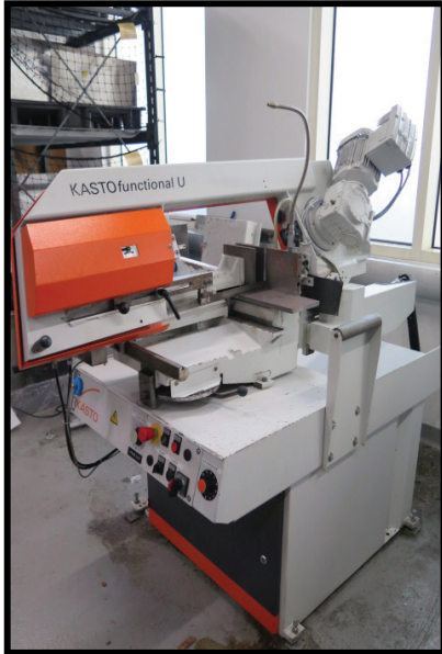
2013 Kasto Type "KASTO functional U" Horizontal Band Saw s/n 6000-109-109 w/ Pneumatic Clamping and Feeds, Coolant Conveyor.
