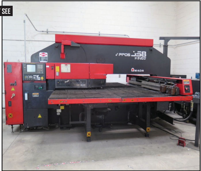
1998 Amada VIPROS 358 King II 30-Ton CNC Turret Punch Press w/ Fanuc Series 18-P Controls, 58-Station Thick Turret, (4) Indexing Positions
