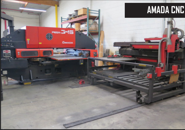
1990 Amada PEGA-345 30-Ton CNC Turret Punch Press s/n AQ450083 w/ Amadan 04P-C Controls, 40-Station Queen Turret, (2) Indexing Positions, Automatic Sheet Repositioner, 39" x 107" Ball-Top Table, Amada MP-1212 NF Automatic Sheet Loader.
