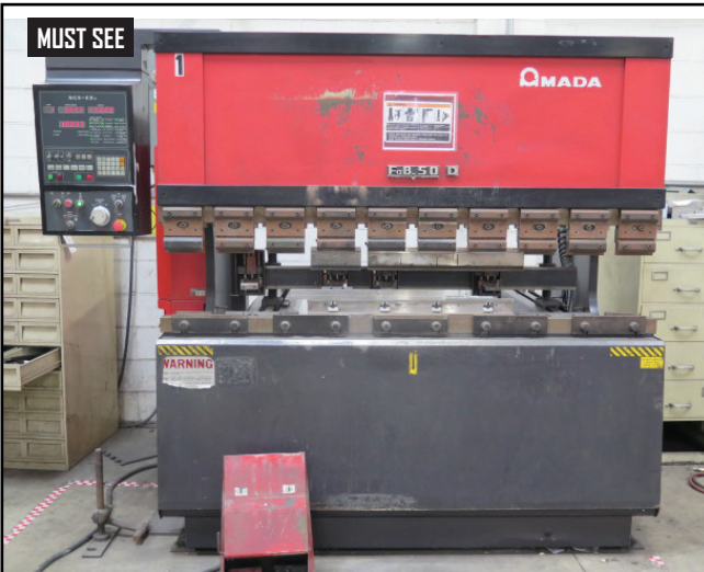
Amada FcxB-50D mdl. FDB-5020E 50-Ton x 78" CNC Press Brake w/ Amada NC9-EX II Controls
