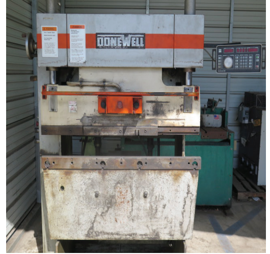
Donewell type 17-1300 17 Ton x 51" CNC Hydraulic Press Brake w/ Autobend 5S Controls
