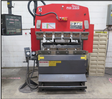
1998 Amada RG-35 35 Ton x 48" CNC Press Brake w/ Amada NC9-EX II Controls
