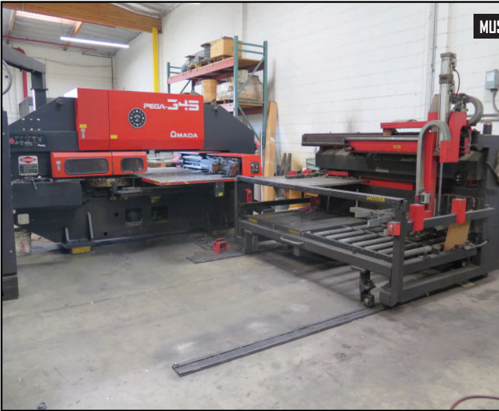
1990 Amada PEGA-345 30-Ton CNC Turret Punch Press s/n AQ450083 w/ Amadan 04P-C Controls, 40-Station Queen Turret, (2) Indexing Positions, Automatic Sheet Repositioner, 39" x 107" Ball-Top Table, Amada MP-1212 NF Automatic Sheet Loader.
