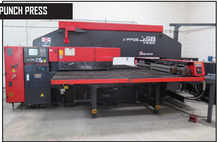
1998 Amada VIPROS 358 King II 30-Ton CNC Turret Punch Press w/ Fanuc Series 18-P Controls, 58-Station Thick Turret, (4) Indexing Positions
