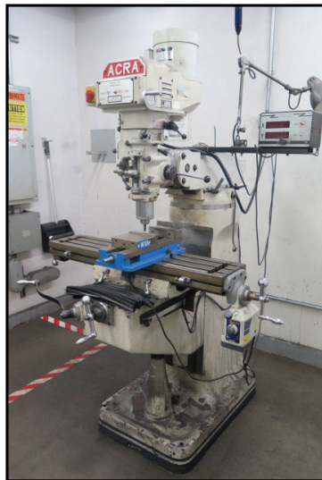
Acra AM-2V Vertical Mill s/n 951456 w/ Sterling DRO, 3Hp Motor, 60-4200 Dial Change Rpm, Chrome Ways, Power Feed, 9" x 42" Table.
