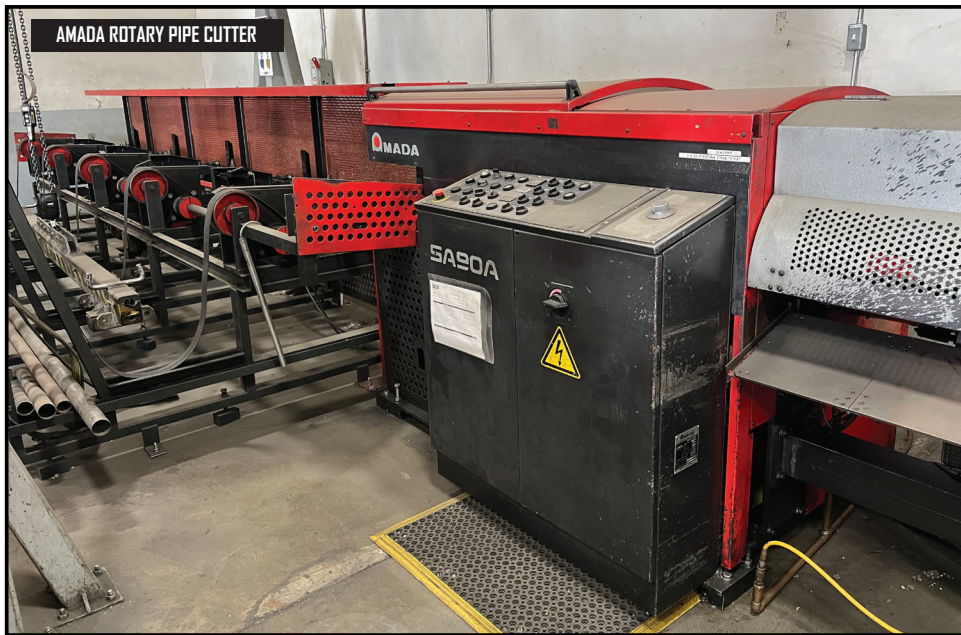
2004 Amada SA90A Rotary Pipe Cutter s/n 90000005 w/ Amada Controls, Automatic Pipe Loader, 1.25"-3.54" x .24" Max Pipe Dia., 137.8"-255.6" Max Pipe Length, 1 1/4", 1 1/2", 1 3/4", 2", 2 1/8", 2 1/4", 2 1/2" and 3" Collet and Liner Sets.
