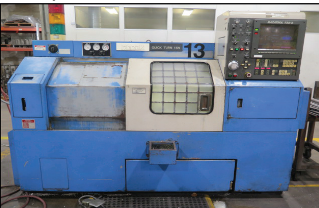
Mazak SQT 15N-U CNC Turning Center s/n 82695 w/ Mazak T32-2 Controls, Tool Presetter, 10-Station Turret, Hydraulic Tailstock, Parts Catcher, 8” 3-Jaw Power Chuck, Coolant.
