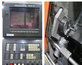
1999 Mazak Super Quick Turn 200MS Live Turret – Twin Spindle CNC Turning Center s/n 139309 w/ Mazatrol 640T PC-FUSION-CNC Controls, Tool Presetter, 12-Station Live Turret (NO TOOLING), 8” 3-Jaw Main Power Chuck, 6” 2-Jaw Sub Spindle Power Chuck, Parts Catcher, Chip Conveyor, Coolant.
