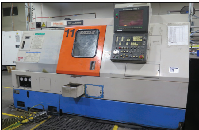
Mazak SQT10MS Live Turret - Twin Spindle CNC Turning Center s/n 106890 w/ Mazak T32-3 Controls, Tool Presetter, 12-Station Turret (NO TOOLING), 6 ½” 3-Jaw Main Spindle Power Chuck, 5” 3-Jaw Sub-Spindle Power Chuck, Parts Catcher, Coolant.
