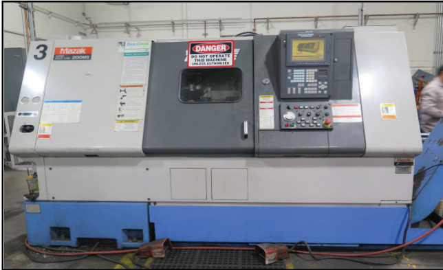
2001 Mazak Super Quick Turn 200MS Live Turret – Twin Spindle CNC Turning Center s/n 152105 w/ Mazatrol 640T PC-FUSION-CNC Controls, Tool Presetter, 12-Station Live Turret (NO TOOLING), 8” 3-Jaw Main Power Chuck, 6” 2-Jaw Sub Spindle Power Chuck, Chip Conveyor, Coolant.
