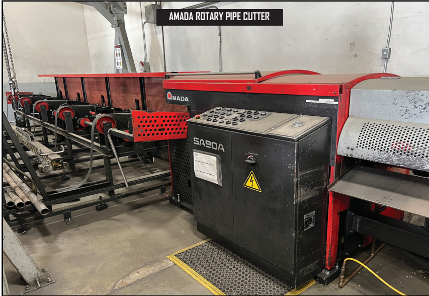
2004 Amada SA90A Rotary Pipe Cutter s/n 90000005 w/ Amada Controls, Automatic Pipe Loader, 1.25"-3.54" x .24" Max Pipe Dia., 137.8"-255.6" Max Pipe Length, 1 ¼", 1 ½", 1 ¾", 2", 2 1/8", 2 ¼", 2 ½" and 3" Collet and Liner Sets.
