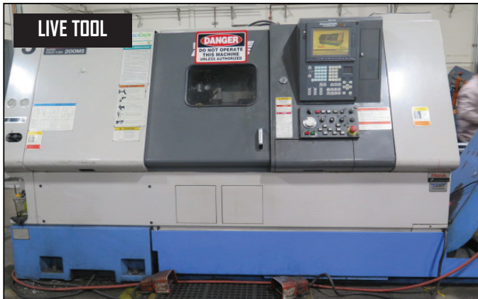
2001 Mazak Super Quick Turn 200MS Live Turret - Twin Spindle CNC Turning Center s/n 152105 w/Mazatrol 640T PC-FUSION-CNC Controls, Tool Presetter, 12-Station Live Turret (NO TOOLING), 8" 3-Jaw Main Power Chuck, 6" 2-Jaw Sub Spindle Power Chuck, Chip Conveyor, Coolant.
