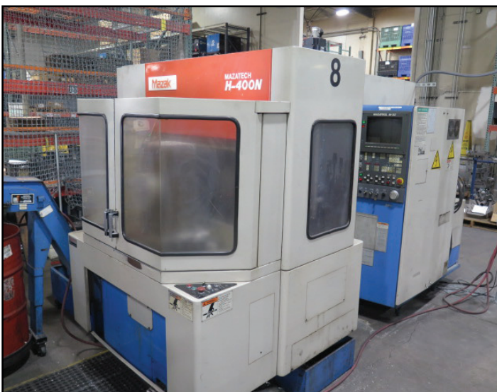
Mazak Mazatech H-400N 2-Pallet 4-Axis CNC Horizontal Machining Center s/n 109392 w/ Mazatrol M-32 Controls, Tool Presetter, 30-Station ATC (NO TOOLING), CAT-40 Taper Spindle, 4 th Axis Thru Pallets @ 1Degree, (2) 15 ¾" x 15 ¾" Pallets, Chip Augers, Chip Conveyor, Coolant.
