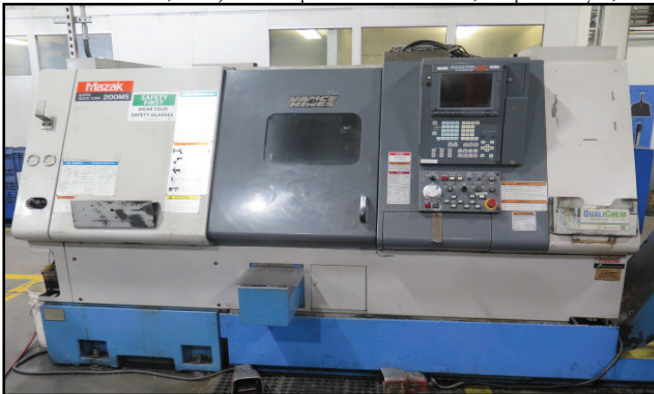
1999 Mazak Super Quick Turn 200MS Live Turret – Twin Spindle CNC Turning Center s/n 139309 w/ Mazatrol 640T PC-FUSION-CNC Controls, Tool Presetter, 12-Station Live Turret (NO TOOLING), 8” 3-Jaw Main Power Chuck, 6” 2-Jaw Sub Spindle Power Chuck, Parts Catcher, Chip Conveyor, Coolant.
