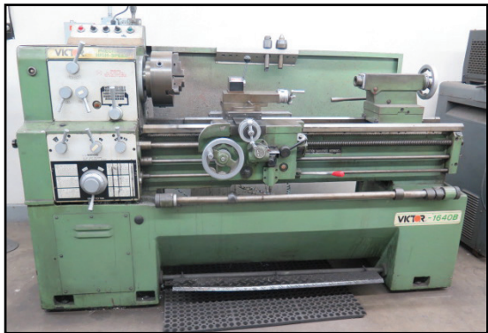
Victor 1640B 16" x 40" Geared Head Gap Bed Lathe s/n 39030572 w/ 55-2000 RPM, Inch/mm Threading, Tailstock, KDK Tool Post, 10" 3-Jaw Chuck.
