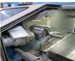
Mazak SQT 15N-U CNC Turning Center s/n 82695 w/ Mazak T32-2 Controls, Tool Presetter, 10-Station Turret, Hydraulic Tailstock, Parts Catcher, 8” 3-Jaw Power Chuck, Coolant.
