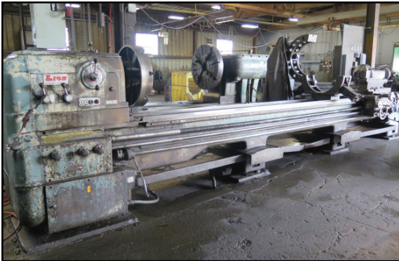
Lion C13/MB 32" x 230" Geared Head Lathe s/n 13MH-5000-80039 w/ 6-1000 RPM, Inch/mm Threading, Tailstock, Steady Rest, 4" Thru Spindle Bore, Aloris Tool Post, 24" 4-Jaw Chuck.
