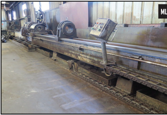
LeBlond Model 4GSR-10A-242-S Treepan Lathe w/ 43.5-210 RPM, 2"-10" ID Cap, 24" Max OD, 30" Travel Depth, 28" 4-Jaw Chuck, Hollow Steady Rests, Coolant.
