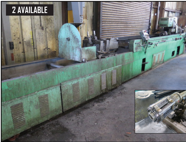
(2) Custom Built Horizontal Honing Machines w/ 20' Power Stroke, 1.5" to 16" Hone Cap, Coolant.
