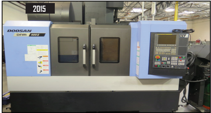
2015 2015 Doosan DNM400 II 5-Axis Capable CNC VMC w/ Fanuc I Series Controls, 30-Side Mount ATC, CAT-40, 12,000 RPM, Thru Spindle Coolant, Rigid, Renishaw Probe System
