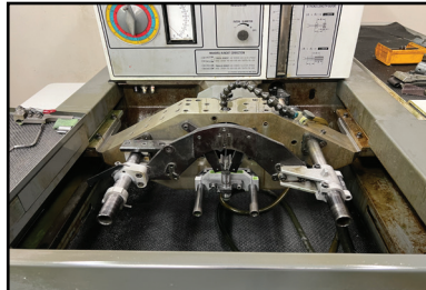
4 SUNNEN HONE ML-2000-DF HONING MACHINE W/ STROKER, 6.7" STROKE, VARIABLE STROKE RATE.
