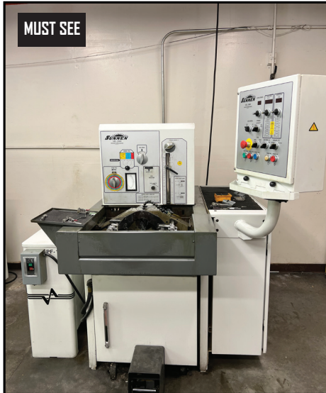
4 SUNNEN HONE ML-2000-DF HONING MACHINE W/ STROKER, 6.7" STROKE, VARIABLE STROKE RATE.
