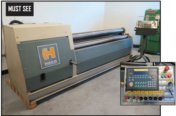
Atlantic / HACO mdl. 4HBR206P 80" 4-Roll CNC Plate Roll w/ Elap-Lynx Controls
