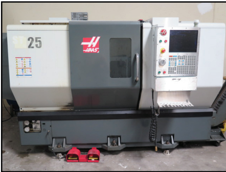
2014 Haas ST-25 CNC Turning Center w/ Haas Controls, Tool Presetter, 12-Station Turret, Hydraulic Tailstock, 4000 RPM, Rigid Tapping, 10" 3-Jaw Chuck
