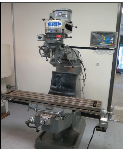
Rutland Vertical Mill w/ Delos DS-2M DRO, 2Hp, 80-5440
