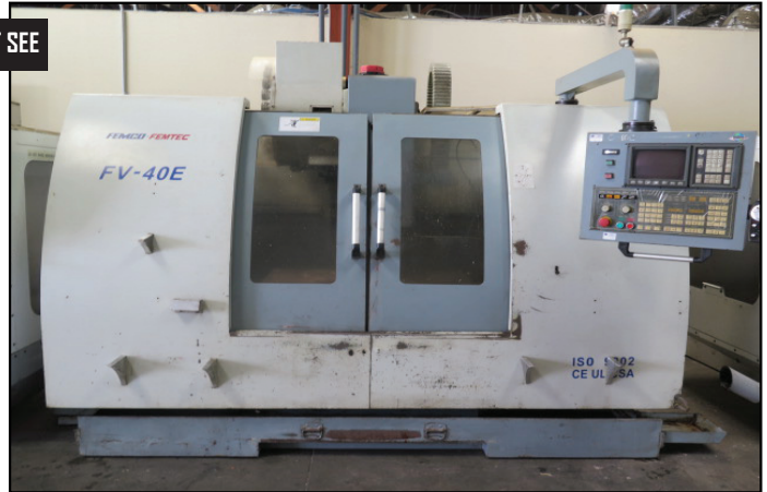
2002 Femco – Femtec FV-40E CNC VMC w/ Fanuc 0-MC Controls, 24-Station Side-Mount ATC, 40-Taper Spindle, 23 ½” x 47” Table
