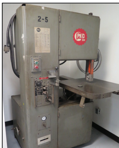
Grob 4V-18 18" Vertical Band Saw w/ Blade Welder
