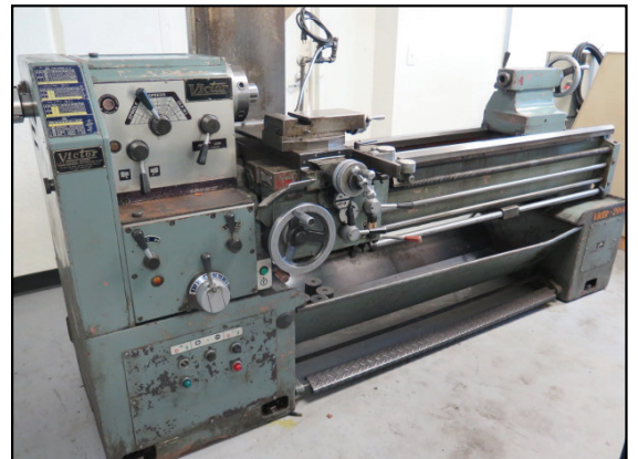
Victor 2060 20" x 60" Geared Head Gap Bed Lathe
