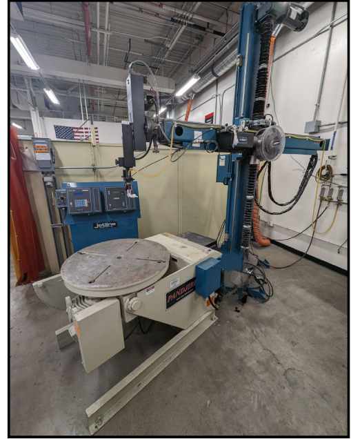
Pandjiris 30-6AB 3000 Lb Cap 30" Motorized Welding Positioner
