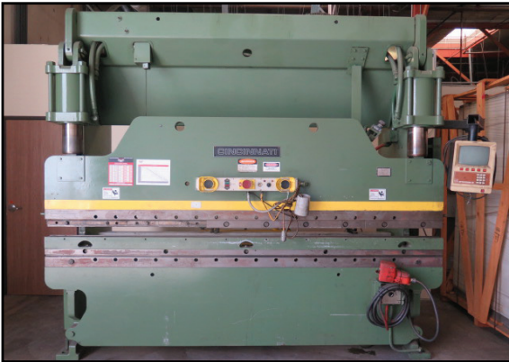
Cincinnati 135CBx8FT 135 Ton x 10' CNC Hydraulic Press Brake w/ Dynabend III Controls, 10' Bed Length, 7" Throat, 8" Stroke
