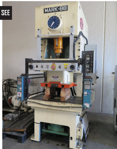
Heller Southerland "MARK 88" 88 Ton Hydraulic Press w/ Southerland Controls, 3.9" Stroke, 55-100 Strokes/Min
