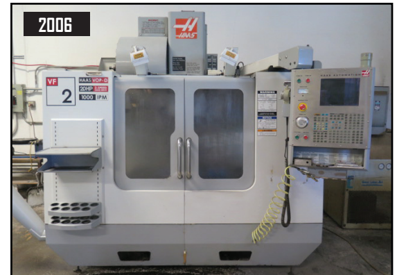
2006 Haas VF-ZB 4-Axis CNC VMC w/ Haas Controls, 24-Side-Mount ATC, CAT-40, 7500 RPM. 20Hp Z-Speed Gear Drive, Haas VOP-D, Rigid Tapping, M19 Spindle Orientation, Coordinate Scaling
