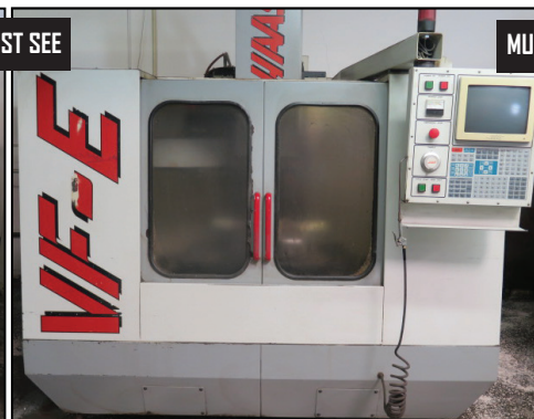
1996 Haas VF-E CNC VMC w/ Haas Controls, Z0-ATC, CAT-40, 7500 RPM
