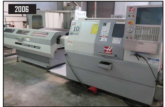
2006 Haas SL-10 CNC Turning Center w/ Tool Presetter, 12-Station Turret, 6000 RPM, Parts Catcher, Rigid Tapping, Servobar 300 Automatic Bar Feeder
