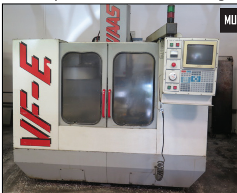
1996 Haas VF-E CNC VMC w/ Haas Controls, Z0-ATC, CAT-40, 7500 RPM 8mm Pitch Ball Screws
