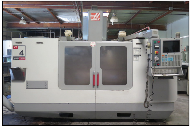
2002 Haas VF-4B CNC VMC w/ Haas Controls, Z0 ATC, CAT-40, 7500 RPM, Rigid Tapping, 20Hp Z-Speed Gear Drive, Programmable Coolant, No Counterbalance, 8mm Pitch Ball Screws
