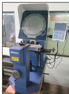
Mitutoyo PH-A14 14" Optical Comparator w/ QM-DATA200 DRO, Surface and Profile Illumination
