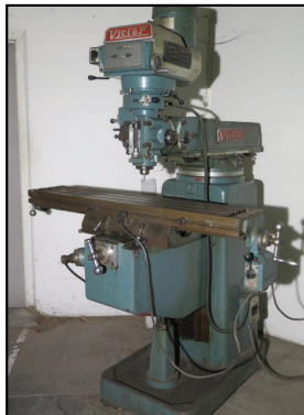
Victor mdl. VICTOR-330V Vertical Mill w/ 3Hp Motor, 60-4200 RPM, Chrome Ways, Power Feed, 10" x 50"
