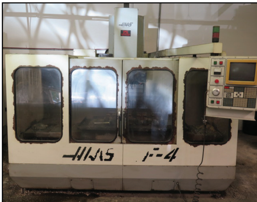
1994 Haas VF-4 CNC VMC w/ Haas Controls, Z0-ATC, CAT-40, 7500 RPM, Rigid Tapping, 15Hp High Torque Motor, Programmable Coolant
