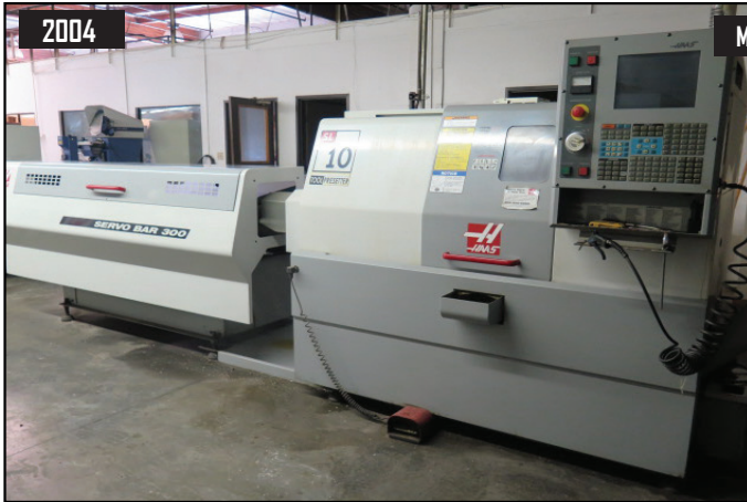
2004 Haas SL-10 CNC Turning Center w/ Haas Controls, Tool Presetter, 12-Station Turret, 6000 RPM, Parts Catcher, Rigid Tapping, Servobar 300 Automatic Bar Feeder
