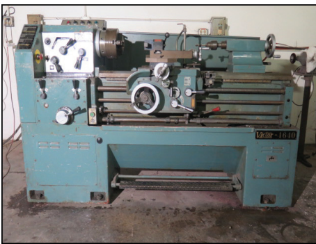
Victor 1640G 16" x 40" Geared Head Gap Bed Lathe w/ 30-1800 RPM, Inch/mm Threading, Tailstock, Trava Dial
