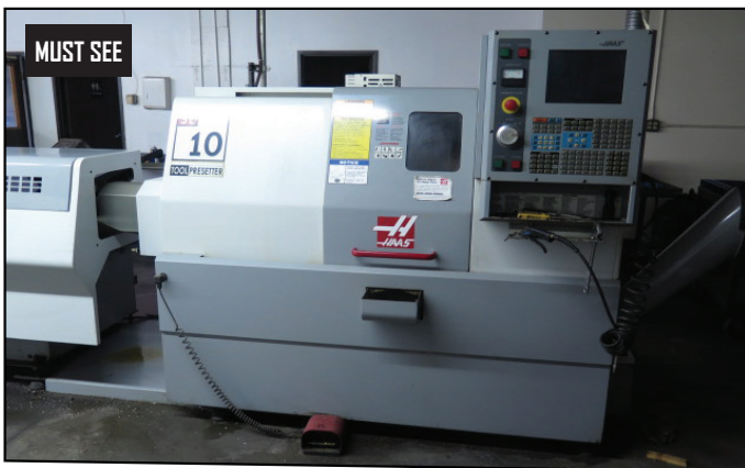
2004 Haas SL-10 CNC Turning Center w/ Haas Controls, Tool Presetter, 12-Station Turret, 6000 RPM, Parts Catcher, Rigid Tapping, M19 Spindle Orientation, Quick Code, 5C
