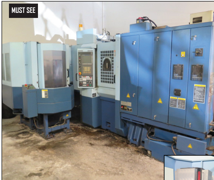
2006 Matsuura H-PLUS-300 11-Pallet CNC HMC w/ G-Tech 30i Controls, Tool Presetter (Needs Cable Repair), 180-Station ATC, CAT-40, 15,000 RPM, 4th Axis @ 1 Degree, Turbo Chip Conveyor
