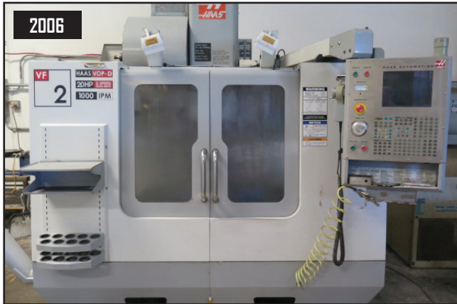
2006 Haas VF-2B 4-Axis CNC VMC w/ Haas Controls, Z4-Side-Mount ATC, CAT-40, 7500 RPM. 20Hp Z-Speed Gear Drive, Haas VOP-D, Rigid Tapping, M19 Spindle Orientation, Coordinate Scaling
