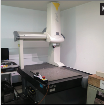
2005 Brown & Sharpe Global Status-5.7.5 CMM Machine w/ Renishaw MH-8 Probe Head, Joystick Controller, PC-DMIS Software
