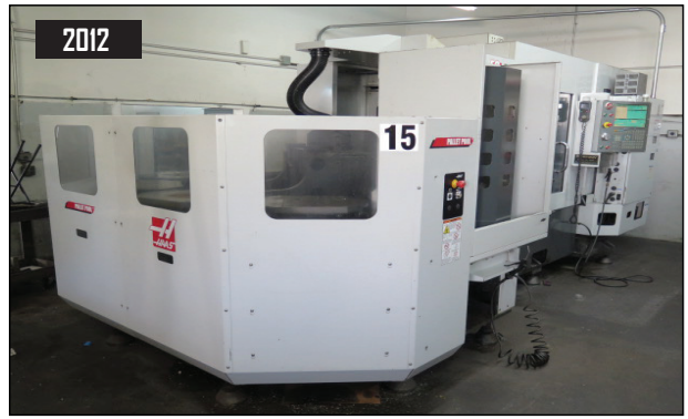
2012 2012 Haas EC-400PP 6-Pallet "Pallet Pool" CNC HMC w/ 70-ATC, CAT-40, 12,000 RPM, Renishaw Tool Presetter, Intuitive Probing System, Full 4 th Axis, Rigid Tapping, Programmable Coolant
