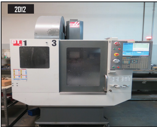
2012 2012 Haas DT-1 CNC VMC w/ 20-ATC, CAT-40, 12,000 RPM, Advanced Tool Management, Programmable Coolant, Rigid Tapping
