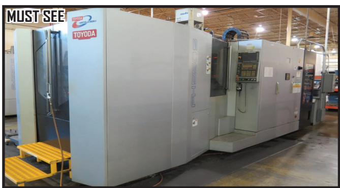
2004 Toyoda FH550S 2-Pallet 4-Axis CNC HMC's w/ Fanuc 30i-Model A Controls, 60-ATC, CAT-50, Laser Presetter, Wireless Probe System, 12,000 RPM, 4 th Axis @ .001 Degrees
