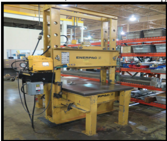
Enerpac 100 Ton Roller Frame Hydraulic Press w/ Enerpac E5 Z-Class Hydraulic Unit
