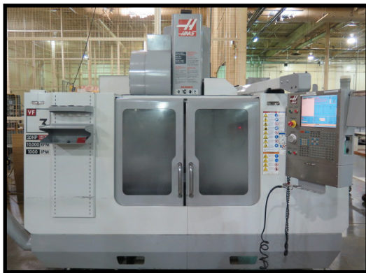
2008 Haas VF-3D 4-Axis CNC VMC w/ 24-Station Side Mount ATC, CAT-40, 10,000 RPM, Renishaw Presetter and Probe, High Speed Machining, Brushless 4 th Axis, Rigid Tapping, Lincoln Spindle Motor, 8mm Pitch Ball Screws
