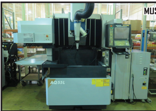
MUST SEE 2006 Sodick AQ55L Die-Sinker EDM Machine w/ LQ1 Controls, Hand Controller, System 3R Head, 32-Station ATC, Sodick 40B Power Source
