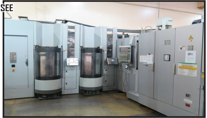
2007 Toyoda 24-Pallet Machining Cell w/ (2) 2007 Toyoda FH450S 2-Pallet 4-Axis CNC HMC's, Pal-Tek FPA-450 24-Pallet Two Level Automatic Pallet Changer Cell
