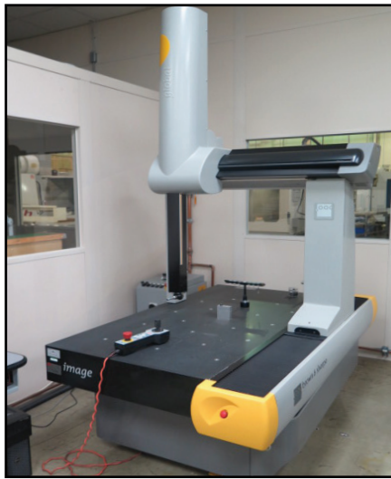
Brown & Sharpe "Global Image 7.10.7" CMM w/ PC-DMIS 2014, Renishaw PH10MQ Probe, MCR20 6-Tip Changer, Joystick Controller, PHC10-2 Probe Controller
