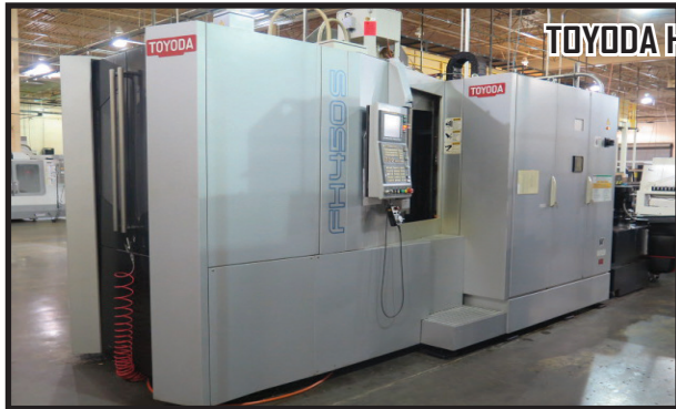
2007 Toyoda FH450S 2-Pallet 4-Axis CNC HMC's w/ Fanuc 31i-Model A Controls, 60-ATC, CAT-40, 15,000 RPM, Tool Presetter, Wireless Probe System, Full 4 th Axis, Thru Spindle Coolant
