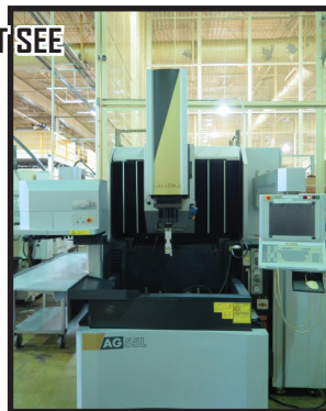
2006 Sodick AQ55L Die-Sinker EDM Machine w/ LQ1 Controls, Hand Controller, System 3R Head, 32-Station ATC, Sodick 40B Power Source
