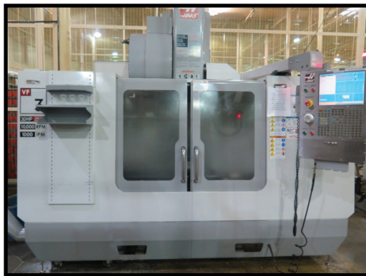
2008 Haas VF-3D 4-Axis CNC VMC w/ 24-Station Side Mount ATC, CAT-40, 10,000 RPM, Renishaw Presetter and Probe, High Speed Machining, Brushless 4 th Axis, Rigid Tapping, Lin
