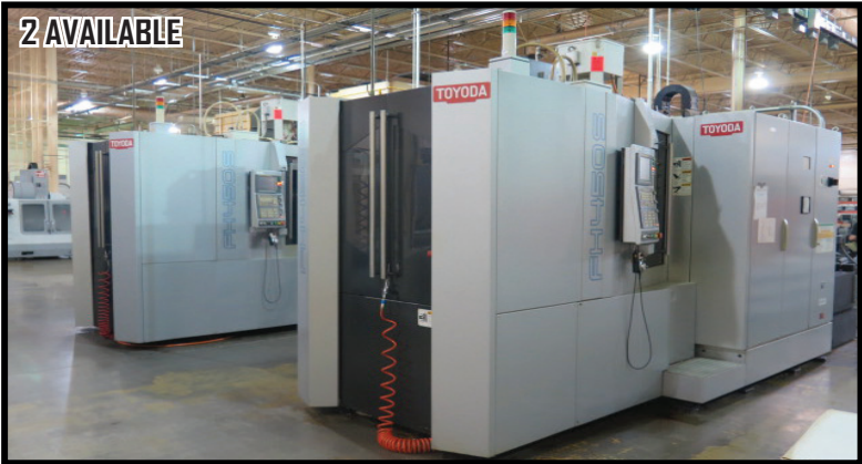
2 AVAILABLE Toyota FH450S 2-Pallet 4-Axis CNC HMC's w/ Fanuc 31i-Model A Controls, 60-ATC, CAT-40,15,000 RPM Full 4th Axis
