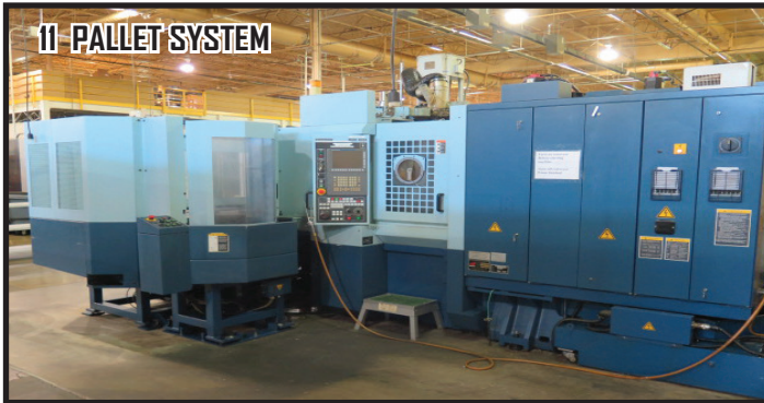
11 PALLET SYSTEM 2006 Matsuura H.Plus-300 PCII 11-Pallet CNC HMC w/ G-Tech 30i Controls, 120-ATC, CAT-40, Laser Presetter, Wireless Probe System, 15,000 RPM, Full 4 th Axis, Thru Spindle Coolant
