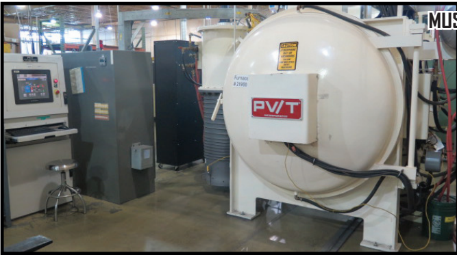
(2) 2008 PV/T 1200 Degree Vacuum Aluminum Brazing Furnace w/ PV/T Touch Screen Controls, 36" x 36" x 60" Work Zone
