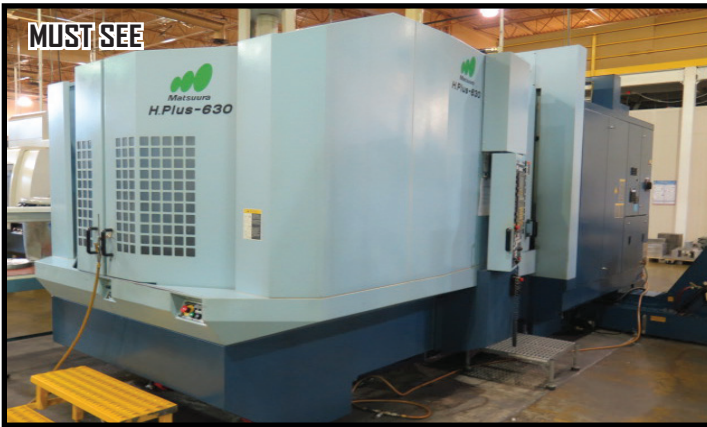
MUST SEE 2005 Matsuura H.Plus-630 2-Pallet 4-Axis CNC HMC w/ G-Tech 30i Controls, 60-ATC, CAT-50, Laser Presetter, Wireless Probe System, Full 4 th Axis, Thru-Spindle Coolant
