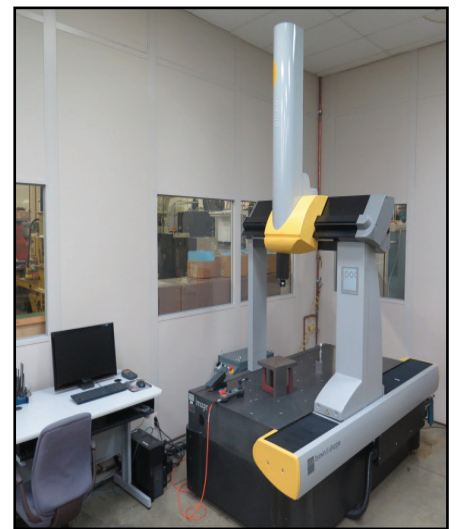
Brown & Sharpe "Global Image 9.15.8" CMM w/ PC-DMIS 2014, Renishaw PH10MQ Probe, MCR20 6-Tip Changer, Joystick Controller, PHC10-2 Probe Controller
