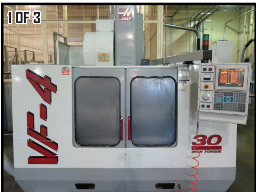
Haas VF-4 CNC VMC w/ 24-Station Side Mount ATC, CAT-40, 10,000 RPM, 30Hp High Torque Option, Rigid Tapping, Sigma Motors X-Y-Z, Programmable Coolant
