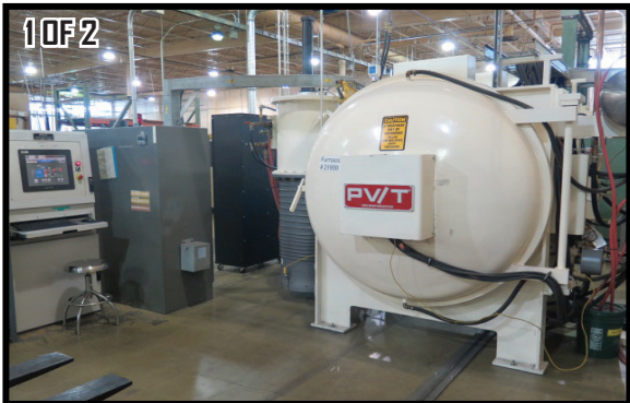
1 OF 2 2008 PV/T 1200 Degree Vacuum Aluminum Brazing Furnace w/ PV/T Touch Screen Controls, 36"x36" x 60" Work Zone
