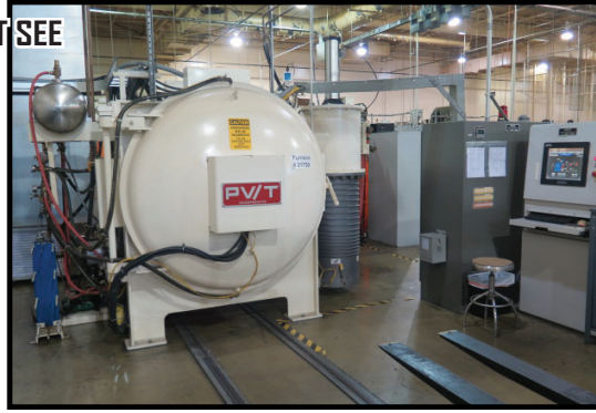
(2) 2008 PV/T 1200 Degree Vacuum Aluminum Brazing Furnace w/ PV/T Touch Screen Controls, 36" x 36" x 60" Work Zone
