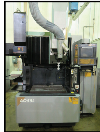
2002 Sodick AQ55L CNC Wire EDM Machine w/ LN1 Controls, Hand Controller, Travels X=29.53",
