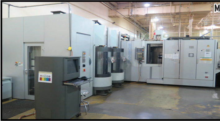
2007 Toyoda 24-Pallet Machining Cell w/ (2) 2007 Toyoda FH450S 2-Pallet 4-Axis CNC HMC's, Pal-Tek FPA-450 24-Pallet Two Level Automatic Pallet Changer Cell
