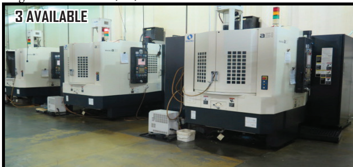
3 AVAILABLE Makino a51 2-Pallet 4-Axis CNC HMC's w/ "Professional 5" Controls, 60-ATC, CAT-40, 0.001 Degree Full 4 th Axis, 12,000 RPM **3-AVAILABLE**
