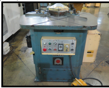
Amada CS-220 8 5/8" x 8 5/8" Hydraulic Corner Notcher
