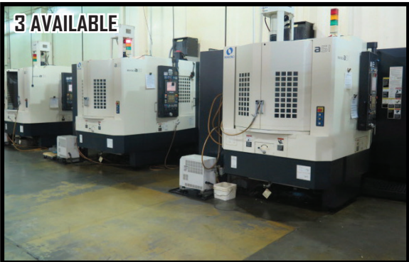
3 AVAILABLE Makino a51 2-Pallet 4-Axis CNC HMC's w/ "Professional 5" Controls, 60-ATC, CAT-40,0.001 Degree Full 4th Axis, 12,000 RPM **3-AVAILABLE**
