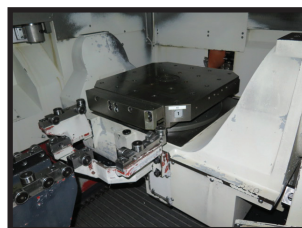
MUST SEE 2004 Mazak Variaxis 630-5X 5-Axis 2-Pallet CNC VMC w/ Mazatrol 640M 5X Controls, Tool Presetter, (2) 40-Station Tool Magazines, 80 Total ATC, CAT-40, 12,000 RPM, Trunnion Style 5 th Axis @ -120 Deg to +30 Deg, Pallet 4 th Axis 360 @ 0.001 Deg, w/ Renishaw Probe
