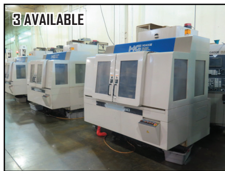
Hitachi Seiki HG400 III 2-Pallet 4-Axis CNC HMC's w/ Seicos Σ16M Controls, 60-ATC, CAT-40, 12,000
