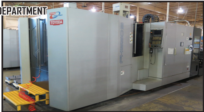
2005 Toyoda FH550S 2-Pallet 4-Axis CNC HMC's w/ Fanuc 30i-Model A Controls, 60-ATC, CAT-50, Laser Presetter, Wireless Probe System, 12,000 RPM, 4 th Axis @ .001 Degrees
