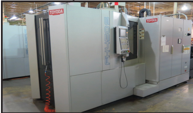
2007 Toyoda FH450S 2-Pallet 4-Axis CNC HMC's w/ Fanuc 31i-Model A Controls, 60-ATC, CAT-40, 15,000 RPM, Tool Presetter, Wireless Probe System, Full 4 th Axis, Thru Spindle Coolant
