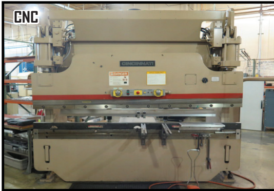
Cincinnati 90 CB II X8FT 90 Ton x 10' CNC Press Brake w/ Cincinnati Controls, 10' Bed
