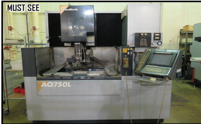
MUST SEE 2002 Sodick AQ750L CNC Wire EDM Machine w/ LN1 Controls, Hand Controller, Travels X=29.53", Y=19.68", Z=15.75", +30 Degree Taper Angle, Wire Chopper
