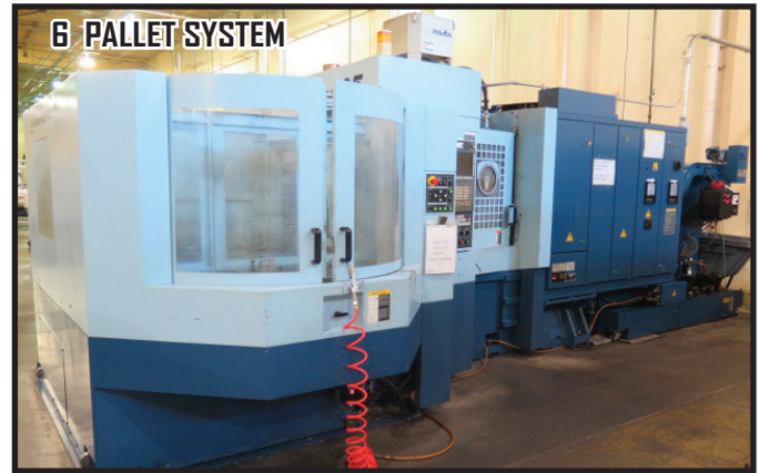
6 PALLET SYSTEM 2005 Matsuura H.Plus-405 6-Pallet CNC HMC w/ G-Tech 30i Controls, 90-ATC, CAT-40, Laser Tool Presetter, Wireless Probe System, 12,000 RPM, Thru-Spindle Coolant, Full 4 th Axis
