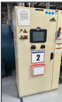
2001 SPALLINGER 5FT X 20FT AUTOCLAVE, REFURBISHED, TOUCH PAD CONTROLS, MAX ALLOWABLE WORKING PRESSURE 125 PSI AT 350 F, MINIMUM DESIGN MATERIAL TEMPERATURE 40 F AT 125 PSI, S/N 01-0960.
