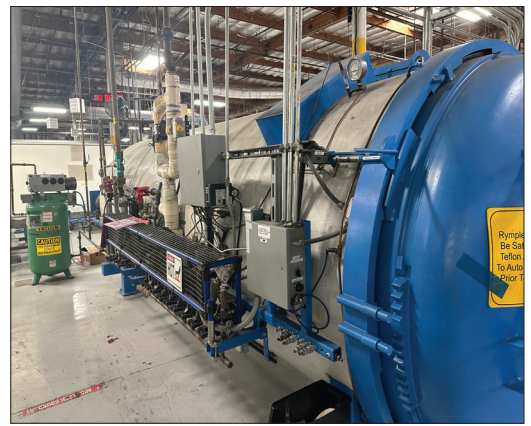
2002 SPALLINGER 5FT X 20FT AUTOCLAVE, REFURBISHED, TOUCH PAD CONTROLS, MAX ALLOWABLE WORKING PRESSURE 125 PSI AT 450 F, MINIMUM DESIGN MATERIAL TEMPERATURE 40F AT 125 PSI, S/N 02-0832.
