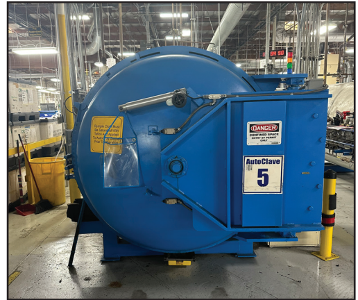
2004 SPALLINGER 6FT X 20FT AUTOCLAVE, REFURBISHED, TOUCH PAD CONTROLS, MAX ALLOWABLE WORKING PRESSURE 125 PSI AT 450 F, MINIMUM DESIGN MATERIAL TEMPERATURE 40 F AT 125 PSI, S/N 04-0258.
