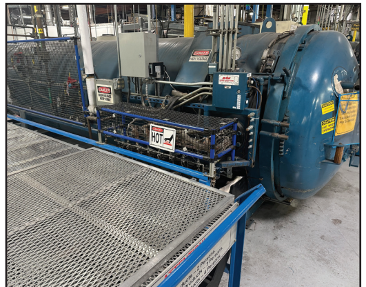
2002 SPALLINGER 5FT X 20FT AUTOCLAVE, REFURBISHED, TOUCH PAD CONTROLS, MAX ALLOWABLE WORKING PRESSURE 125 PSI AT 450 F, MINIMUM DESIGN MATERIAL TEMPERATURE 40F AT 125 PSI, S/N 02-0832.
