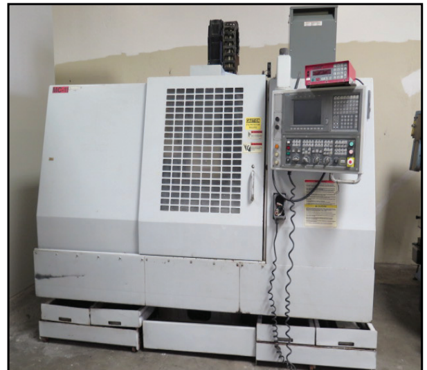
Okuma CadetMate CNC VMC w/ OSP700M Controls, 20-Station ATC, 40-Taper Spindle 6128 2016 Doosan DNM 5700 4-Axis CNC VMC w/ Fanuc iSeries Controls, "Easy Operation Package", 30-Station ATC, 40-Taper Spindle
