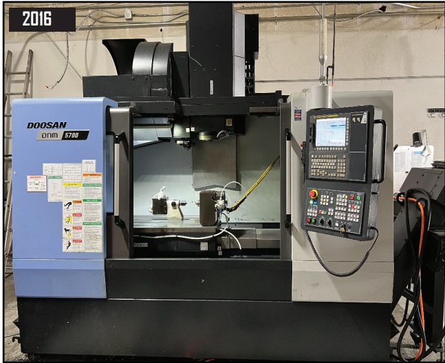
2016 Doosan DNM 5700 4-Axis CNC Vertical Machining Center s/n MV0091-000413 w/ Doosan-Fanuc iSeries Controls, Hand Wheel, "Easy Operation Package", 30-Station ATC, 40-Taper Spindle
