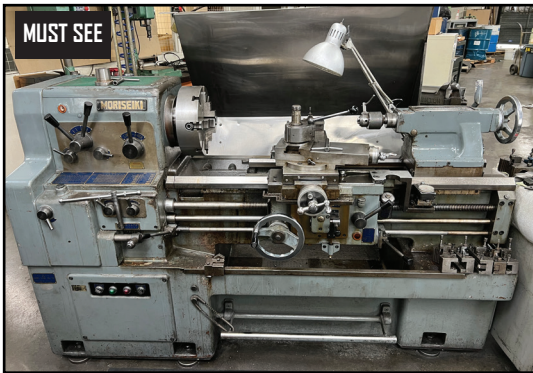
MORI SEIKI MS 850G, GAP FRAME ENGINE LATHE, 4 JAW CHUCK, STEADY REST, TOOLED.
