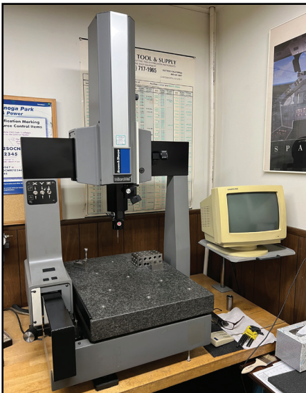
BROWN & SHARP MICRO VAL CMM W/ RENISHAW TP1S PROBE AND COMPUTER.
