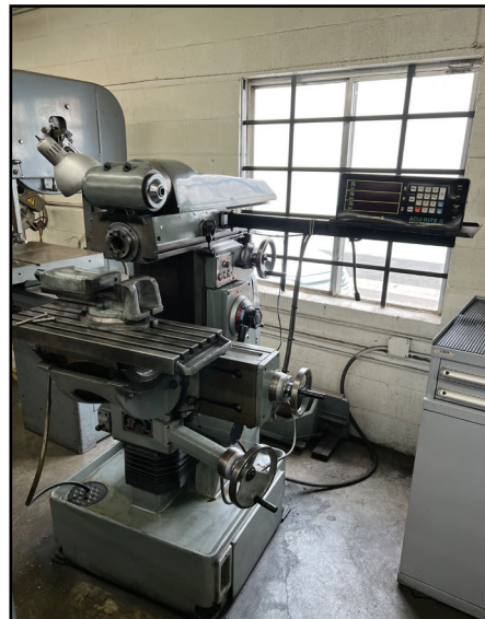
SELECT ZUTM UNIVERSAL TOOL ROOM MILLING MACHINE W/ VERTICAL & HORIZONTAL HEADS, DRO, S/N 1562.
