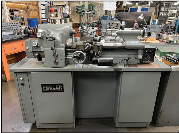
FEELER MODEL FTL-618E TOOL ROOM LATHE, W/ IN AND METRIC THREADING, S/N TL84172.
