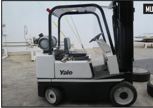
Yale 5000 Lb Cap LPG Forklift w/ 3-Stage Mast, Side Shift, Solid Tires
