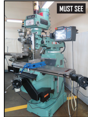
MUST SEE Proto-Trak TRAK-K3 KMX 2-Axis CNC Vertical Mill w/ Proto-Trak KMX Controls, 3Hp, Dial RPM, Power Draw-Bar, Chrome Box Ways, 10" x 50" Table
