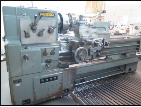
Mori Seiki MH1500G 24" x 62" Gear-Gap Lathe w/ 27-1205 RPM, 3" Thru Spindle, Inch Threading, Tailstock, Steady Rest, Trava-Dial, 14" Chuck
