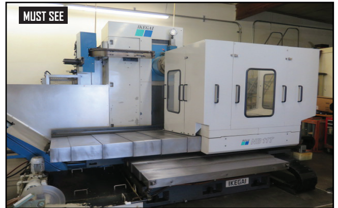
Ikegai NB 11T CNC HMC w/ Fanuc 16i-M Controls, 30-Station ATC, BT-50, 5" Spindle, 37 1/2" x 41 1/2" Table
