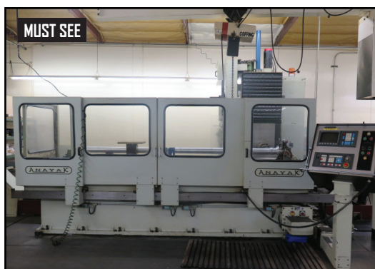
1997 Anayak "Anak-Matic-9-CNC" CNC VMC w/ Fanuc 0-m Controls, 20-Station ATC, BT-50, 21" x 51" Table
