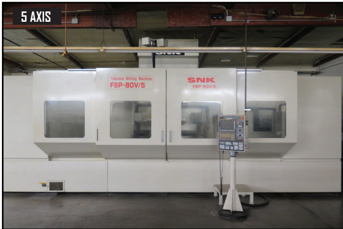
SNK FSP-80 V-5 5-Axis "Titanium Milling Machine w/ Fanuc 31i-MODEL A5 Controls, 40-Station ATC, BT-50, 4000 RPM, Travels X=90.5", Y=33.4", Z=27.5", A & B=+/- 30 Deg, 31 1/2" x 78 3/4" Table
