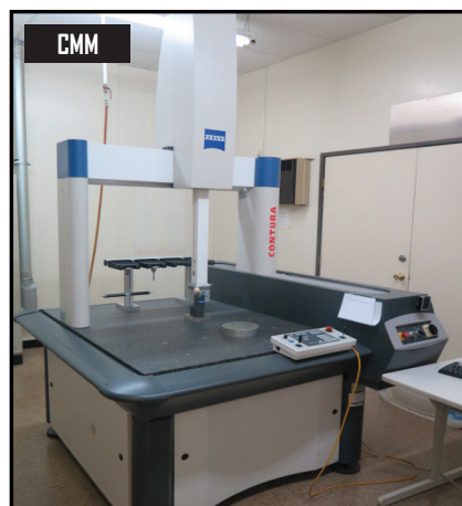
Zeiss "Contura 7/10/6" CMM Machine w/ VAST Probe Head, 4-Station Tip Changer, Zeiss Joystick Controller, Calypso 2019 Software
