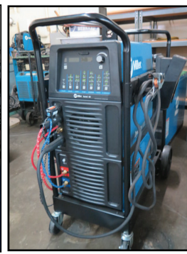
Miller Dynasty 400 Arc Welding Power Source w/ Wireless Foot Control
