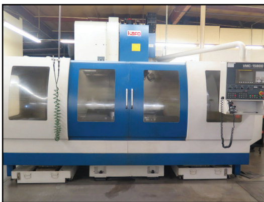
2006 Kafo VMC-15800 CNC VMC w/ Fanuc 0i-MC Controls, 30-Station ATC, BT-50, Coolant Filtration, 30" x 75" Table
