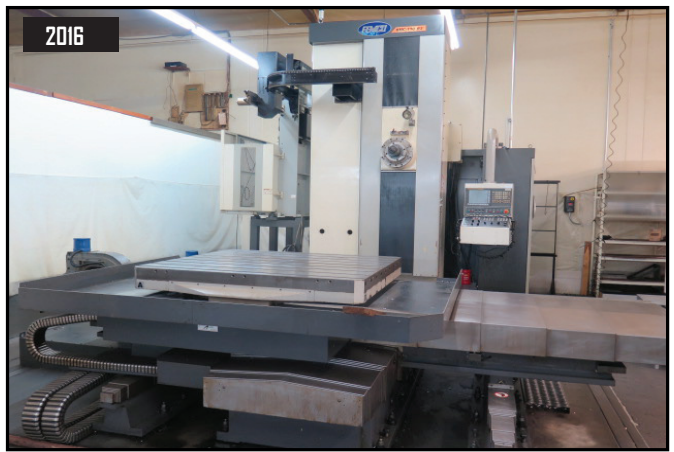
2016 Femco BMC-110 R2 CNC Horizontal Boring Mill w/ Fanuc 32i-MODEL B Controls, 60-Station ATC, BT-50, 6" Spindle, 56 3/4" x 63" Table
