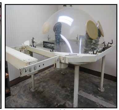
Jetline WC-48 Welding Chamber w/ Flip-Top
