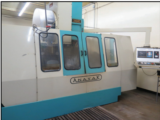
1997 Anayak "Anak-Matic-9-CNC" CNC VMC w/ Fanuc 0-m Controls, 20-Station ATC, BT-50, 21" x 51" Table
