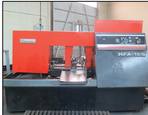
Amada HFA-16S 16" Automatic Horizontal Band Saw w/ Micro Processor Control
