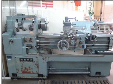
Mori Seiki MS-850G 17" x 36" Gear-Gap Lathe w/ 32-1800 RPM, 2 1/8" Thru Spindle, Inch Threading, Tailstock, Steady Rest, Trava-Dial, 10" Chuck
