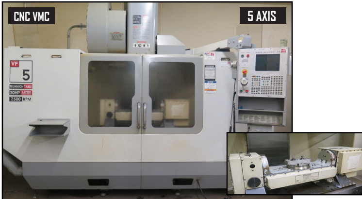
2005 Haas VF5/50TR 5-Axis Trunnion CNC VMC w/ Haas Controls, 30-Station ATC, BT-50, 8" 5 th Axis Trunnion Table, 30Hp, 2-Speed Gear Drive, 7500 RPM 8" 5 th Axis Trunnion Table
