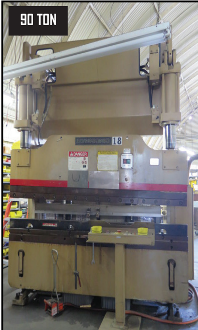
90 TON Cincinnati 90CBIIx6 90 Ton x 8' CNC Hydraulic Press Brake w/ Cincinnati Controls, 8' Bed, 12" Throat
