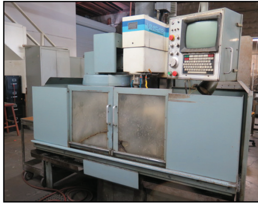
Fadal VMC40 4-Axis CNC VMC w/ CNC88 Controls, 21-ATC, CAT-40, 7500 RPM
