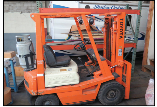
Toyota 42-5FGC25 4000 Lb Cap LPG Forklift w/ 3-Stage Mast, Solid Tires
