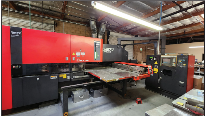
1994 AMADA MODEL APELIO II 357 CNC LASER AND PUNCH COMBINATION, W/ AMADA 04PC CONTROL, 58 STATION TURRET, 33 TON CAPACITY, 1.5 KW LASER.
