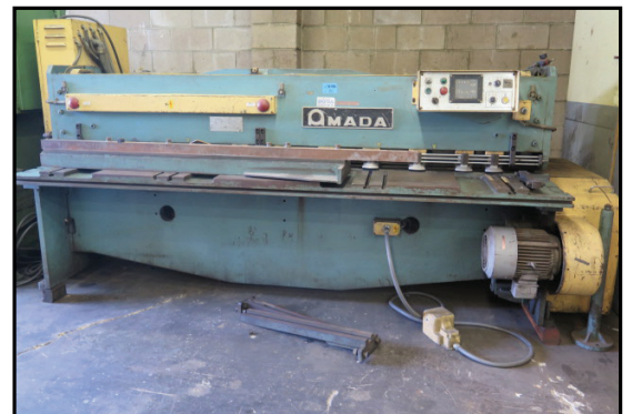
Amada M-2045 3/16" x 78" Power Shear w/ Amada Controls and Back Gauging, 86" Squaring Arm,
