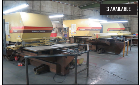
3 AVAILABLE Strippit "Fabri-Center" FC-1000 III 33-Ton 33-Station CNC Turret Punch Presses w/ Fanuc GN6 and HECC-80/3 Controls ***3-AVAILABLE***
