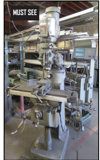
Bridgeport Series 1 – 2Hp Vertical Mill w/ Mitutoyo DRO, 62-4200 RPM, Chrome Ways, Power Feed
