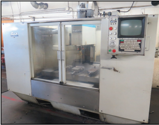
Fadal VMC4020 CNC VMC w/ CNC88HS Controls, 21-ATC, CAT-40, 7500 RPM, Rigid Tapping, High Speed CPU, Graphics, Tool Load Comp, Software Assist
