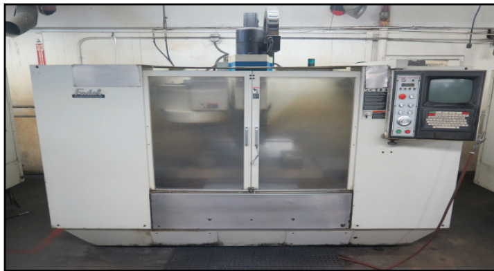
Fadal VMC4020 CNC VMC w/ CNC88 Controls, 21-ATC, CAT-40, 7500 RPM
