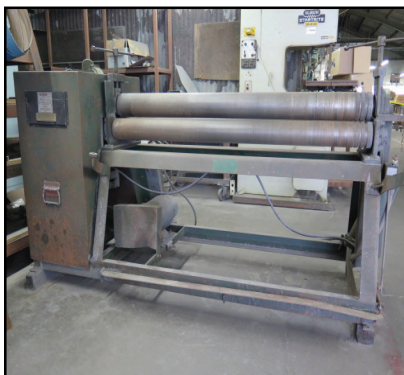
New Dimension mdl. 5-125 60" Power Roll w/ 4 1/2" Rolls
