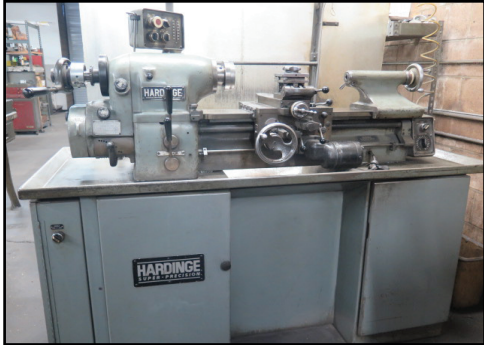
Hardinge HLV-H Wide Bed Tool Room Lathe w/ 130-3000 RPM, Inch Threading, Tailstock, Power Feeds, Compound Cross Slide, 5C, 6" 3-Jaw Chuck
