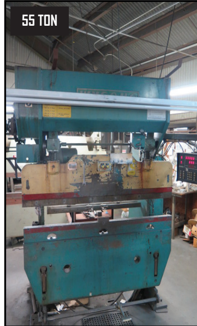
55 TON Wysong mdl. 55-4 55 Ton x 6' CNC Press Brake w/ Dynabend 1 Controls, 3" Stroke, 3" Ram Adj., 12" Die Space
