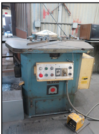
Amada CS-220 8 5/8" x 8 5/8" 10 Ton Hydraulic Power Corner Notcher
