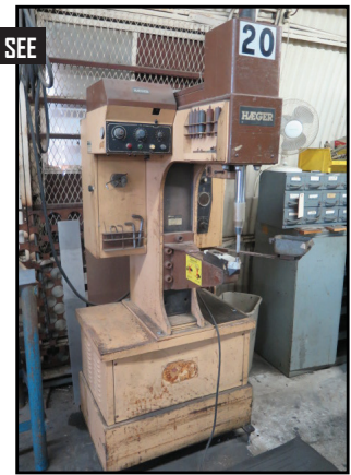
MUST SEE Haeger BP6-10 6-Ton Hardware Insertion Press w/ Haeger Automatic Feeder
