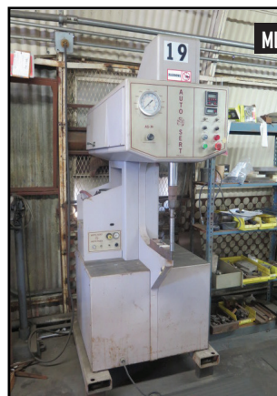
MUST SEE Auto-Sert A.S-7.5 7.5 Ton Hardware Insertion Press w/ 20" Throat, Auto-Sert Automatic Feeder
