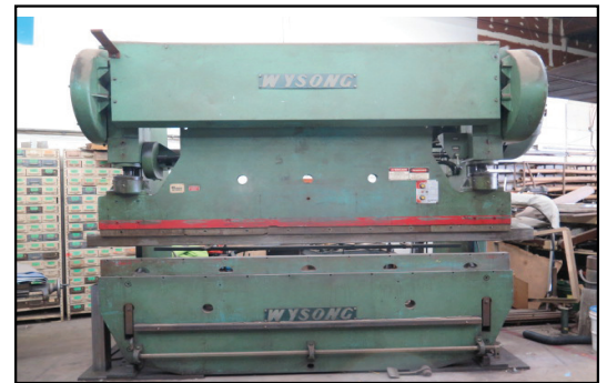
Wysong 150-8 150 Ton x 10' Mechanical Press Brake w/ 120" Bed, 8 5/8" Throat, 3" Stroke, 12" Die Space
