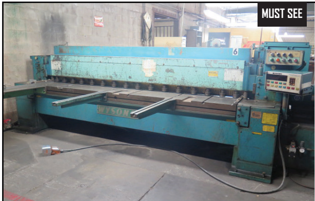
Wysong 1025 1/4" x 122" Power Shear w/ Wysong Controls and Back Gauging, 128" Squaring Arm, Front Supports
