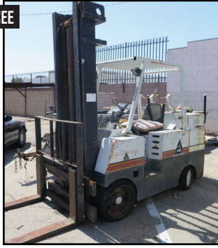
Allis Chalmers ACC70L 6100 Lb Cap LPG Forklift w/ 2-Stage Mast, 168" Lift Height, Solid Tires
