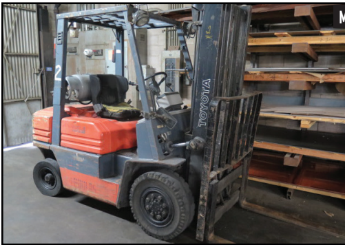
Toyota 5000 Lb Cap LPG Forklift w/ 3-Stage Mast, Side Shift, Solid Yard Tires
