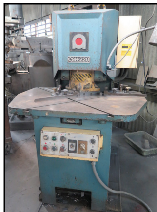
Amada CSH-220 1/4" 9" x 9" Hydraulic Power Corner Notcher
