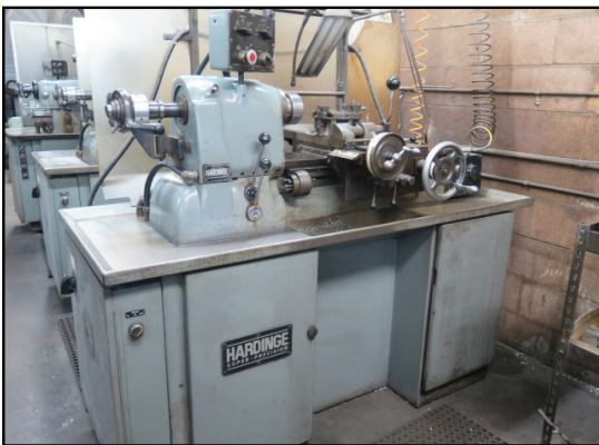
Hardinge HC Hand Chucker w/ 125-3000 RPM, 8-Station Turret, Power Feeds, 6" 3-Jaw Chuck
