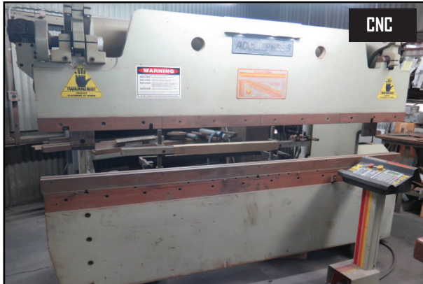
1997 Accurpress 7608 100 Ton x 8' Hydraulic Press Brake w/ Accurpress ETS Controls, Manual Back Gauging, 8 1/2" Throat
