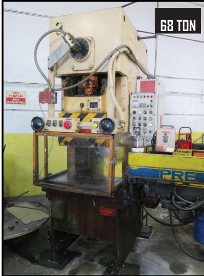
Aida NC1-6(1) 68 Ton Gap Frame Press w/ Aida Controls, 60-120 Strokes/Min, 3.54" Stroke, 10.63" Die Height, 2.76" Slide Adj., 18.89" x 15.74" Ram, 34.25" x 15.74" Bolster
