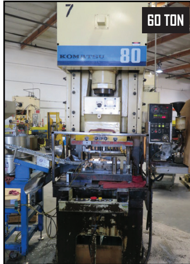
Komatsu OBS 80-3 80 Ton Gap Frame Press w/ Komatsu Controls, 37-75 Strokes/Min, 5.12" Stroke, 13.78" Die Height, 3.15" Slide Adj., 21.65" x 17.73" Ram, 39.37" x 23.62" Bolster
