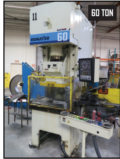
2000 Komatsu OBS 60-33 60 Ton Gap Frame Press w/ Komatsu Digital Controls, 75-150 Strokes/Min, 11.81" Die Height, 2.76" Slide Adj., 19.7" x 15.7" Ram, 35.4" x 21.7" Bolster
