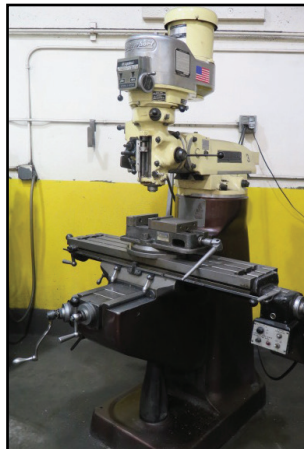
Bridgeport Vertical Mill w/ 2Hp, 60-4200 Dial RPM, Chrome Ways, Power Feed
