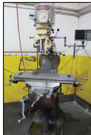
Bridgeport Vertical Mill w/ Anilam Wizard 211 DRO, 1.5Hp, 60-4200 Dial RPM, Chrome Ways, 9" x 32"
