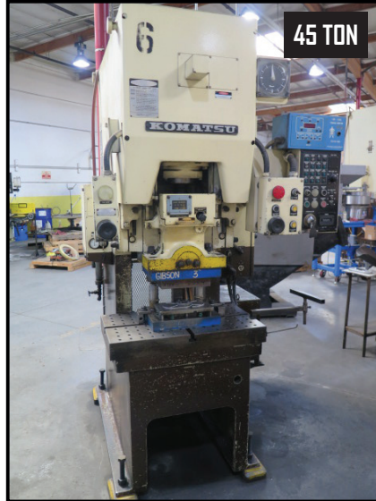
Komatsu OBS 45-2 45 Ton Gap Frame Press w/ Komatsu Controls, Link System 1000 Tollage Meter, 50-100 Strokes/Min, 3.94" Stroke, 9.43" Die Height, 2.36" Slide Adj., 15.75" x 11.81" Ram, 31.5" x 17.72" Bolster
