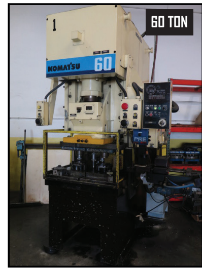
1992 Komatsu OBS 60-3 60 Ton Gap Frame Press w/ 75-150 Strokes/Min, 3.54" Stroke, 11.81" Die Height, 2.76" Slide Adj., 19.69" x 15.75" Ram, 35.43" x 21.65" Bolster
