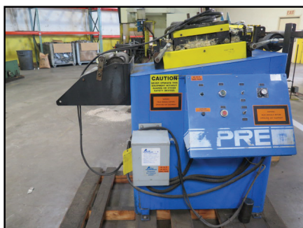
Press Room Equipment PR-HD-10-DG2-GC-480 10" Straightener / Feeder
