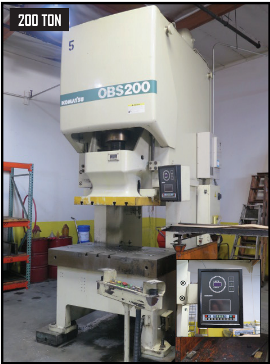
Komatsu OBS 200-5 200 Ton Gap Frame Press w/ Komatsu Digital Controls, 25-50 Strokes/Min, 6.3" Stroke, 18.9" Die Height, 4.72" Slide Adj., 33 1/2" x 25 3/4" Ram, 57" x 33" Bolster
