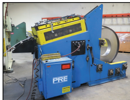
Press Room Equipment 18" Coil Cradle Straightener
