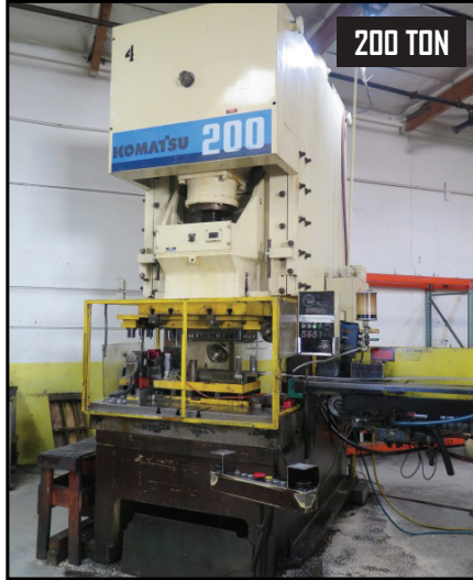
1991 Komatsu OBS 200-3 200 Ton Gap Frame Press w/ Komatsu Controls, 25-50 Strokes/Min, 9.84" Stroke, 18.9" Die Height, 4.72" Slide Adj., 33 1/2" x 25 1/2" Ram, 57" x 35" Bolster
