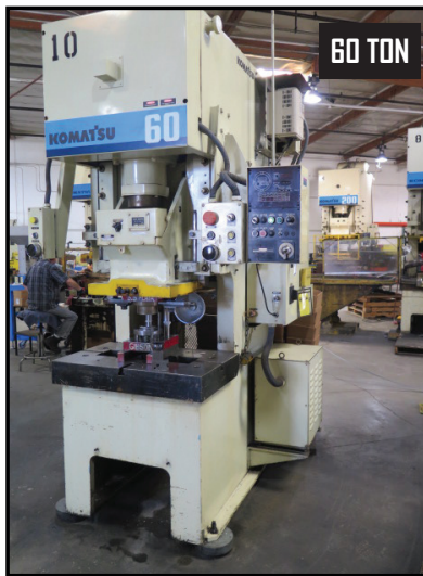
1995 Komatsu OBS 60H-VS-# 60 Ton Gap Frame Press w/ Komatsu Controls, 75-150 Strokes/Min, 3.54" Stroke, 11.81" Die Height, 2.76" Slide Adj., 19.69" x 15.75" Ram, 35.43" x 21.65" Bolster
