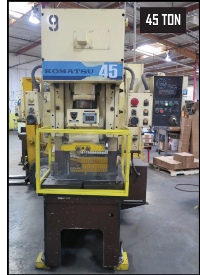
Komatsu OBS 45-3 45 Ton Gap Frame Press w/ Komatsu Controls, 100-200 Strokes/Min, 1.97" Stroke, 9.84" Die Height, 2.36" Slide Adj., 15.78" x 13.78" Ram, 31.5" x 17.72" Bolster
