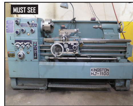
Kingston HJ-1100 17" x 46" Gear-Gap Lathe w/ 35-2000 RPM, Inch/mm Threading, Tail-stock, Steady Rest, 10" 3-Jaw and 12" 4-Jaw Chucks
