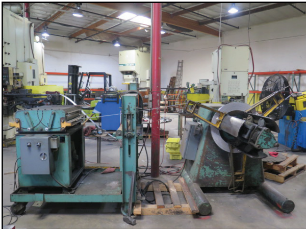
Rowe Straightener / Feeder w/ Uncoiler
