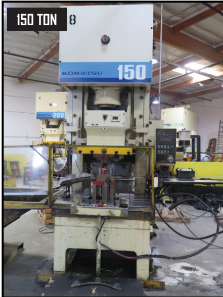
Komatsu OBS 150-3 150 Ton Gap Frame Press w/ Komatsu Controls, 27-55 Strokes/Min, 7.89" Stroke, 17.72" Die Height, 4.94" Slide Adj., 27.56" x 21.65" Ram, 49.21" x 31.5" Bolster
