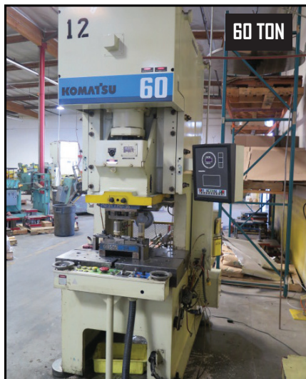
1998 Komatsu OBS 60L-VS-3 60 Ton Gap Frame Press w/ Komatsu Digital Controls, 42-85 Strokes/Min, 4.72" Stroke, 11.22" Die Height, 2.76" Slide Adj., 19.69" x 15.75" Ram, 35.43" x 21.65" Bolster
