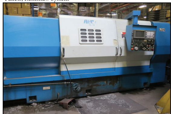
Femco HL-55S CNC Turning Center w/ Fanuc 18-T Controls, 12-Station Turret, Hydraulic Tailstock, 2500 RPM,
