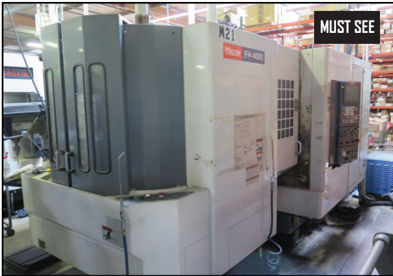
2001 Mazak FH 4000 2-Pallet CNC HMC w/ Mazatrol 640M PC-Fusion-CNC Controls, Tool Presetter, 40-Station ATC, CAT-40, 12,000 RPM, 4 th Axis @ 1 Degree, (2) 15 3/4" x 15 3/4" Pallets, Renishaw System
