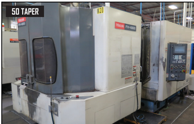
2001 Mazak FH 4800 2-Pallet CNC HMC w/ Mazatrol 640M PC-Fusion-CNC Controls, Tool Presetter, 80-Station ATC, CAT-40, 12,000 RPM, 4th Axis @ 1 Degree, (2) 15 3/4" x 15 3/4" Pallets, Renishaw System
