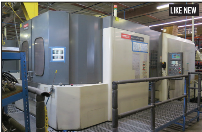
Mazak FH-6800 2-Pallet CNC HMC w/ Mazatrol 640M PC-Fusion-CNC Controls, Tool Presetter, 80-Station ATC, CAT-50, 4th Axis @ 1 Degree, (2) 24 3/4" x 24 3/4" Pallets, Oil Cooler, Mazak Coolant Filtration System
