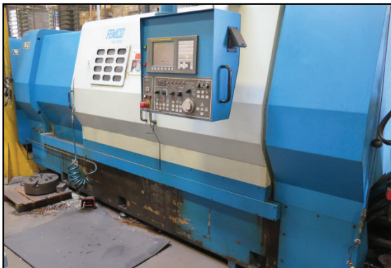
Femco HL-55S CNC Turning Center w/ Fanuc 0i-Tc Controls, 12-Station Turret, Hydraulic Tailstock, 2500 RPM, 15" 3-Jaw Chuck
