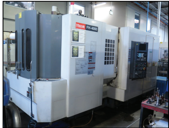
2002 Mazak FH 4000 2-Pallet CNC HMC w/ Mazatrol 640M PC-Fusion-CNC Controls, Tool Presetter, 40-Station ATC, CAT-40, 12,000 RPM, 4 th Axis @ 1 Degree, (2) 15 3/4" x 15 3/4" Pallets, Renishaw System
