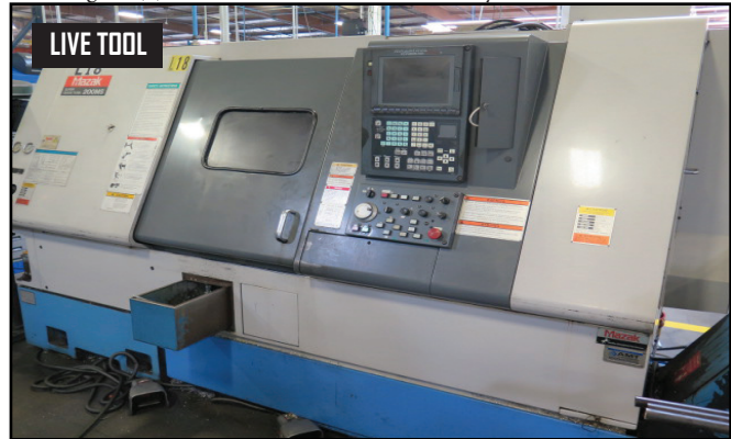
2002 Mazak Super Quick Turn 200MS Twin Spindle Live Turret CNC Turning Center w/ Mazatrol 640T PC-Fusion-CNC Controls, Tool Presetter, 12-Station Live Turret, (3) Rotary Tooling, 5000 RPM, 4500 Rotary Tool RPM
