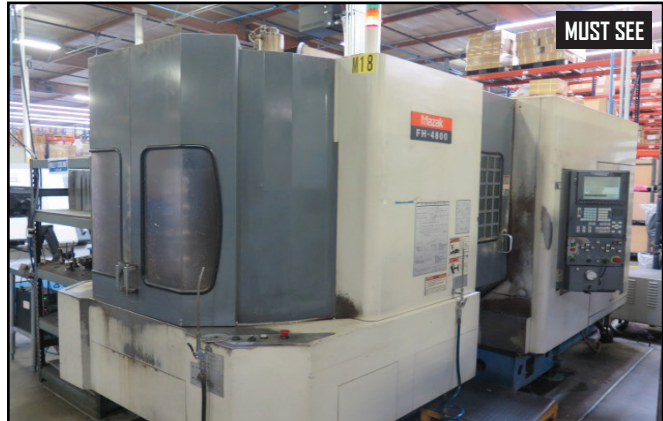
Mazak FH 4800 2-Pallet CNC HMC w/ Mazatrol 640M PC-Fusion-CNC Controls, Tool Presetter, 80-Station ATC, CAT-40, 12,000 RPM, 4th Axis @ 1 Degree, (2) 15 3/4" x 15 3/4" Pallets, Renishaw System
