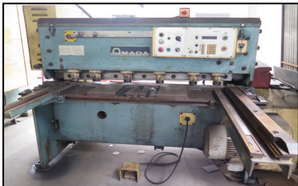
Amada M-1260 1/4" x 48" Power Shear w/ Amada Controls and Back Gauging
