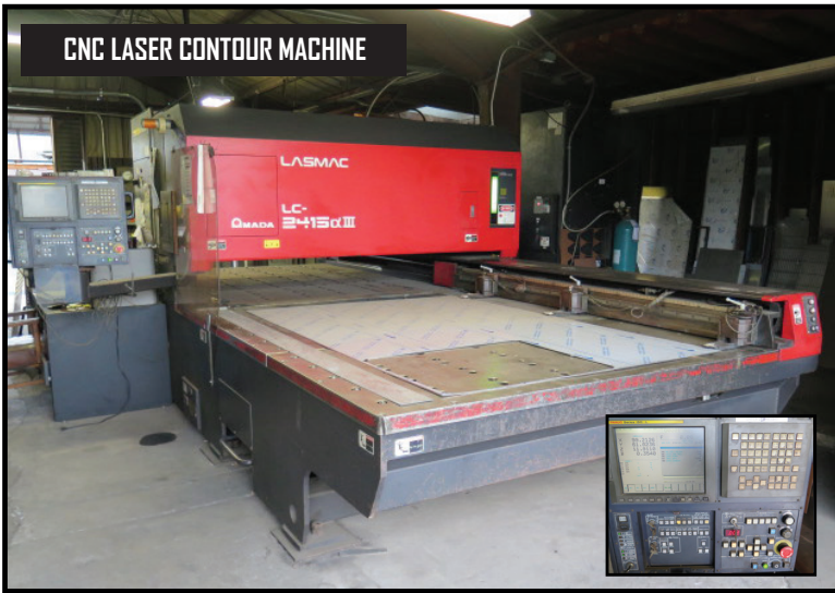
2001 Amada LASMAC LC-2415 cx III 3kW CNC Laser Contour Machine w/ Fanuc Series 160i-L Controls, Fanuc AF 3000D Laser Package
