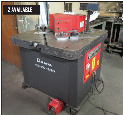
Amada CSHW-220 9" x 9" Hydraulic Corner Notcher w/ Amada Controls, 2-Axis DRO **2-AVAILABLE**
