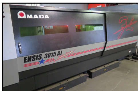
May/2019 Amada ENSIS 3015 AJ Fiber Laser 2-Pallet 5' x 10' CNC Laser Contour Machine w/ Amada AMNC 3i Controls, 3.15kW Laser Package
