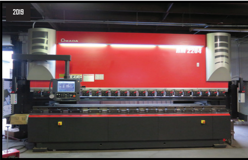
2019 Amada Model HM2204 169.3" x 243 Ton CNC Press Brake w/ Amada AMNC-PC 4 Axis CNC Controls.
