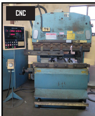
Amada RG-35S 35 Ton x 4' CNC Press Brake w/ Amada NC9-EX Controls
