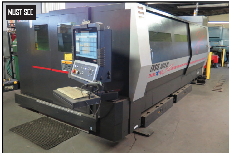
May/2019 Amada ENSIS 3015 AJ Fiber Laser 2-Pallet 5' x 10' CNC Laser Contour Machine w/ Amada AMNC 3i Controls, 3.15kW Laser Package
