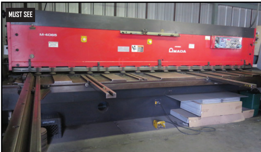
Amada M-4065 1/4" x 161" Mechanical Power Shear w/ Amada Digital CNC Controls and Back Gauging
