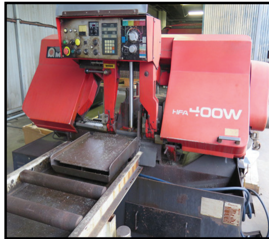
Amada HFA-400W 16" Automatic Hydraulic Horizontal Band Saw w/ Amada Controls
