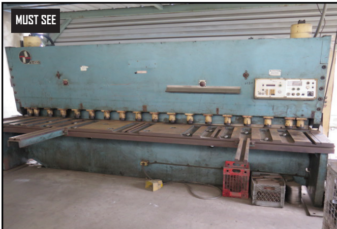
Amada H-4013 1/2" x 157.5" Power Shear w/ Amada Controls and Back Gauging
