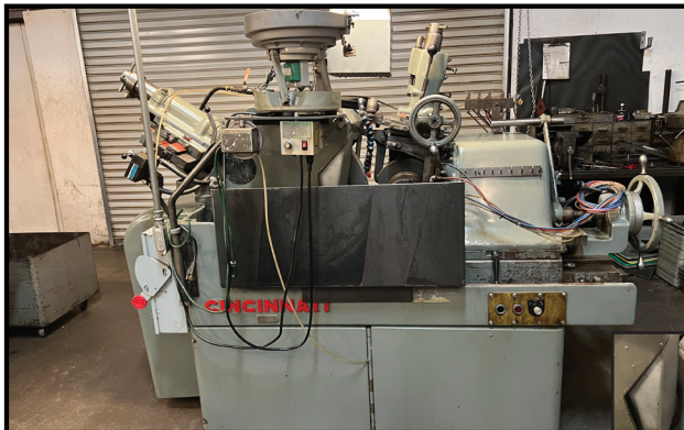
CINCINNATI MODEL OM CENTERLESS GRINDER, 24" WHEEL, S/N 2M2HIW-476.
