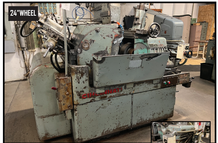
CINCINNATI MODEL OM CENTERLESS GRINDER, 24" WHEEL, W/ ALLEN AIR BELLOWS END FEED, S/N 2MWHIW-73.
