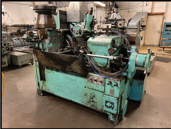
CINCINNATI MODEL CINCO 15 CENTERLESS GRINDER, 20" WHEEL, w/ AUTO BOWL FEED LOADER, S/N 35028HST-0113.
