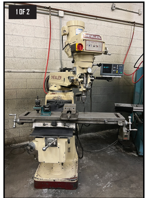
1 OF 2 CHEVALIER VERTICAL MILLING MACHINES, VAR SPEED, DRO, POWER FEED TABLE. CONTROLS, S/N 95-609.
