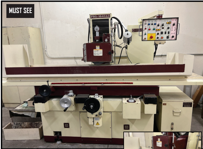
CHEVALIER FSG1640AD, 16" X 40" AUTOMATIC HYD SURFACE GRINDER, ELECTRO MAG CHUCK, EMS SPEED CONTROL.
