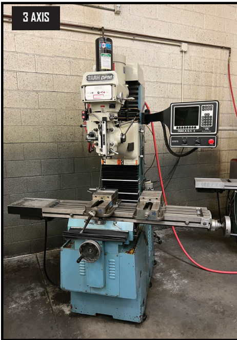
3 AXIS SOUTHWESTERN INDUSTRIES TRAK DPM 3 AXIS CNC BED MILL, 10" X 50" TABLE, 40 TAPER, 31" X 17" X 23.5" (XYZ), VARIABLE SPEED, 60-4200 RPM, PROTO TRAK A.G.E. 3 CONTROL, S/N 97-3095.
