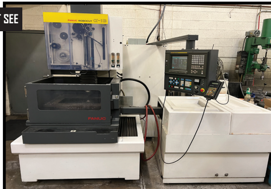
FANUC ROBOCUT ALPHA-1B CNC WIRE EDM, W/ FANUC 16-W CONTROLS, 17.73" X 11.82" X 11.82" (XYZ), MAX WORKPIECE SIZE: 29.5" X 25.5" X 12".
