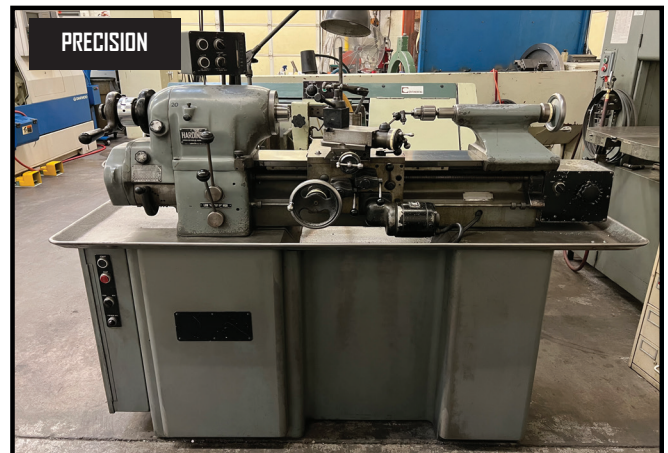
PRECISION HARDINGE HLH-H TOOL ROOM LATHE, W/ THREADING, S/N 4836.
