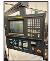
FANUC ROBOCUT ALPHA-1B CNC WIRE EDM, W/ FANUC 16-W CONTROLS, 17.73" X 11.82" X 11.82" (XYZ), MAX WORKPIECE SIZE: 29.5" X 25.5" X 12".
