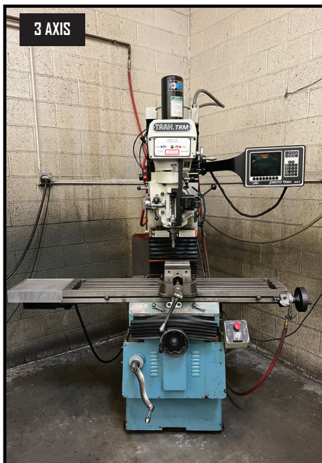
3 AXIS SOUTHWESTERN INDUSTRIES TRAK TRM 2 AXIS CNC BED MILL, 10" X 50" TABLE, 40 TAPER, 31" X 17" X 23.5" (XYZ), VARIABLE SPEED, 60-4200 RPM, PROTO TRAK MX2 CONTROLS, S/N 95-609.
