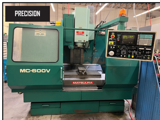
MATSUURA MC-600V CNC VMC, W/ 20 ATC, YASNAC CONTROLS, 40 TAPER.
