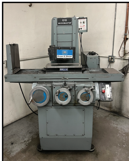
BROWN & SHARPE 618 MICROMASTER 6" X 18" SURFACE GRINDER, WALKER ELECTRO MAG CHUCK.
