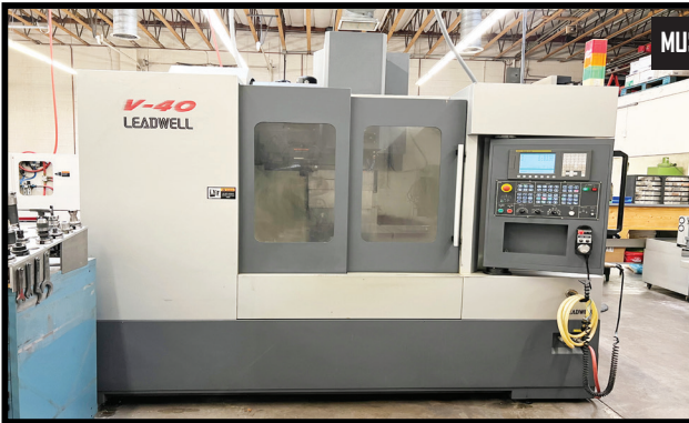
2011 LEADWELL MODEL V-40 CNC VMC, W/ FANUC Oi-MD CONTROL, 3 AXIS, 24 ATC, BT-40, 10,000 RPM, 40" X 20" X 24" (XYZ), S/N L2TAJ1132.
