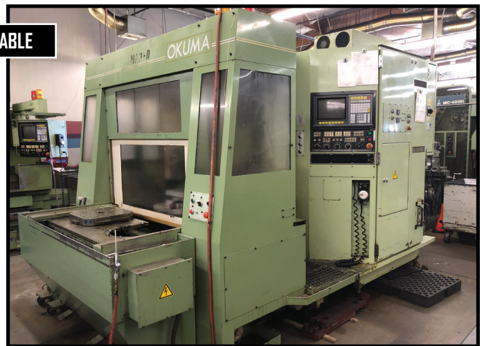
(2) OKUMA MODEL MC-40H CNC HMC'S, 3 PALLET SYSTEM, OKUMA SOP 5000M CONTROLS, 30 ATC.
