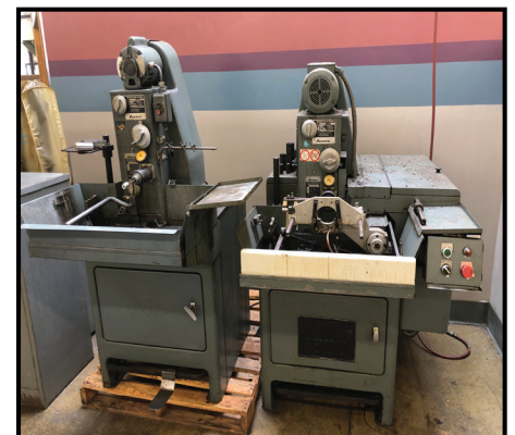
SUNNEN MODEL MBB 1660 & MBB 1801 HONING MACHINES, ONE WITH STROKER.
