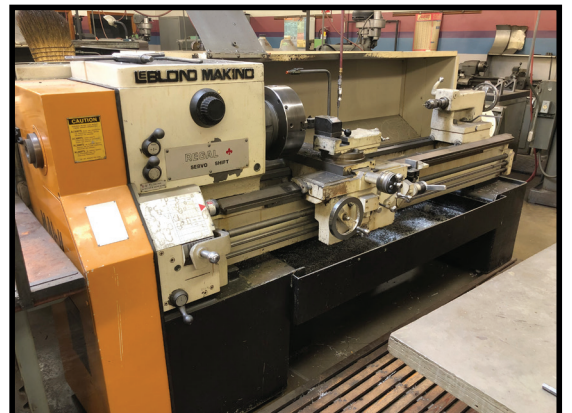
LE BLOND MAKINO 19" X 60" ENGINE LATHE, SERVO SHIFT, IN/MM THREADING.
