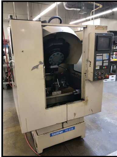
BROTHER MODEL TC-215 CNC DRILL AND TAPPING CENTER, 10 ATC. BROTHER MODEL TC-221 DRILL AND TAP CENTER, 10 ATC, BROTHER CONTROL.
