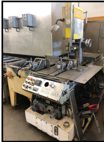
MARVEL MODEL V-10A VERTICAL IN FEED BAND SAW, PNEUMATIC CLAMPING, CONVEYOR. MARVEL MODEL V-10A VERTICAL
