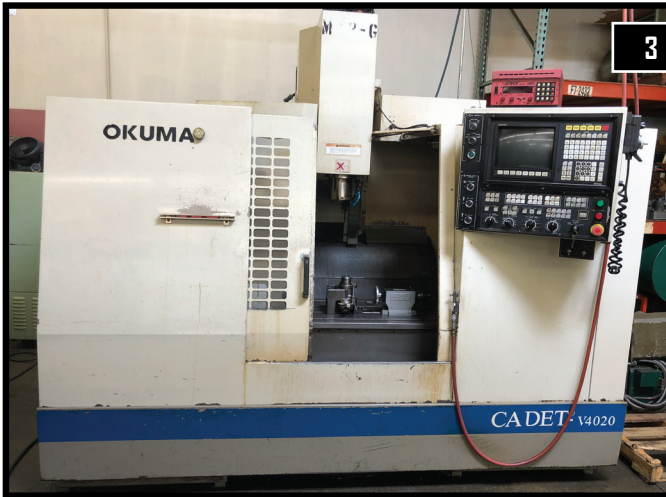
(3) OKUMA CADET-V4020 CNC VMC'S, 40" X 20" X 20" (XYZ), OKUMA 5020M CONTROL.
