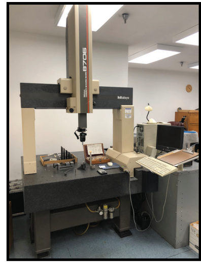
MITUTOYO MODEL B706 CMM, 36" X 50" TABLE, RENISHAW MIH PROBE.
