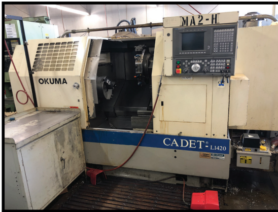
OKUMA CADET CNC LATHE, 12" CHUCK, TAIL STOCK, 3.5" SPINDLE BORE, OKUMA OSP-700L CONTROL, S/N 0267.
