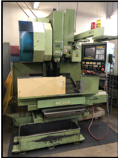
(2) OKUMA MODEL MC-4VAE VMC'S, 20 ATC, OKUMA 5020M CONTROL OKUMA MODEL MC-4VA VMC, 32 ATC, OSP 5000M-G CONTROL.
