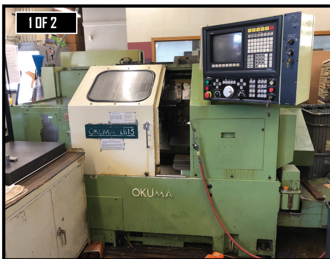
(1 OF 2) OKUMA LB15 CNC LATHES, W/ TAILSTOCK, OKUMA OSP 5020L & 5000L CONTROLS, 10 STATION TURRET.
