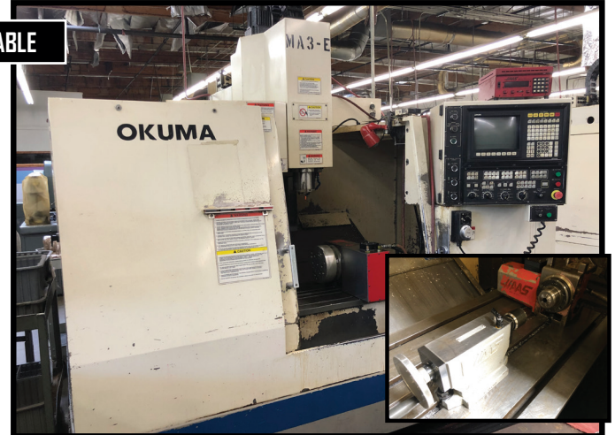
(3) OKUMA CADET-V4020 CNC VMC'S, 40" X 20" X 20" (XYZ), OKUMA 5020M CONTROL.
