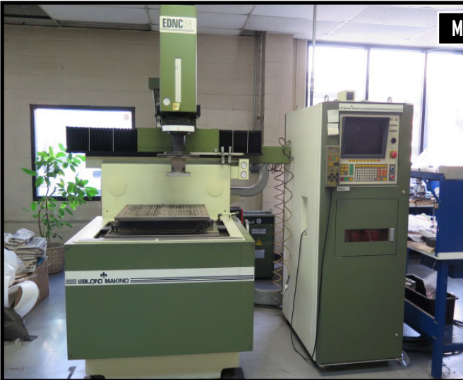
LEBLOND MAKINO MODEL EDNC64 CNC SINKER EDM, W/ MGC LS 42 CONTROLS, LS44 TEMP SENSOR
