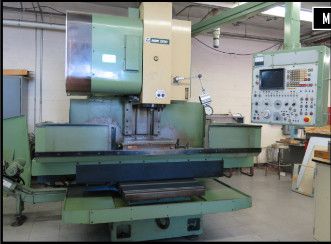
MORI SEIKI MV-45/40 CNC VMC, 40 TAPER, 31.5" X 17.7" X 19.7" (XYZ), FANUC CONTROL.
