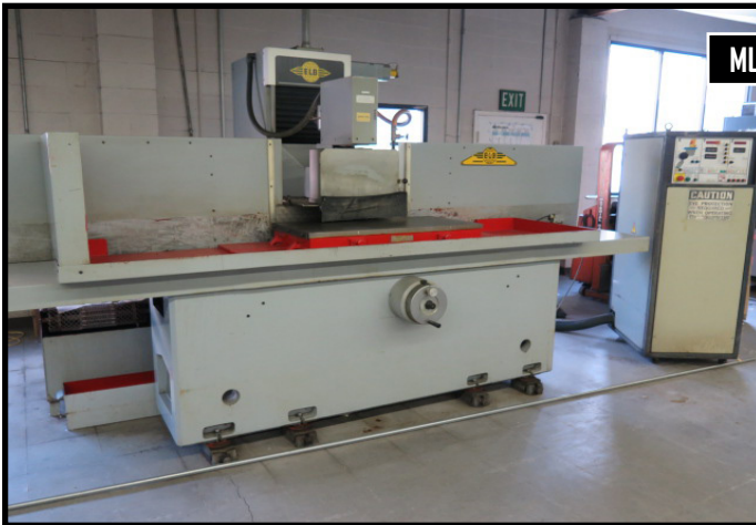
ELB SCHLIFF MODEL SWBE 0101NPC-K, HIGH PRECISION SURFACE GRINDER W/ CONTROLS.
