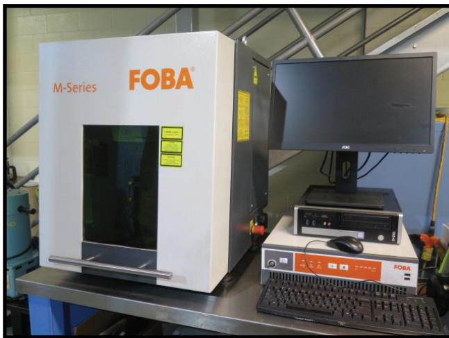
Foba M-Series Laser Marking System w/ Controls, Laser Cabinet, 9 1/2" x 19 1/2" Table, Computer, FOBA MarkUS 2.11.25.0 Software
