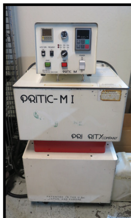
Pritic Magnetic Polishing Machine w/ Pritic-M Controls, Pritic-MI Magnetic Field Generation Tank
