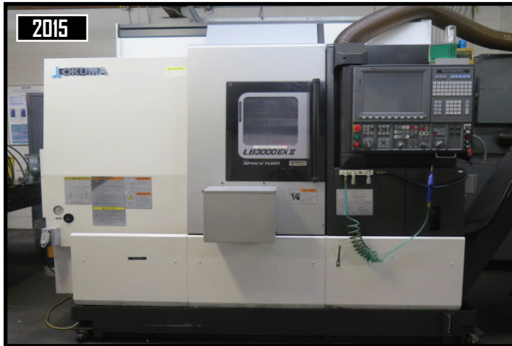
2015 Okuma "Space Turn" LB3000EX II CNC Live Turret Turning Center w/ Okuma OSP-P300L Controls, Presetter, 12-Station Live Turret, Tailstock, Full "C" Axis, "Y" Axis, Capto Tool Blocks, Hainbuch Collet Nose SK 65, Thermal Compensation, Navi-L-G Harmonics Spindle Speed Control, Synchronous Tapping, IGF Function
