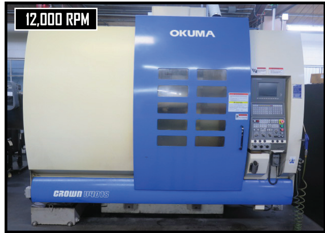
Okuma Crown V4018 CNC VMC w/ Okuma OSP-U10M Controls, 20-Station Side Mount ATC, CAT-40 Spindle, 12,000 RPM, Rigid Tapping, Thru Spindle Coolant
