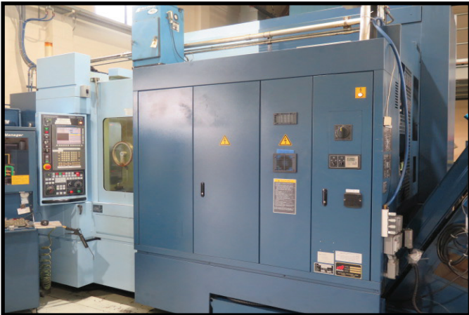
2) Matsuura H.Plus-300 in a 24 Linear Pallet System 4-Axis Horizontal Machining Center w/ Matsuura G-Teck 30i Controls, Renishaw NC4TX Laser Setting System, 240 / 320-Station ATC, CAT-40 Spindle, 15,000 and 20,000 RPM, CMM Probing Full 4 th Axis, High Pressure Coolant
