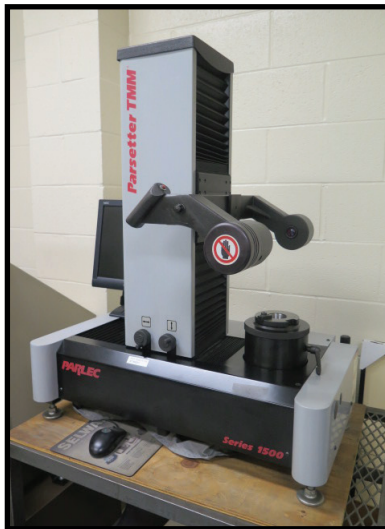
Parlec Series 1500 "Parsetter TMM" mdl. P1500 Tool Presetting System w/ 40 & 50 Taper Adapter
