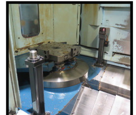
2) Matsuura H.Plus-300 in a 24 Linear Pallet System 4-Axis Horizontal Machining Center w/ Matsuura G-Teck 30i Controls, Renishaw NC4TX Laser Setting System, 240 / 320-Station ATC, CAT-40 Spindle, 15,000 and 20,000 RPM, CMM Probing Full 4 th Axis, High Pressure Coolant
