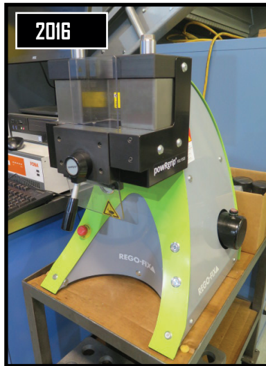
2016 Abnox / Rego-Fix mdl. powerGrip PGU9500 40 Taper Tool Holding System w/ CAT-40 Tooling
