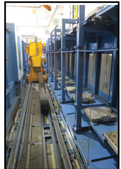
2002 Matsuura Maxia PC-17 Maxia Cell Management System, 2 Machines, 26 Pallet System, 24-Pallet Stacker, w/ Fanuc Power Mate16i and 30i CNC Controls, Maxia WS-26-26 Cell Management System, Pallet Car
