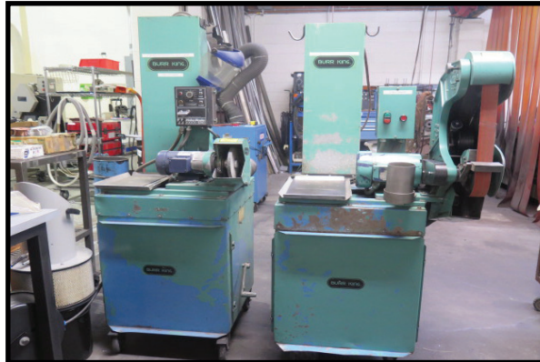
Burr King Deburring and Polishing Grinder and Burr King 2" Belt Sander w/ Burr King Dust Collectors
