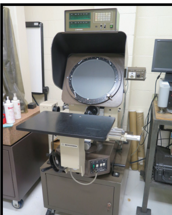
Mitutoyo PH-350 13" Optical Comparator w/ Mitutoyo DRO, Optoeye M1 Edge Zone Detector, Surface and Profile Illumination
