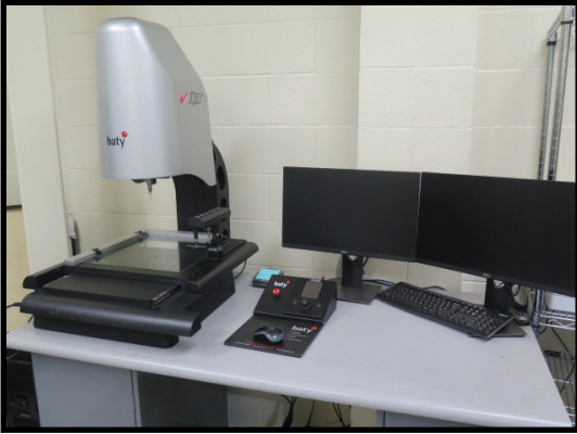
Fowler Baty Venture-3030XT Vision/CMM Machine w/ Video Feed Head, Renishaw MCR20 6-Station Probe Changer, Metrology Fusion MK4 3D Software
