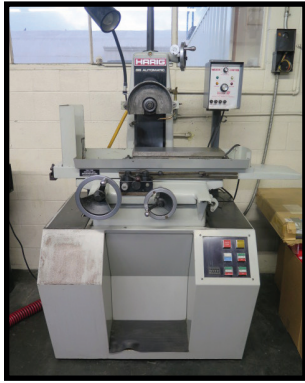
Harig "618 Automatic" 6' x 18' Automatic Hydraulic Surface Grinder
