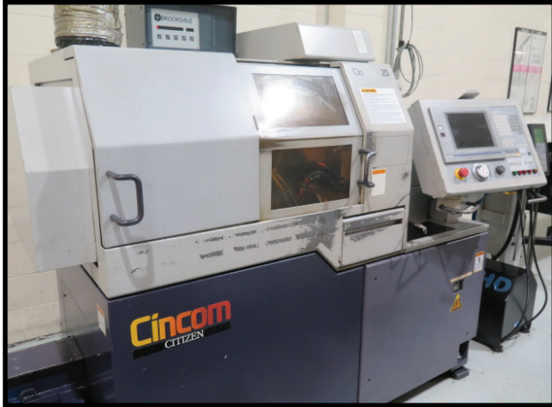
Citizen Cincom 20 Type L-20 Swiss Type CNC Screw Machine w/ Citizen Controls, (3) Drill/Bore Stations, (6) Turning Stations, (4) Overhead Tool Holders, 2000 PSI Cool Blaster HD High Pressure Coolant System
