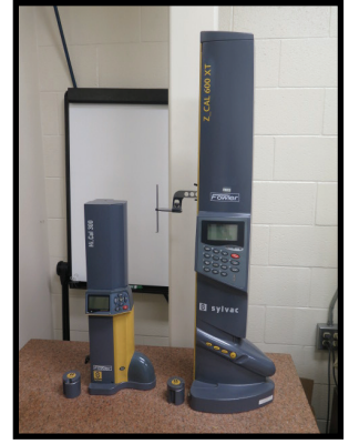
Fowler Sylvac Z_CAL 600XT 24" and Fowler Sylvac Hi_CAL 300 12" Digital Height Gages
