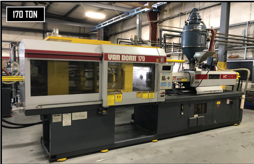
VAN DORN MODEL 170-RS-14F-HT, 170 & 14 OZ PLASTIC INJECTION MOLDER W/ CNC CONTROLS, S/N 397.
