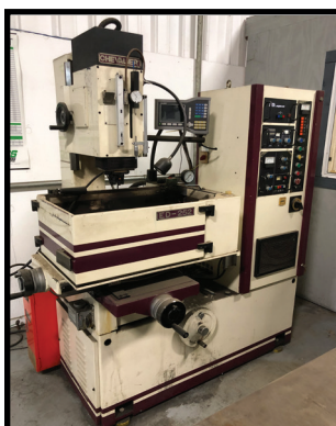
CHEVALIER RAM TYPE MODEL ED-252 SINKER EDM WITH DRO.
