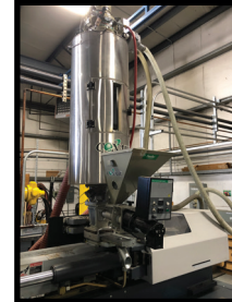
DEMAG ERGOTECH-CONCEPT 1100/470-430, 110 TON PLASTIC INJECTION MOLDER W/ DEMAG NC4 CNC CONTROLS, S/N 7173-0068.
