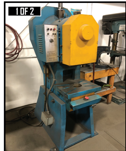
HEIM MODEL T15, 15 TON MECHANICAL PUNCH PRESSES W/ PALM BUTTON.
