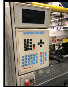
VAN DORN MODEL 170-RS-14F-HT, 170 & 14 OZ PLASTIC INJECTION MOLDER W/ CNC CONTROLS, S/N 397.
