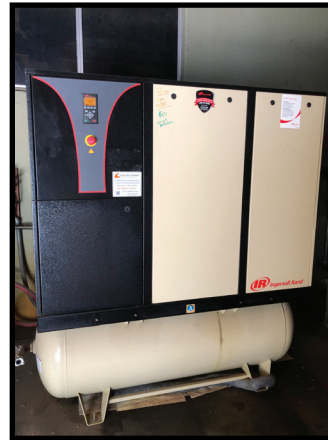
IR IRN20H-CC, 20 HP ROTARY AIR COMPRESSOR WITH TANK, 150 PSI RATED PRESSURE.
