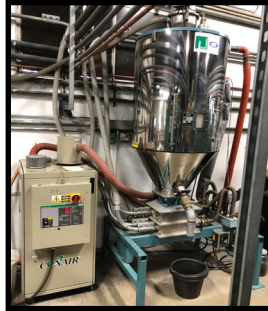
CONAIR COMPU DRY CD60 AND UNA DYN 400 SOLID CONE HOPPER.
