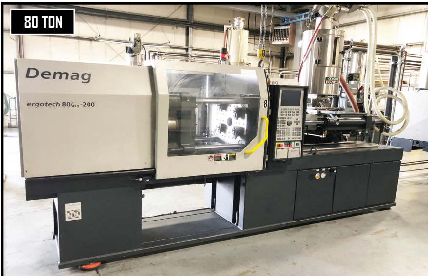
DEMAG ERGOTECH 800/420-200, 80 TON PLASTIC INJECTION MOLDER W/ DEMAG NC4 CNC CONTROLS, S/N 7153-0016.
