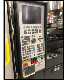
DEMAG ERGOTECH-CONCEPT 1100/470-430, 110 TON PLASTIC INJECTION MOLDER W/ DEMAG NC4 CNC CONTROLS, S/N 7173-0068.
