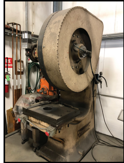
ROUSSELLE MODEL 4G, 40 TON DEEP THROAT PUNCH PRESS, AIR CLUTCH.
