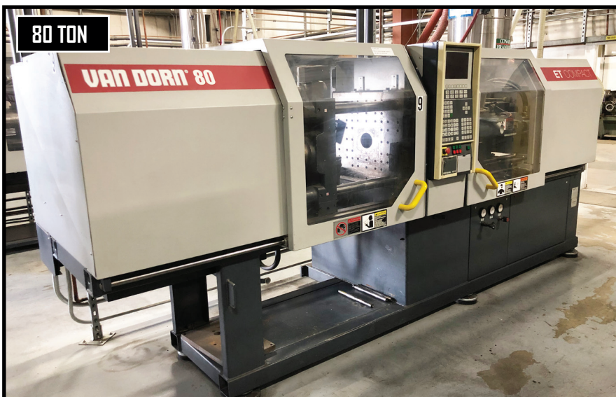
VAN DORN DEMAG ERGOTECH COMPACT 800-200, 80 TON PLASTIC INJECTION MOLDER W/DEMAG NC4 CNC CONTROLS, S/N 7151-0180.
