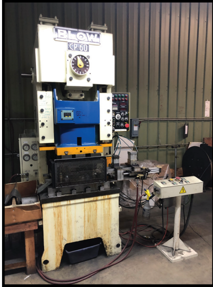
2001 BLOW CP - 60, 60 TON GAP FRAME PUNCH PRESS, W/ 3.94" STROKE, 60-90 SPM, 11.81" DIE HEIGHT, 33.08" X 19.69" BOLSTER AREA.
