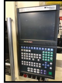
VAN DORN 400HP-RS—48FHS, 400 TON & 48 OZ PLASTIC INJECTION MOLDER, UPGRADED WITH SUMITOMO DEMAG NC5 CNC CONTROLS, S/N 397.
