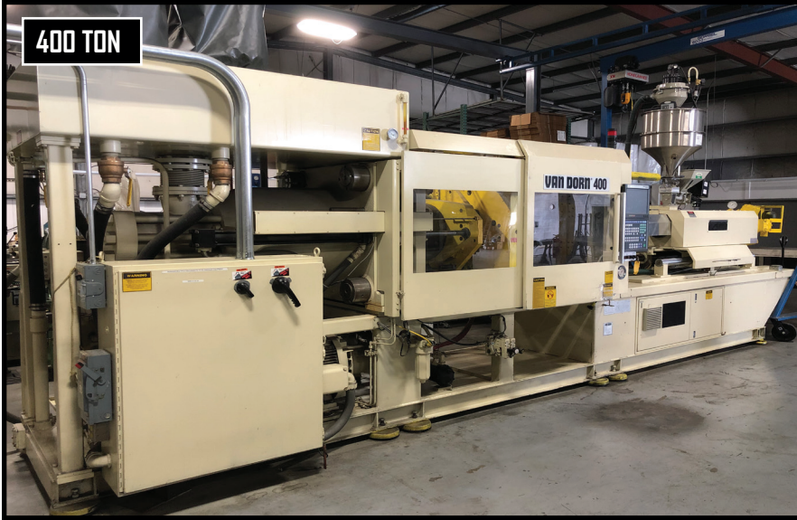
VAN DORN 400HP-RS—48FHS, 400 TON & 48 OZ PLASTIC INJECTION MOLDER, UPGRADED WITH SUMITOMO DEMAG NC5 CNC CONTROLS, S/N 397.
