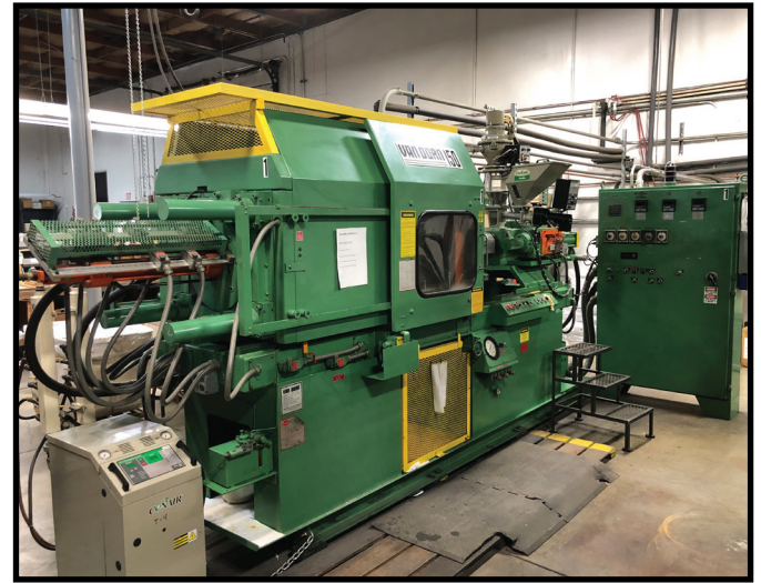
VAN DORN 150-RS-8F, 150 TON & 8 OZ PLASTIC INJECTION MOLDER.
