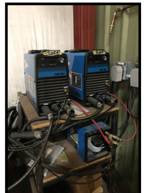
AUTOMATIC WELDING SYSTEM W/ MILLER MAXSTAR 200 WELDING POWER SUPPLIES.
