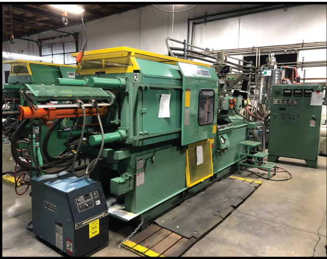
VAN DORN 200-RS-14F, 200 TON & 14 OZ PLASTIC INJECTION MOLDER
