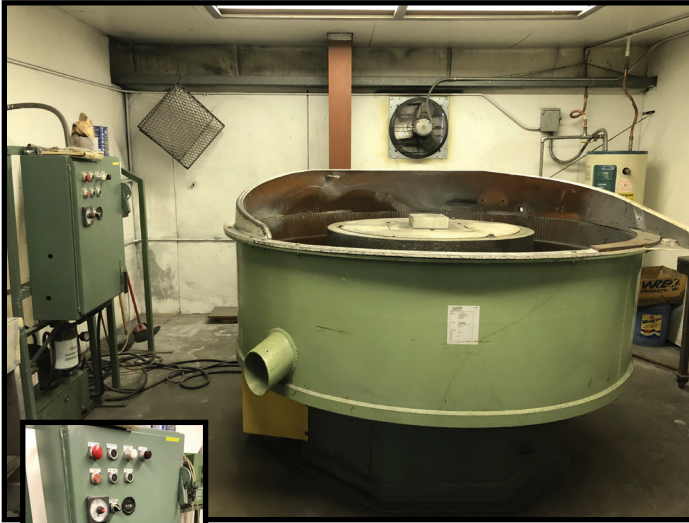
LARGE VIBRATORY BOWL TUMBLER WITH CONTROLS.
