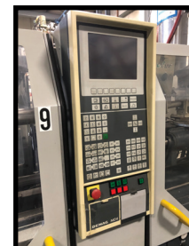
VAN DORN DEMAG ERGOTECH COMPACT 800-200, 80 TON PLASTIC INJECTION MOLDER W/DEMAG NC4 CNC CONTROLS, S/N 7151-0180.
