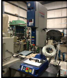
BRANSON MODEL 2000 iW PLUS ULTRASONIC WELDER.
