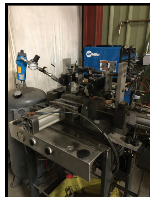
AUTOMATIC WELDING SYSTEM W/ MILLER MAXSTAR 200 WELDING POWER SUPPLIES.
