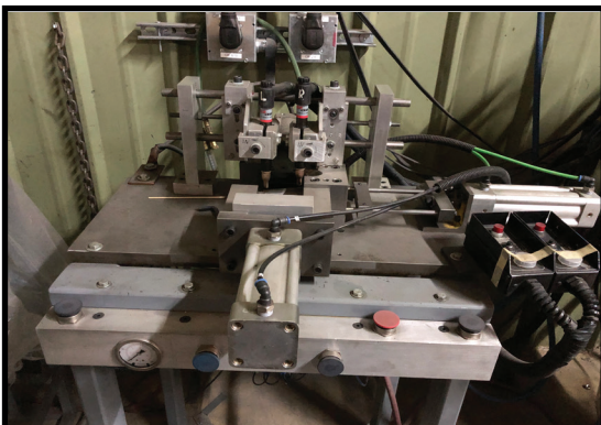
AUTOMATED WELDING SYSTEM W/ 2) MILLER INTELLITIG POWER SUPPLIES.
