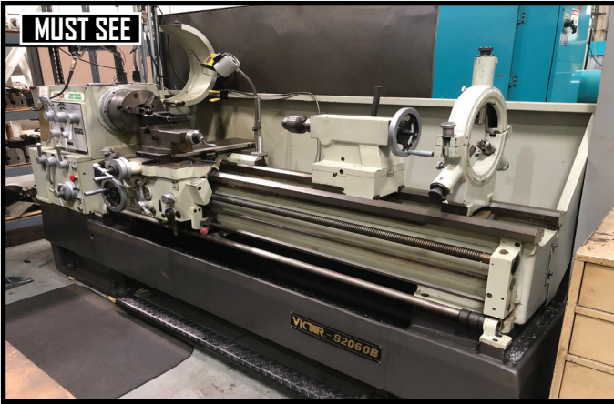
VICTOR MODEL S2060B, 20" X 60" ENGINE LATHE, W/ DRO, IN/METRIC THEADING.
