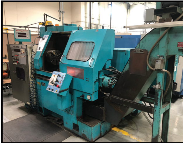
MAZAK DYNA TURN 3L CNC LATHE, WITH FANUC CONTROL, CHIP CONVEYOR, TAIL STOCK.
