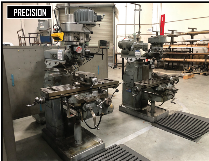
TREE MODEL 2UVR AND 2VG VERTICAL MILLING MACHINES.
