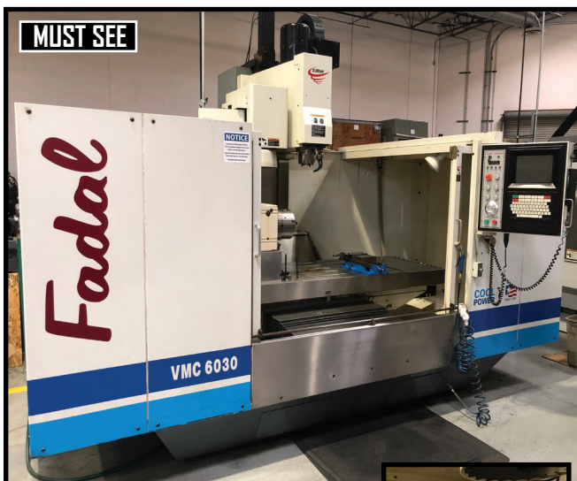
FADAL MODEL 6030 CNC VMC, 10,000 RPM, 4 TH AXIS READY, 60" X 30" X 30" (XYZ), S/N 9807431.
