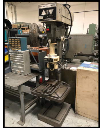
ROCKWELL VAR SPEED DRILL PRESS WITH PROCUIER TAPPING HEAD.
