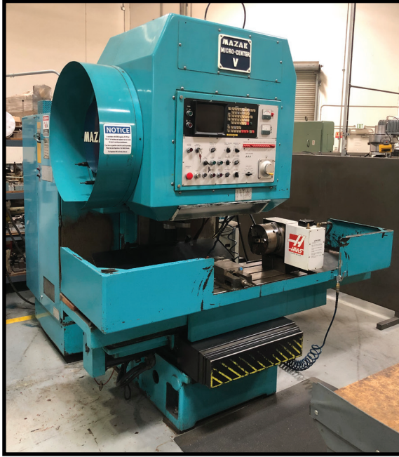
MAZAK MODEL MICRO CENTER V CNC VMC, FANUC 6M, 24 ATC, 30" X 15.7" X 17.7" (XYZ), 4TH AXIS READY, S/N 70338926..
