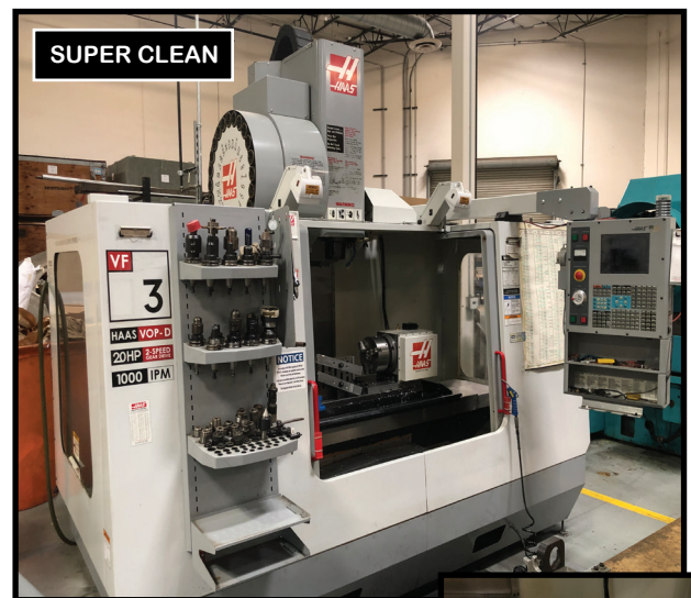
2004 HAAS MODEL VF-3B CNC VMC, 2 SPEED GEAR DRIVE, SIDE MOUNT TOOL CHANGER, 24 ATC, CAT 40 TOOL HOLDER, 4 TH AXIS READY, 40" X 20" X 20 (XYZ), S/N 36724.
