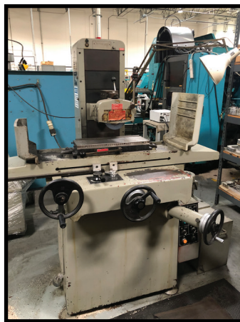
YAMAZEN MODEL KGS-250AH, 6 X 18 AUTOMATIC SURFACE GRINDER.
