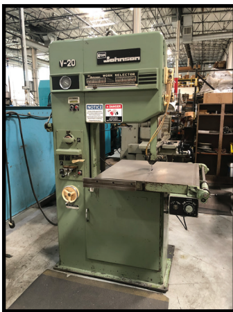
KYSOR JOHNSON MODEL V-20 BAND SAW, 20" THROAT CAPACITY, BLADE WELDER.
