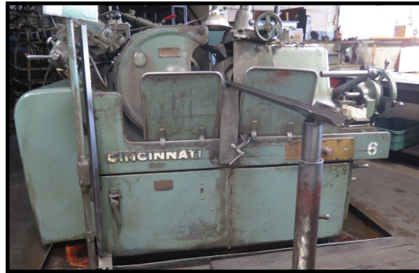
Cincinnati OM Centerless Grinding Machine w/ Hydraulic Grinding Wheel Dresser, Manual Feed Wheel Dresser, 21" Grinding Wheel, Belt Drive Conversion
