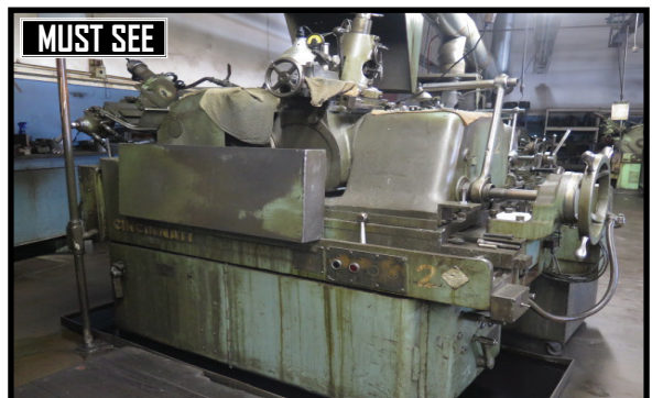
Cincinnati OM Centerless Grinding Machine w/ Hydraulic Grinding Wheel Dresser, Manual Feed Wheel Dresser, 21" Grinding Wheel, Belt Drive Conversion
