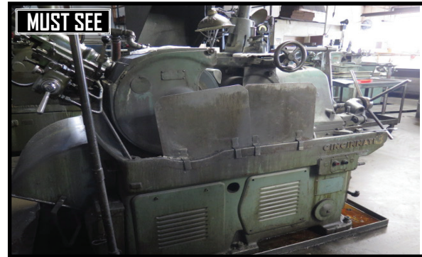
Cincinnati EA Centerless Grinding Machine w/ OM Conversion, Hydraulic Grinding Wheel Dresser, Manual Feed Wheel Dresser, 21" Grinding Wheel, Belt Drive Conversion
