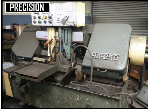
Amada HA-250 10" Automatic Hydraulic Horizontal Band Saw w/ Hydraulic Clamping and Feed
